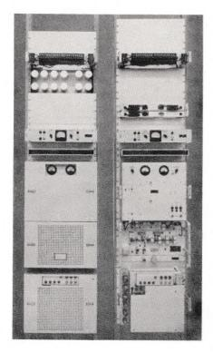
FIG. 2. Two Type 72 transmitter assemblies arranged to transmit over a common antenna.
