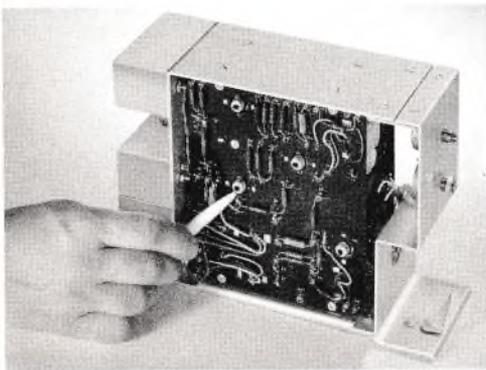
*FIG. 3. The carrier frequency supply unit for a Type 45CB carrier terminal. The pointer indicates one of the six transistors in this unit.*
