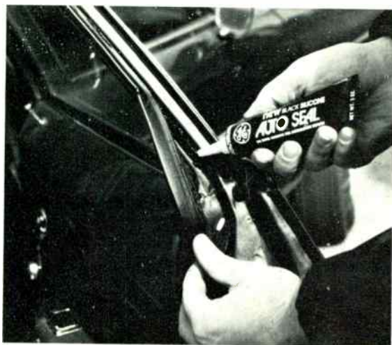
Resticking car door gaskets or forming new ones with GE Auto Seal will stop leaks. The silicone rubber stays flexible in below zero temperatures.
