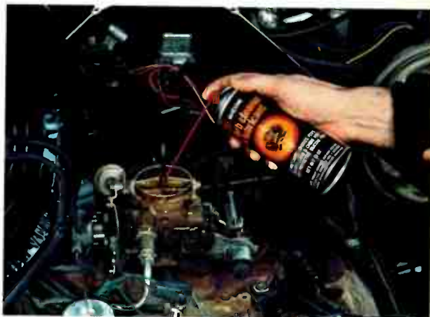
Silicone carb cleaner and lubricant provides inexpensive preventive maintenance against hard starts and rough running.
