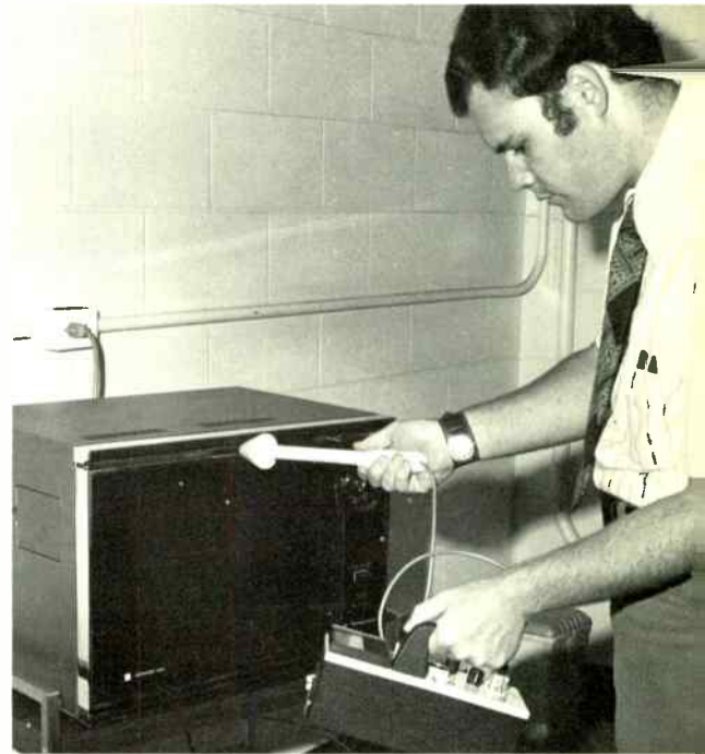
Tests of GE microwave ovens insure that radiation leakage is far below stringent safety requirements set by the Federal Government.
