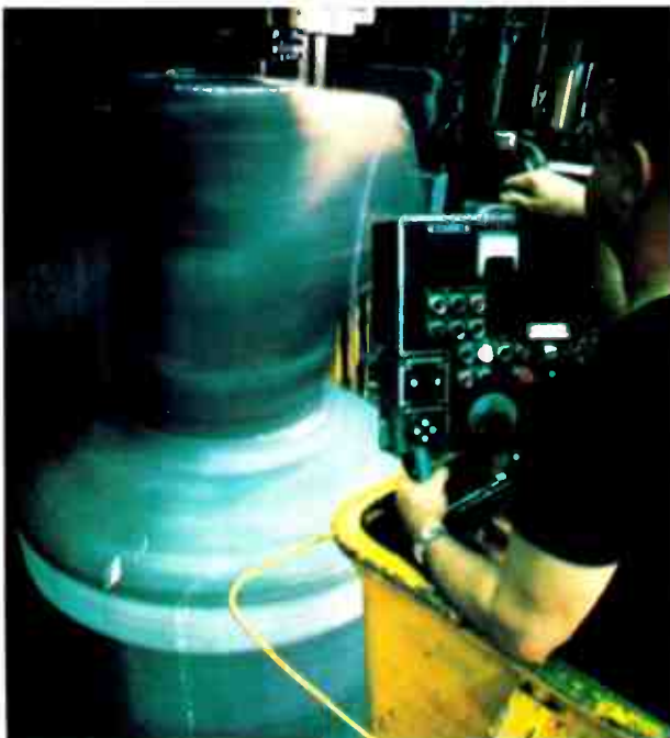
"A turbine shell, marked in numbered squares to guide grinding operations, reminded me of a huge turtle."
