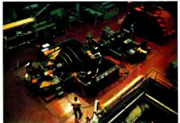
"They do things on a big scale in this business. The Product Development Lab even has this permanent turbine just to test turbine components."
