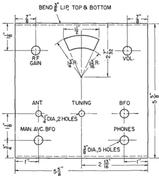
Fig. 7. Front panel layout of Mobile-Marine Receiver.
