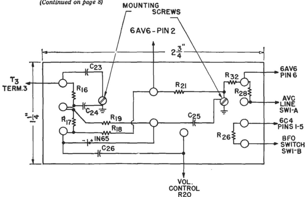
Fig. 9. Sub-assembly diagram.
