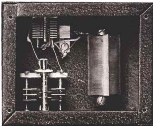
Fig. 6. Detail View of Oscillator Grid Circuit.
