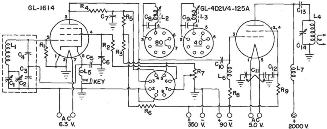
Fig. 4. Circuit Diagram of the Economy Half-Kilowatt.
