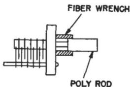
Fig. 8. Hex Shaft Variable With Regular Shaft Added.
