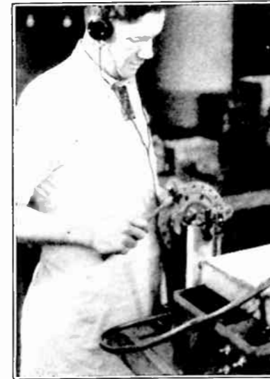
Centering the cylinder by means of radio amplification. This operation measures the concentricity of the cylinder with the eccentric stud by means of radio amplification which reveals very minute errors of concentricity by changes in the tone as the cylinder revolves around the stud.
