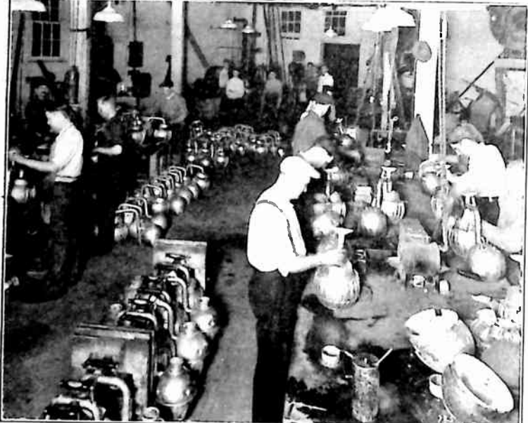
Assembly line where all soldering is done.
