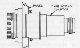
Figure 3. Panel connector mounted with a Type 900-Q Adaptor.
