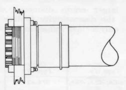
Figure 4. Panel connector mounted with flange behind panel.
