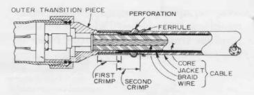
Section view of a GR874 connector attached to a coaxial cable. The larger-diameter second crimp still grips the lacket securely, without reducing the diameter of the braid.
