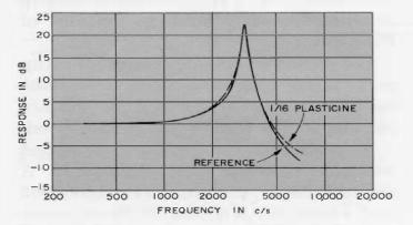
Figure 4. Frequency response of Type 1560-P52 Vibration Pickup attached by means of 1/16inch-thick layer of Plasticine. Reference line shows response of pickup mounted directly on shaker.
