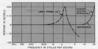
Figure 8. Frequency response of the Type 1560-P53 Vibration Pickup mounted on hand-held 6-inch long by ¼-inch diameter probe. Curve is smoothed average of several responses. Reference line shows response of Pickup mounted directly on shaker.
