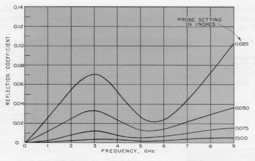
Figure 1. Typical probe reflections at four penetrations.
