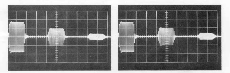
Figures 3a (*left*) and 3b (*right*). Waveforms received by one of two transducers mounted in the end of a closed tube, when the other transducer is driven by a tone burst of (a) 2.95 kc. and (b) 3.0 kc. Fram left to right, the pulses are the direct response, the first reflection from the tube end, and the second reflection from the tube end. Notice the consistency in amplitude of the direct pulse at the two frequencies; compare with Figures 4a and 4b.
