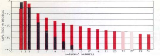
Figure 8. Amplitude of the first 31 Fourier harmonics of a one-cycleon, one-cycle-off tone burst. Switching at zero crossings in black; switching at peak points in red.
