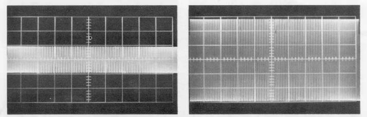
Figures 4a (*left*) and 4b (*right*). Waveforms produced in the same manner as those in Figure 3, except that the driving signal is a continuous one of (a) 2.95 kc. and (b) 3.0 kc. The variation of amplitude indicates the presence of standing waves, which obscure the transducer's frequency characteristic.
