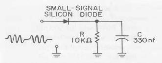
Figure 5a. Example of a simple rectifying circuit tested with a tone burst.
