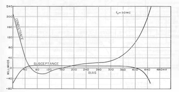
Figure 3. Admittance characteristics of Raytheon CK40 series diodes as a function of bias, measured at 50 Mc. The correct setting of the output line may be performed with an 874-WN3 Short Circuit in place of the diode holder if desired, since this provides substantially the same reference plane as the latter. Alternatively a special (short circuited) diode may be placed in the holder; this choice is better in principle, since any lead inductance effects should be automatically compensated.
