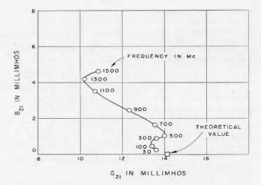
Figure 10. Forward transadmittance versus frequency for a Type 874-G10 Attenuator Pad.
