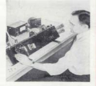
The Transfer-Function Meter described in this issue is a completely new, null-type device, which opens up a new field of measurement. The cover photograph shows the Transfer-Function Meter set up for the measurement of transistors at 400 Mc.
