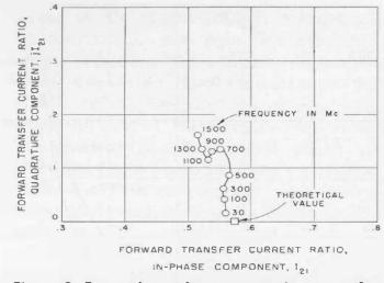
Figure 9. Forward transfer current ratio versus frequency for a Type 874-G10 Attenuator Pad.
