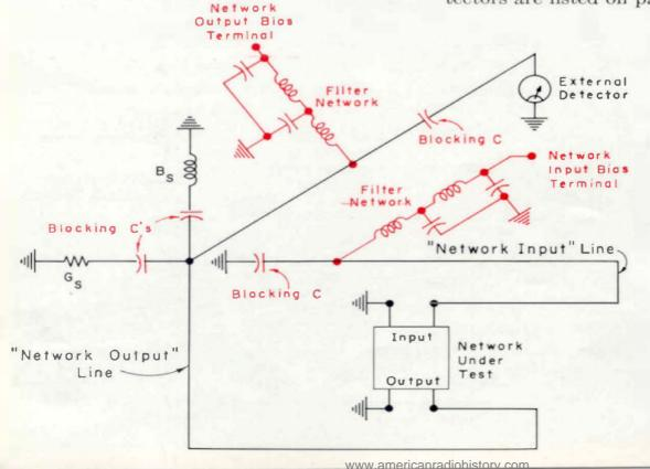
Figure 4. Schematic diagram of d-c circuits of the Transfer-Function Meter.
