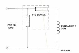
Figure 7 - Typical Degaussing Circuit
