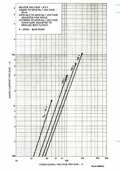
Figure 2 – Typical Drive Characteristics, Cathode-Drive Service
