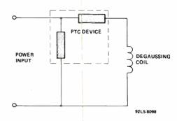
Figure 7 – Typical Degaussing Circuit
