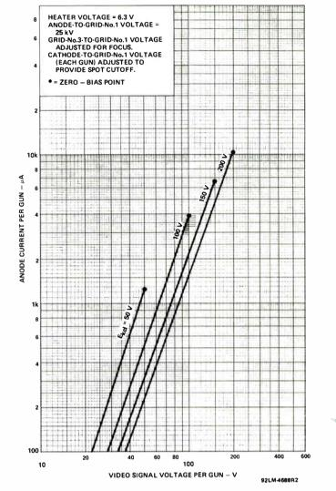
Figure 2 - Typical Drive Characteristics, Cathode-Drive Service
