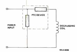
Figure 7 – Typical Degaussing Circuit
