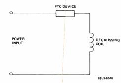
Figure 7 – Typical Degaussing Circuit
