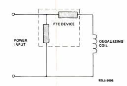
Figure 7 - Typical Degaussing Circuit
