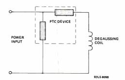
Figure 7 – Typical Degaussing Circuit
