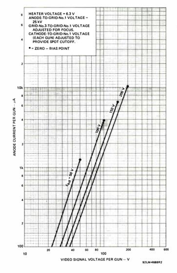
Figure 2 - Typical Drive Characteristics, Cathode-Drive Service
