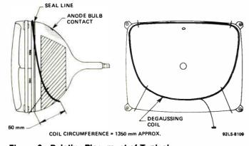
Figure 6 - Relative Placement of Typical Tilted "Z" Degaussing Coli
