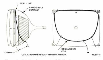
Figure 6 - Relative Placement of Typical Tilted "Z" Degaussing Coll
