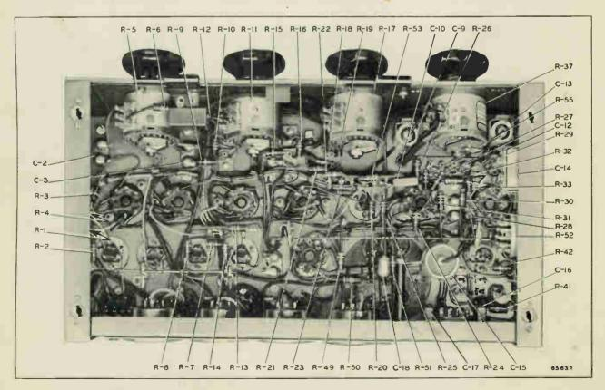
Figure 10—Location of parts, bottom view with attenuator caps removed
