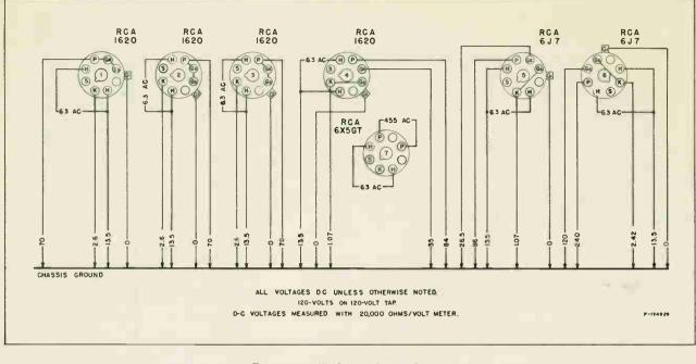
Figure 8—Tube socket voltages
