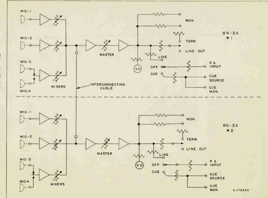
Figure 7—Block Diagram of Parallel Connections
