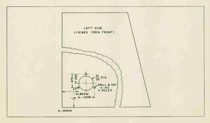
Figure 6—Dimensions of Mounting Holes for Receptacle
