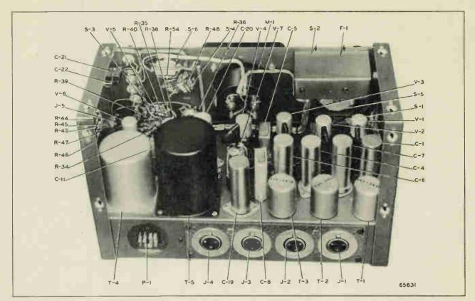
Figure 9-Location of parts, rear view
