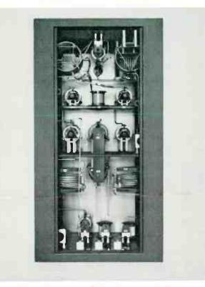
Phasing Cabinet showing simplicity of design and layout. Custom equipment provides maximum stability for dependable AM operation, for three tower, 10-KW stations.
