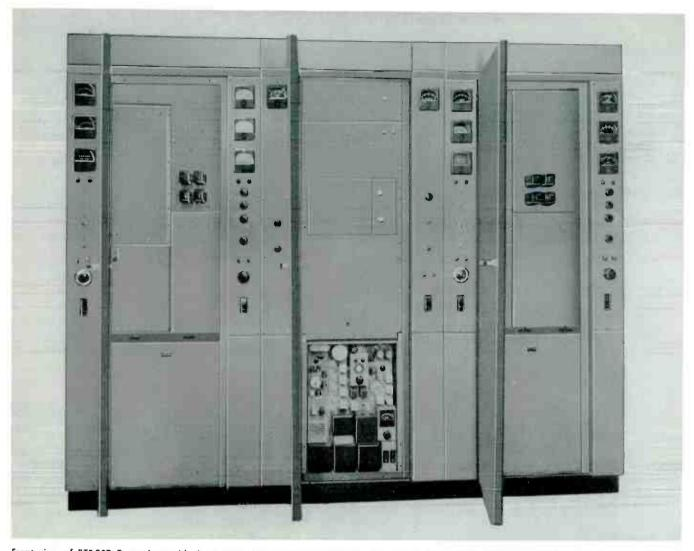
Front view of BTF-20D Transmitter with doors open. In Center cabinet is seen the "Direct FM" exciter which is housed here together with 400-watt driver. Two 10-kw amplifiers with associated power supplies and blowers occupy matching cubicles on right and left.
