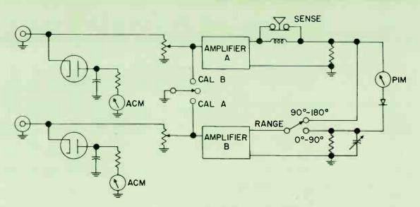
Functional block diagram of the Model 108-E Phase Monitor.
