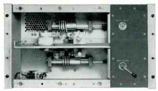
BTF-5D 250-Watt IPA with front panel removed.
