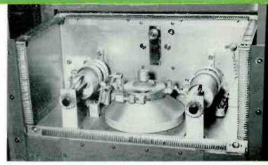
R-f cavity with shielded cover removed.
