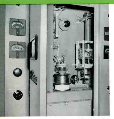
BTA-5T PA stage comprising one 5762 tube used for the high efficiency operation. The coil shown on the right, is the third harmonic coil used in the plate circuit of the PA to increase efficiency by shaping the plate waveform.
