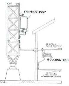
Typical installation of Sampling Loop and Isolation Coil.
