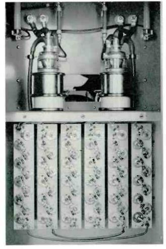
a step-start and damping circuit. This at one time was only available in the higher-power transmitters, but now longer life and added reliability are provided in the BTA-5U/10U with the incorporation of this circuit for the suppression of starting transients. The damping circuit and the primary line reactors afford continuous protection against possible operational transients.
