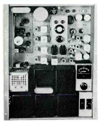
BTE-10B Exciter including self-contained semiconductor d-c power supply is housed on hinged vertical chassis which provides instant accessibility to all components and circuits. The built-in scope permits constant observation of the AFC circuits. The meter, in the lower right side, is used to check all important circuit constants.
