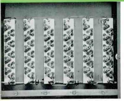
View of Silicon Rectifier Chassis. The silicon cells offer improved performance since they are particularly resistant to aging, moisture and wide temperature variations.
