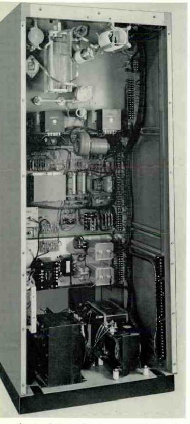
Rear view of BTA-1R1, with rear panels removed, showing vertical construction and accessibility of component parts.
