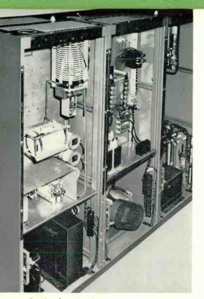
Rear view of transmitter showing reach-in accessibility to transmitter facilities. The modulation transformer and final PA tank circuitry are seen in foreground, rear of modulator and blower in center cabinet, while heavier components of driver are shown mounted on floor of third cabinet.
