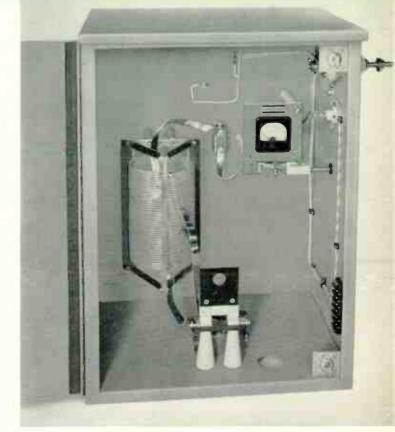
Basic 1 KW Antenna Tuning Unit, MI-27767-A.
