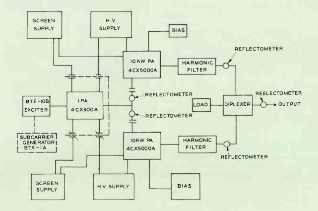
Block diagram of BTF-20D FM Transmitter.
