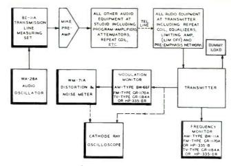
Test set-up for transmitter aural measurements.
