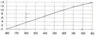
Voltage as a function of Phase Angle for 180°-90° Range.
