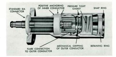
Cutaway view showing typical features common to most Heliax connectors. For example, friction type inner connectors can separate due to differential expansion. This is prevented in Heliax connectors by means of an extra heavy tefton anchor. No special tools or skills are required to install Heliax connectors.
