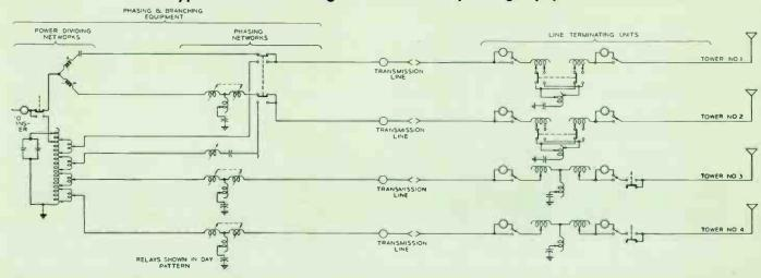
Typical schematic diagram of antenna phasing equipment.
