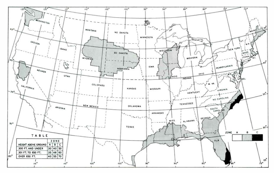
The above map and table, extracted from EIA Standard RS-222, gives minimum windload design pressures in pounds per square foot on flat surfaces with no ice for the zones indicated. This map, as well as the table, must be interpreted in view of local knowledge and applicable building codes. See Table 1 of RS-222 for zone boundaries listed by state and county.
