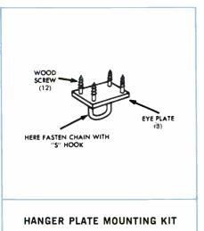
For attaching Hanger and Fastener Kit to plaster or wood surfaces. Consists of three steel eye plates and mounting hardware.
