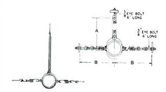
Spring hanger for horizontal suspension of single line. Anchored at three points. Complete with eye bolts and springs.
