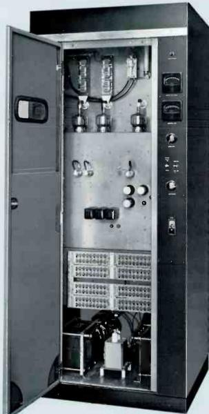
Rear view of BTA-1R2, with rear panels removed, showing vertical construction and accessibility of component parts.
