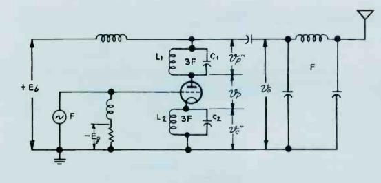
Simplified schematic of the new high efficiency PA stage. The adjustment of the circuit differs from a conventional class "C" only in that the coils  $L_1$  and  $L_2$  are resonated for maximum efficiency.
