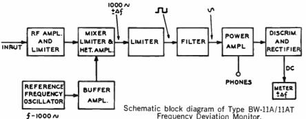
quick check on all circuits. When the monitor is working normally and this button is pressed, the meter deflection increases by approximately 5 Hz. A change appreciably different from 5 Hz indicates a defective circuit.
