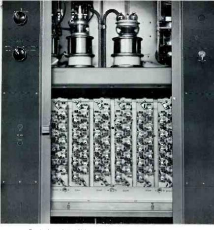
Front view of the Silicon Rectifier Chassis of the BTA-5T1. The silicon cells offer improved performance since they are particularly resistant to aging, moisture and wide temperature variations.
