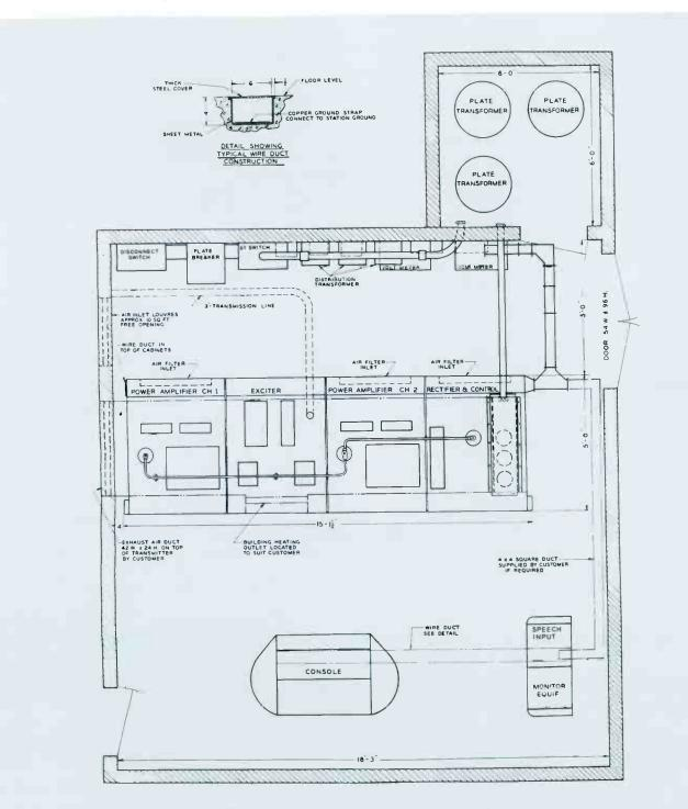
Typical floor plan for the BTA-50H1 Transmitter.
