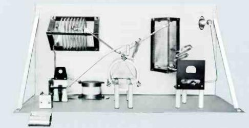
Line Terminating Unit installed on open panel.
