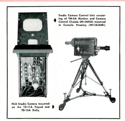
A typical single studio might be arranged by the addition of one studio camera chain, tripod and dolly and equipment rack for power supplies. The studio camera control unit may be added as a "fifth" section to the "Basic-Buy" console, in cases where the studio can be located as a part of, or adjacent to the "Basic Buy" transmitter room.
