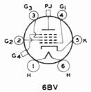
PIN 1: HEATER PIN 2: GRID NO.2 PIN 3: GRID NO.3 PIN 4: GRID NO.1 PIN 5: CATHODE PIN 6: HEATER END CAP: PATTERN ELECTRODE SIDE CAP: GRID NO.4
