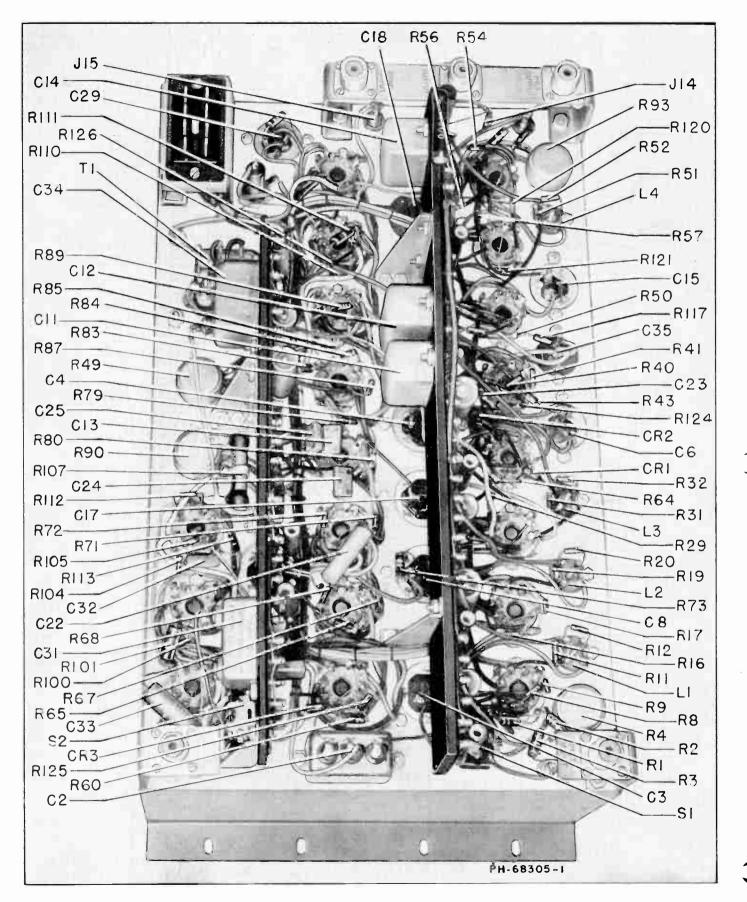
Figure 5-TA-5C Stabilizing Amplifier, Rear View
