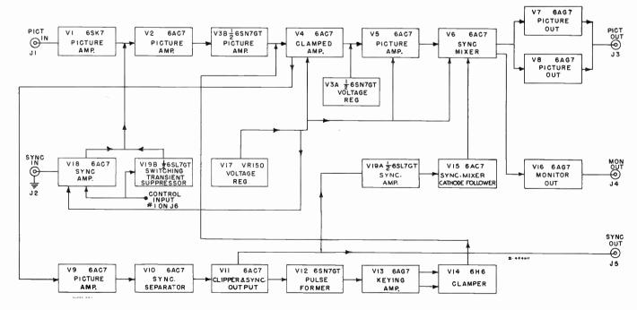
Figure 2-TA-5C Stabilizing Amplifier, Block Diagram
