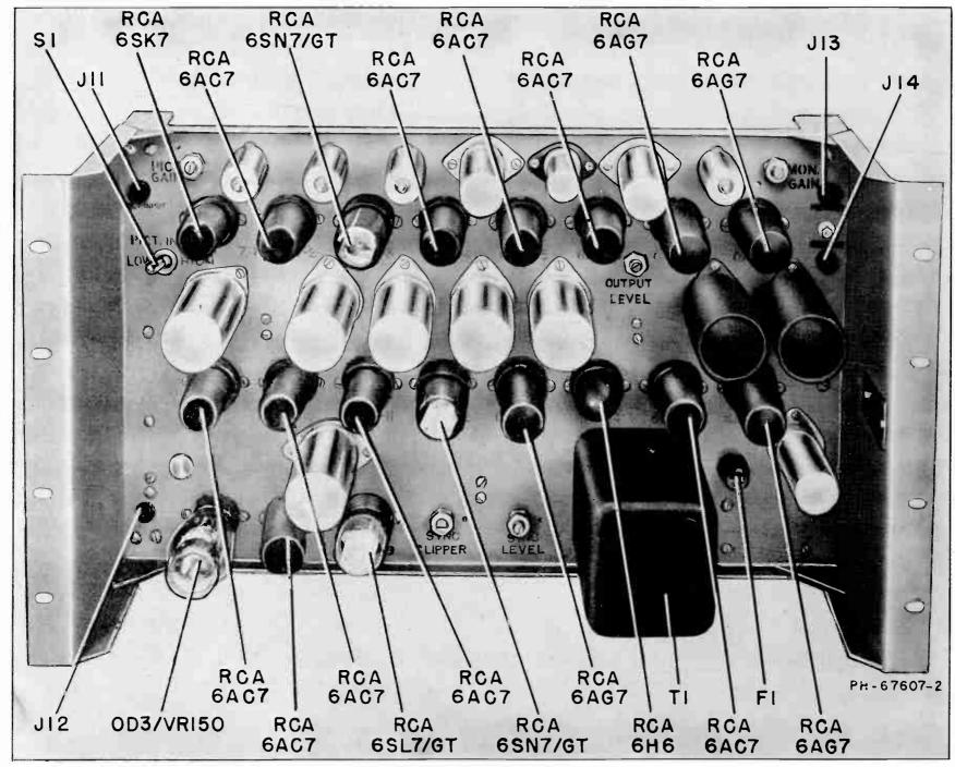
Figure 1—TA-5C Stabilizing Amplifier, Front View
