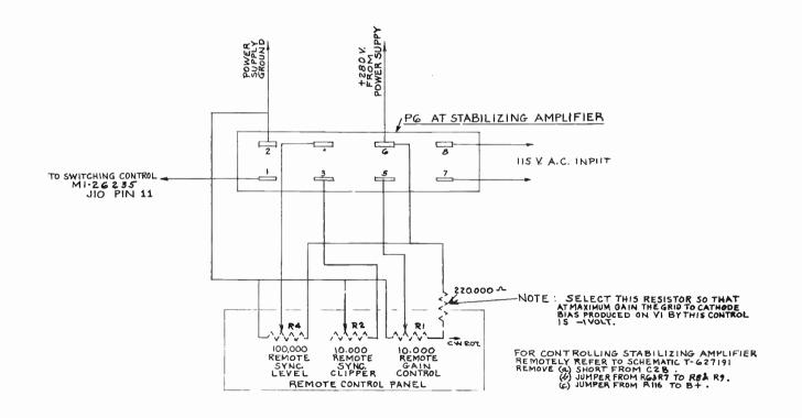
Figure 4-Remote Control Connections
