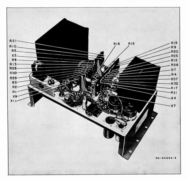
Figure 8—Type 580-D Regulated Power Supply, Rear Right Oblique View
