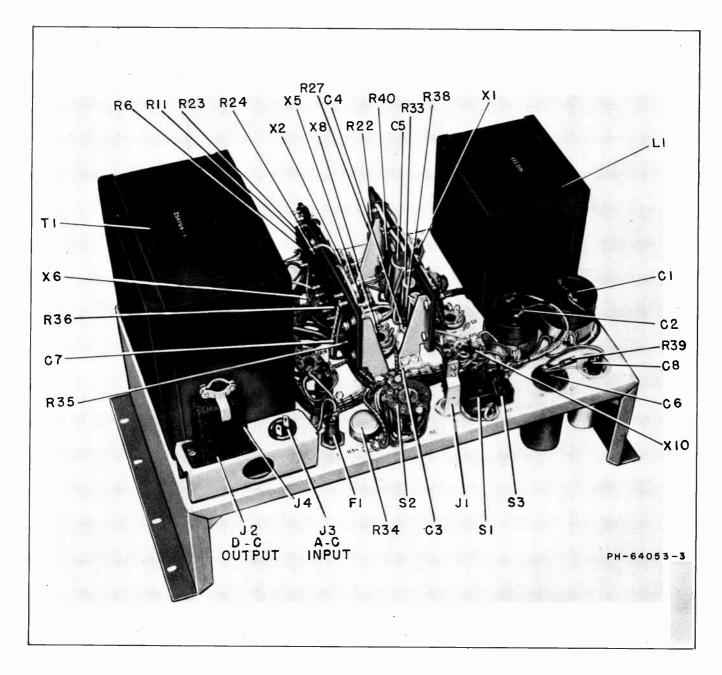
Figure 7–Type 580-D Regulated Power Supply, Rear Left Oblique View
