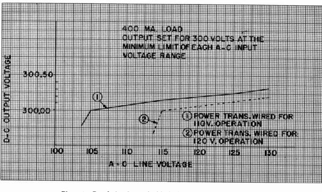
Figure 2-Regulation Curve of a Typical Unit Showing Output Voltage Versus Line Voltage
