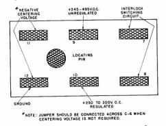
Figure 6—D-C Output Receptacle Connections
