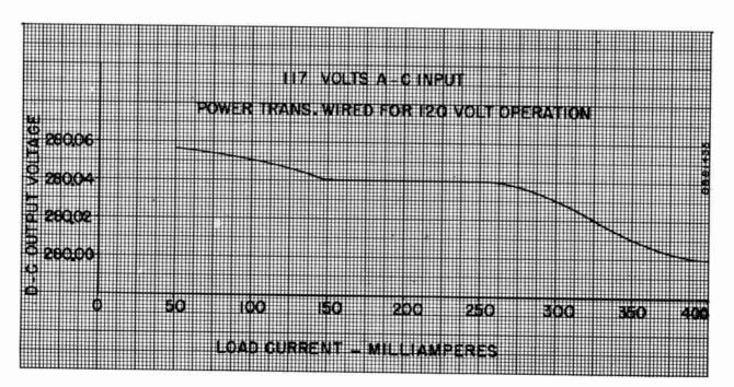
Figure 3–Regulation Curve of a Typical Unit Showing Output Voltage Versus Load Current
