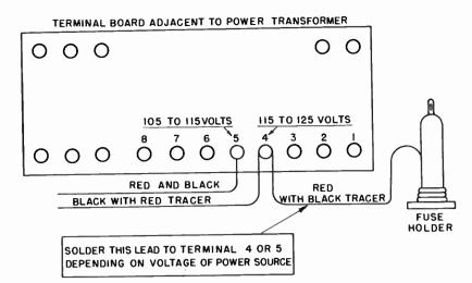
Figure 5–Terminal Board Connections for 105 to 115 Volts or 115 to 125 Volts Operation
