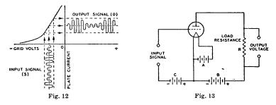
amplification, or gain, provided by the tube. The voltage amplification due to the tube is expressed by the following convenient formulas:
