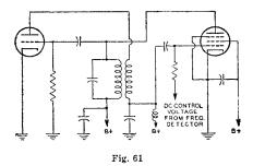
plate current of the reactance tube is shunted across the oscillator tank circuit. Because the plate current and plate voltage of the reactance tube are almost  $90^{\circ}$  out of phase, the control tube affects the tank circuit in the same manner as a reactance. The grid bias of the tube determines the magnitude of the effective reactance and, consequently, a control of this grid bias can be used to control the oscillator frequency.
