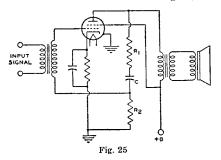
The application of the constantvoltage type of inverse feedback to a power output stage using a single beam power tube is illustrated by Fig. 25. In this circuit,  $R_1$ ,  $R_2$ , and C are connected across the output of the 6L6 as a voltage divider. The secondary of the grid-input transformer is returned to a point on this voltage divider. Capacitor C blocks the dc plate voltage from the grid. However, a portion of the tube's af output voltage, approximately equal
