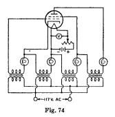
give a high-resistance short, it is desirable that the indicating lamps operate on very low current. It is also desirable to maintain the filament or heater of the tube at its operating temperature during the short-circuit test, because short-circuits in a tube may sometimes occur only when the electrodes are heated.
