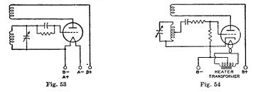
produced by electrostatic or electromagnetic coupling between the grid and plate circuits. When sufficient energy is fed back to more than compensate for the loss in the grid circuit, the tube will oscillate. The action consists of regular surges of power between the plate and the grid circuit at a frequency dependent on the circuit constants of inductance and capacitance. By proper choice of these values, the frequency may be adjusted over a very wide range.
