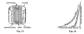
for modulation-distortion, the cause is usually the last intermediate-frequency stage. The characteristics of remote-cutoff types are such as to enable them to handle both large and small input signals with minimum distortion over a wide range.
