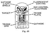
contain two main parts: (1) a triode which operates as a dc amplifier and (2) an electron-ray indicator which is located in the bulb as shown in Fig. 49. The target is operated at a positive voltage and therefore attracts electrons from the cathode. When the electrons strike the target they produce a glow on the fluorescent coating of the target. Under these conditions, the target appears as a ring of light.
