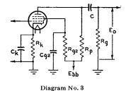
voltage of from 15 to 40 volts with respect to the cathode. The voltage output at  $f_1$  for "n" like stages equals  $(0.7)^n E_0$  where  $E_0$  is peak output voltage of final stage. For an amplifier of typical construction, and for  $R_p$  values of 0.1, 0.25, and 0.5 megohm, approximate values of  $f_2$  are 20000, 10000, and 5000 cps, respectively.
