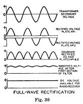
through plate No. 1 on one half-cycle when plate No. 1 is positive with respect to the cathode, and through plate No. 2 on the next half-cycle when plate No. 2 is positive with respect to the cathode. Because the current flow to the filter is more uniform in the full-wave circuit than in the half-wave circuit, the output of the full-wave circuit requires less filtering. Rectifier operating information and circuits are given under each rectifier tube type and in the CIRCUIT SECTION, respectively.
