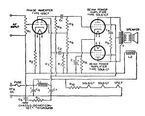
$\begin{array}{l} C_1 \ C_2 = 0.006 \ \mu f \\ C_3 = 25 \ \mu f, \ \text{electrolytic, } 25 \ v. \\ C_4 = 0.035 \ \mu f \\ C_5 = 0.1 \ \mu f, \ \text{paper, } 150 \ v. \\ C_6 = 0.2 \ \mu f, \ \text{electrolytic, } 150 \ v. \\ C_7 = 4 \ \mu f, \ \text{electrolytic, } 150 \ v. \\ C_7 = 4 \ \mu f, \ \text{electrolytic, } 150 \ v. \\ L_1 = \ Filter \ choke, \ 10 \ henries \ at \\ 125 \ ma., \ 60 \ ohms \end{array}$
