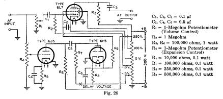
output voltage across the primary of the output transformer: first, when a 400-cycle signal is applied to the input, and second, when a 100-cycle signal of the same voltage as the 400-cycle signal is applied to the input. The correct value of capacitance is the one which gives equal output voltages for the two signal inputs. In practice, this value is usually found to be in the order of 0.05  $\mu$ f.
