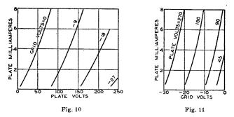
Dynamic characteristics include amplification factor, plate resistance, controlgrid—plate transconductance and certain detector characteristics, and may be shown in curve form for variations in tube operating conditions.
