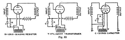
the plate current in the case of a triode, or to the sum of the plate and screen currents in the case of a tetrode, pentode, or beam power tube. Since the voltage drop along the resistance is increasingly negative with respect to the cathode, the required negative grid-bias voltage can be obtained by connecting the grid return to the negative end of the resistance.
