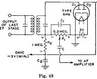
a comparatively slow rate. The avc voltage therefore cannot vary at frequencies as high as the audio range but can vary at frequencies high enough to compensate for most fading. Thus the filter permits the avc circuit to smooth out variations in signal due to fading, but prevents the circuit from smoothing out audio modulation.
