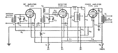
$R_1 = 100000$  ohms, 0.5 watt  $R_2 = 2 - 5$  megohms, 0.5 watt  $R_3 = 0.25$  megohm, 0.5 watts  $R_4 = Volume control, potenti-$ ometer, 0.5 megohm $<math>R_5 R_7 = Potentiometers, 50000$ ohms
