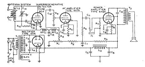
C<sub>1</sub> C<sub>2</sub>= 0.1  $\mu$ f, paper, 400 v. C<sub>3</sub> C<sub>4</sub>= 100  $\mu\mu$ f, mica, 500 v. C<sub>6</sub> C<sub>6</sub> C<sub>7</sub>= 20  $\mu$ f, electrolytic, 450 v.
