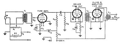
$C_1 = 5 \ \mu f$ , electrolytic, 25 v.  $C_2 = 4 \ \mu f$ , electrolytic, 250 v.  $C_3 = 0.025 \ \mu f$ .  $C_4 = 25 \ \mu f$ , electrolytic, 25 v. M = Microphone, double-button B. Betrovicence 500 ebras
