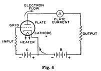
with a signal, the plate current varies with the signal. Because a small voltage applied to the grid can control a comparatively large amount of plate current, the signal is amplified by the tube. Typical three-electrode tube types are the 6C4, 6J5, and 2A3.
