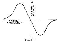
Because this type of FM detector is sensitive to amplitude variations in the rf carrier, a limiter stage is frequently used to remove most of the amplitude modulation from the carrier. (See Limiters under Amplification.)
