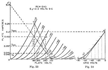
**Example:** Fig. 23 illustrates the application of the method to a pair of 2A3's operated at  $E_o = 300$  volts. The tubes have a plate-dissipation rating each of 15 watts. The method is to erect a vertical line at  $0.6E_o$ , or at 180 volts, which intersects the  $E_c = 0$  curve at the point  $I_{max} = 0.26$  ampere. Using the simplified formulas, we obtain
