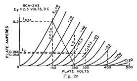
The method for calculating power output for triodes in push-pull class A operation is as follows: Erect a vertical line at  $0.6E_0$  (see Fig. 20), intersecting the  $E_c = 0$  curve at the point  $I_{max}$ . Then,  $I_{max}$  is determined from the curve for use in the formula
