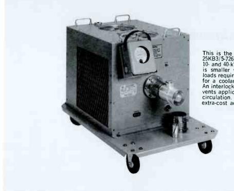
This is the 20 kW system (Bird 8644/4805/ 25KB3/5-726) and is representative of the 10- and 40-kW loads as well. The 10-kW load is smaller while the 40- is larger. These loads require a source of commercial power for a coolant pump within the enclosure. An interlock connection, properly used, pre-vents application of power without coolant circulation. Dolly shown is optional as an extra-cost accessory.
