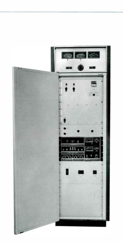
Heart of the BTF-3E1 Transmitter is the solid-state exciter, shown here with stereo and two SCA modules in place.
