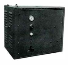
Engineered and manufactured specifically for pressurizing RF transmission lines, these two compressor/dehydrator units differ only in output capacity and physical dimensions. The units deliver dry, compressed air at the rate of one or two cubic feet per minute  $(0.028 \text{ or } 0.056 \text{ m}^3)$ .
