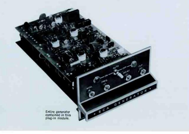
The BTX-1B SCA Subcarrier Generator is a plug-in module for the Type BTE-15A FM Exciter System. However, it is offered separately in a self-powered, rack-mount assembly for use with RCA exciters and transmitters of earlier design.
