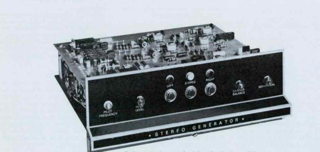
Entire generator contained in this plug-in module.
