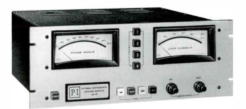
The PM-19 system uses the AM-19 (204) Antenna Monitor as a base and adds to it a PMA-19 Precision Monitor Adapter. The combination of the two units increases resolution and repeatability to onc-tenth degree for phase angle and one-tenth percent for current deviation measurements. The system reads out loop current ratios directly. The system provides both analog and digital readout of all three parameters.
