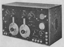
THE IP-501 Receiver shown in the accompanying illustration is a compact unit containing the radio frequency and detecting circuits in a single case. Its range is 250 to 8,000 meters. It is particularly suitable for installations where cost and space factors are of great importance.
