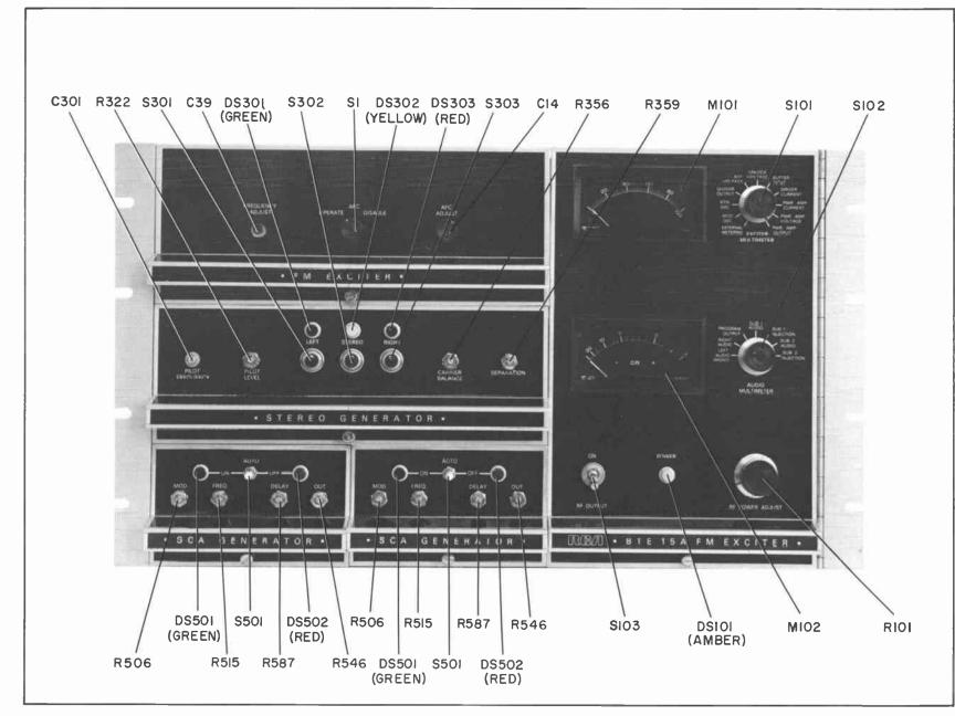
Figure 6. BTE-15A Exciter System, Front View
