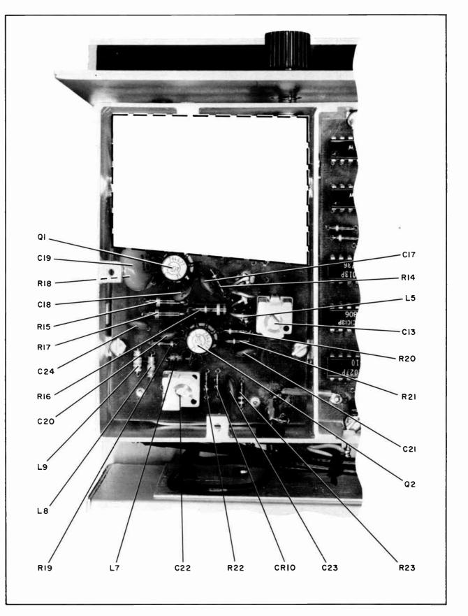
Figure 20. Exciter, Modulated Oscillator Board, Parts Location
