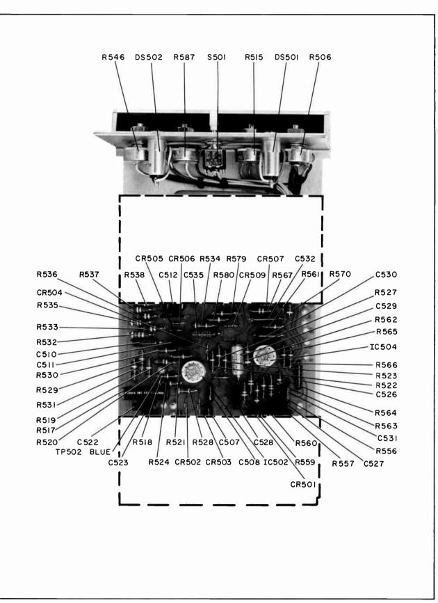
Figure 42. SCA Generator Board, Parts Location
