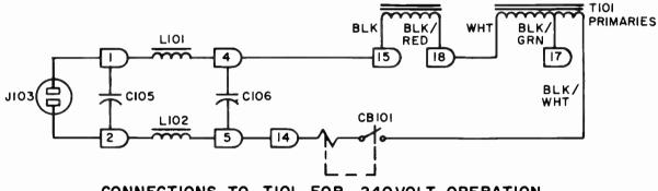
CONNECTIONS TO TIOI FOR 240 VOLT OPERATION
