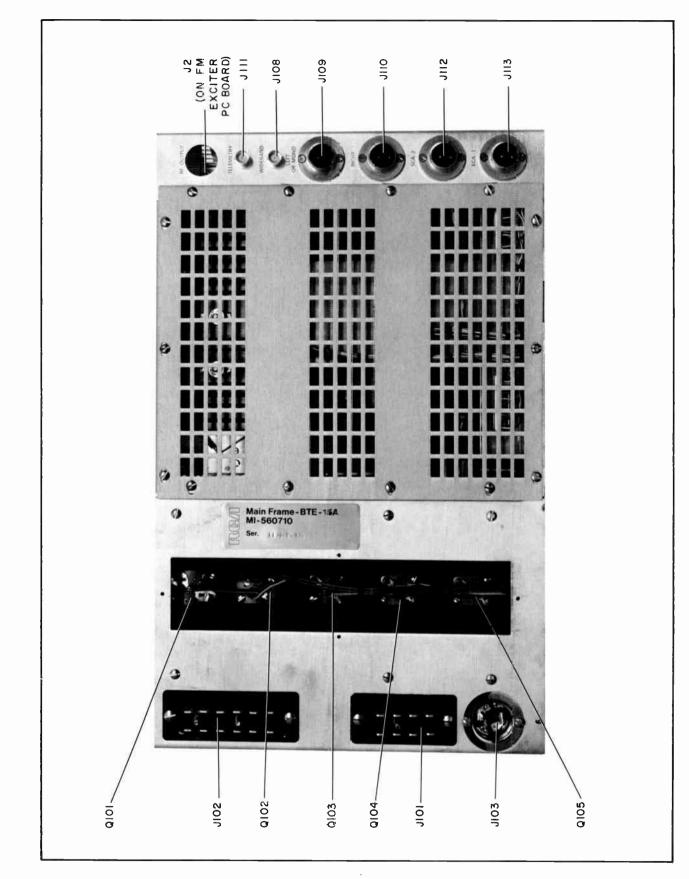
Figure 10. Main Frame, Rear View
