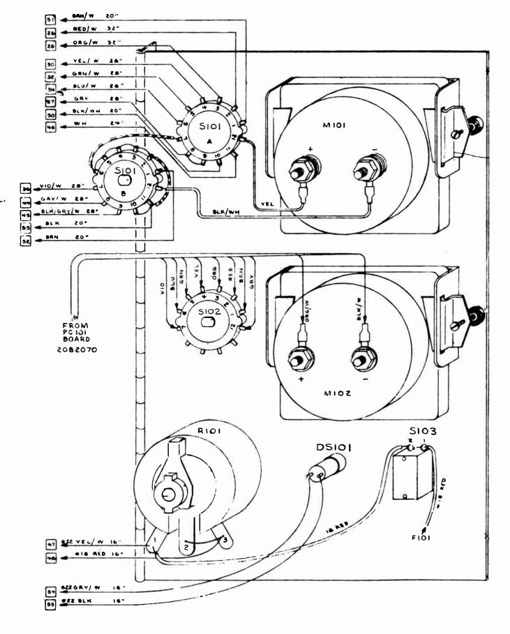
Figure 59. Main Frame Door Assembly, Wiring Diagram
