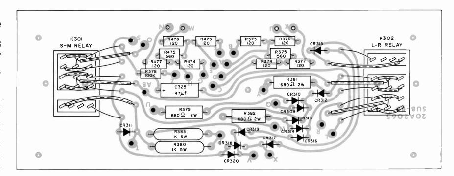
Figure 37. Stereo Generator Sub-Board, Parts Overlay, Bottom
