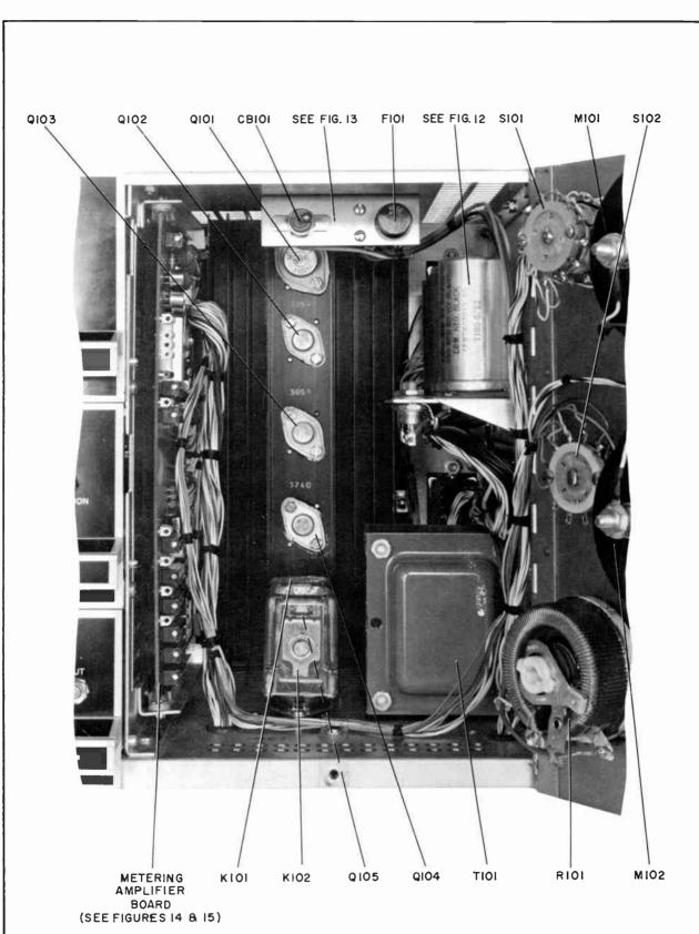
Figure 11. Main Frame, Parts Location
