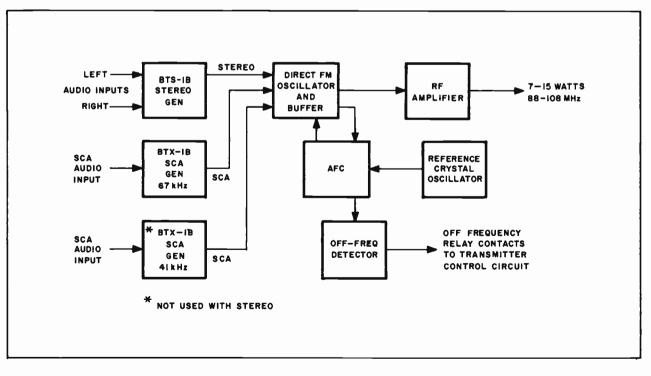
Figure 2. BTE-15A System, Block Diagram
