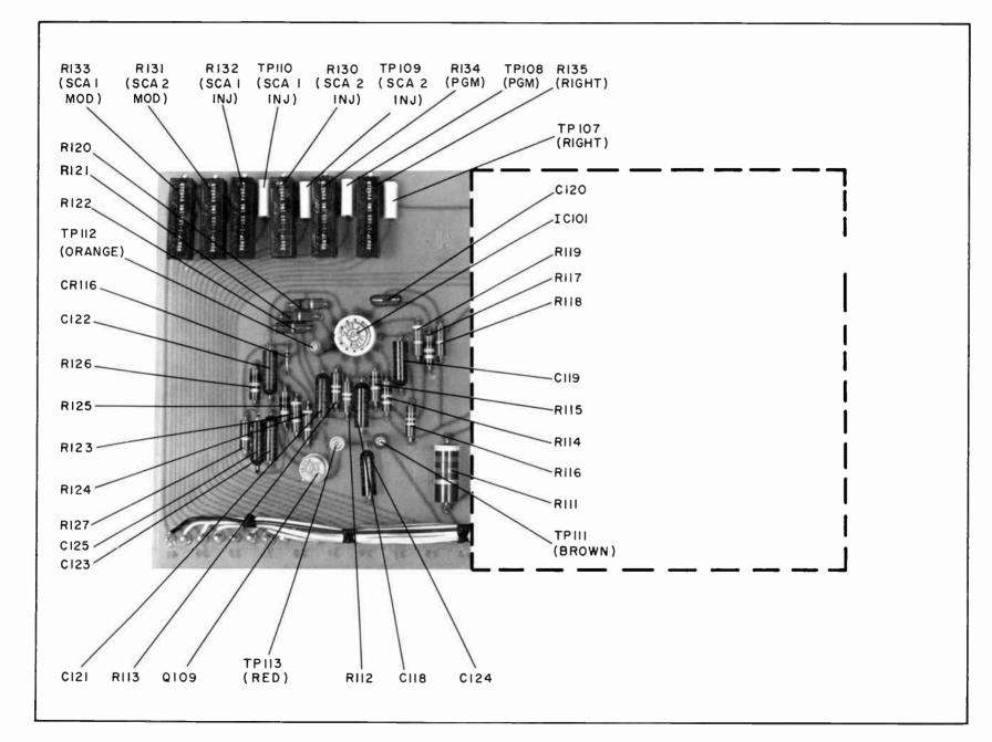
Figure 15. Main Frame Metering Amplifier Board, Parts Location
