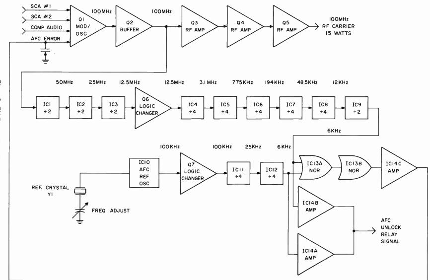
Figure 3. FM Exciter, Simplified Block Diagram
