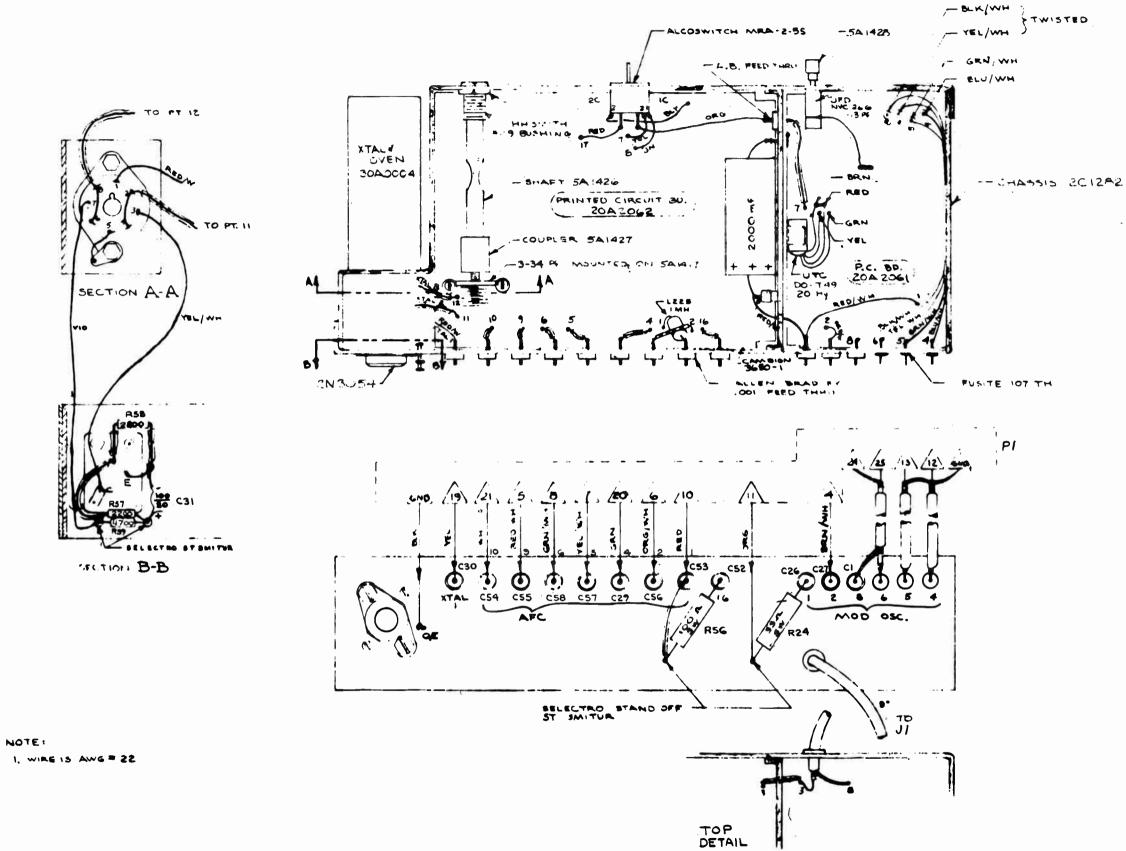
Figure 61. Exciter, Modulated Oscillator and AFC Assembly, Wiring Diagram
