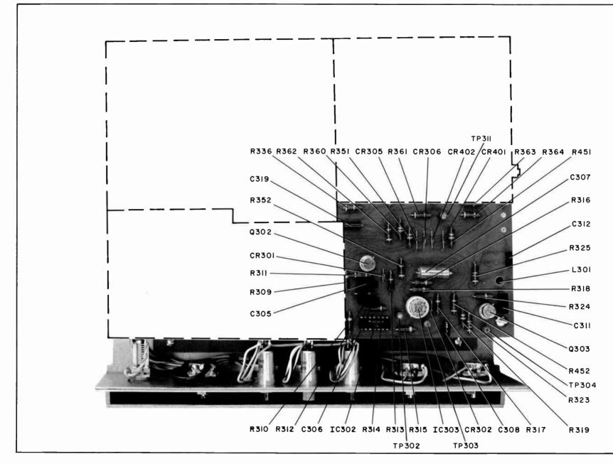
Figure 32. Stereo Generator Board, Parts Location
