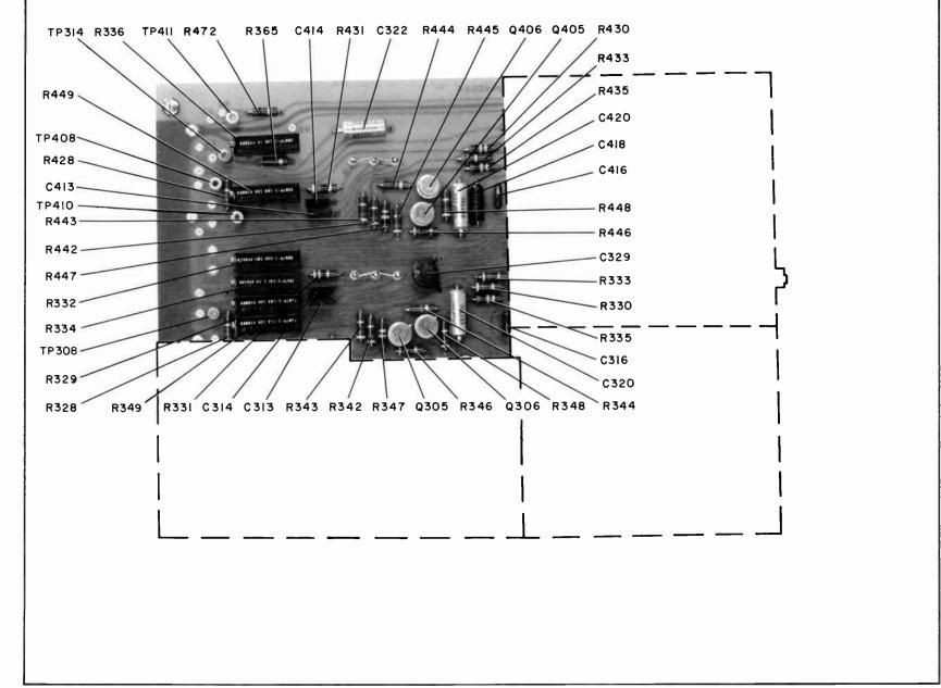
Figure 31. Stereo Generator Board, Parts Location
