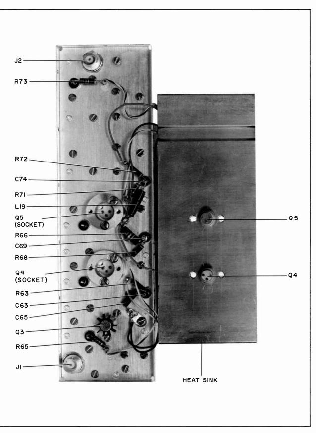
Figure 22. Exciter, RF Amplifier, Parts Location, Top
