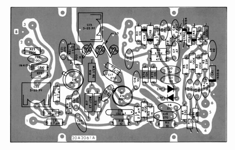
Figure 25. Exciter, Modulated Oscillator Board, Parts Overlay, Bottom
