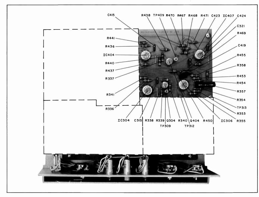
Figure 30. Stereo Generator Board, Parts Location
