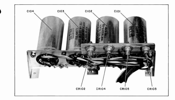
Figure 12. Main Frame, Rectifier and Filter
