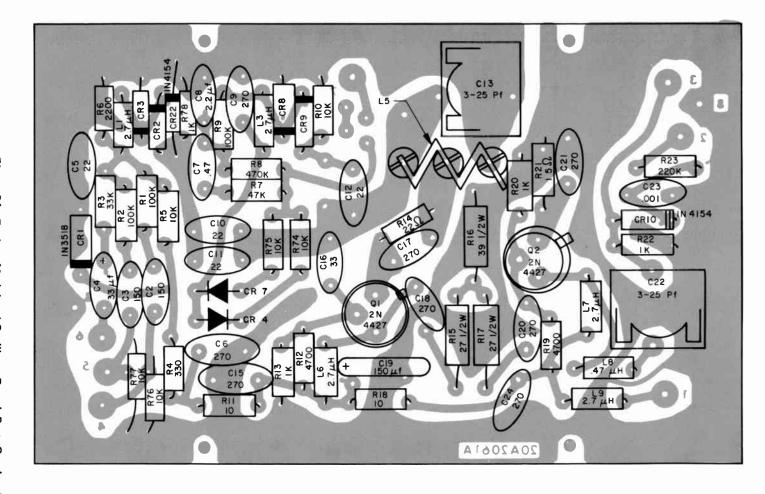
Figure 24. Exciter, Modulated Oscillator Board, Parts Overlay, Top
