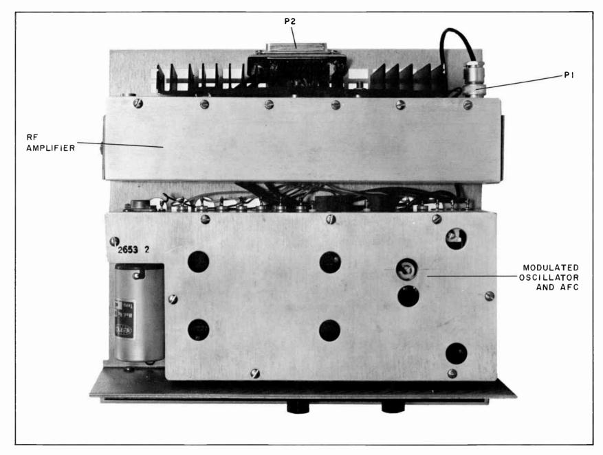
Figure 18. Exciter, Top View
