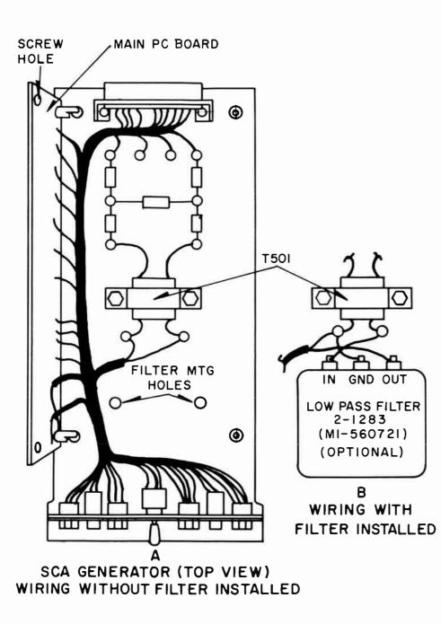
INSTRUCTIONS FOR INSTALLING THE OPTIONAL MI-56072I LOW PASS FILTER IN THE BTX-IB SCA GENERATOR,
