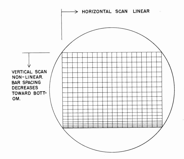
Figure 6 Non-linear Vertical Deflection Checked by Horizontal Bar Spacing
