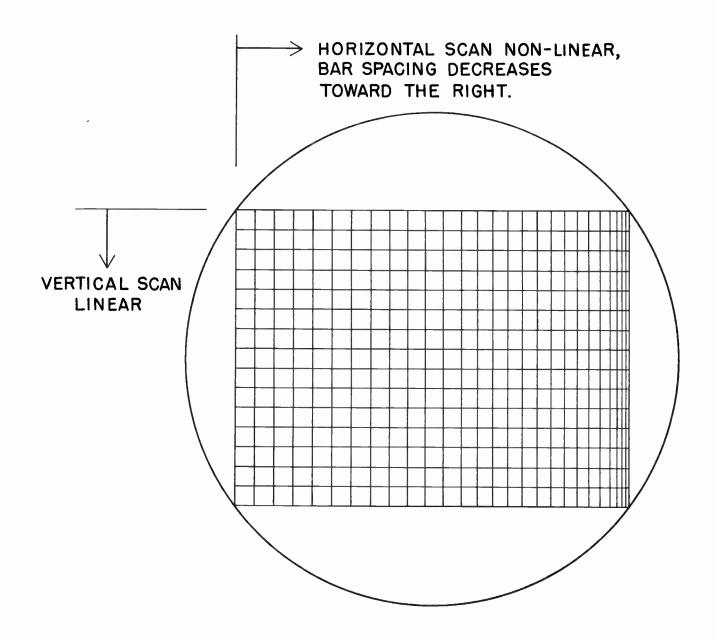
Figure 7 Non-linear Horizontal Deflection Checked by Vertical Bar Spacing
