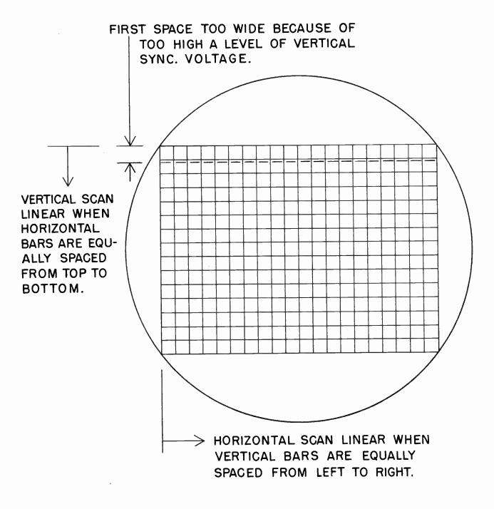
Figure 5 Grating Pattern on Kinescope with Linear Horizontal and Vertical Deflection
