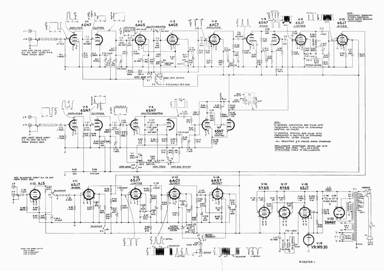
Figure 9A - Schematic WA-3A Grating Generator 1<sup>9</sup> 44 - 52 ,
