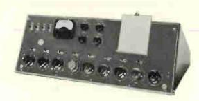
THE "GENERAL-PURPOSE" AUDIO CONSOLETTE BC-3B. Thirteen Inputs-6 microphones, 2 turntables, 2 remate lines, 1 network, 2 utility inputs which may be used for additional turntables, tape, or as required. Eight mixer positions. Built-in power supply. Easily ex-panded for dual channel use by pairing with BC-5A. Convenient script rack.
