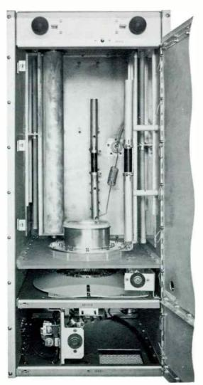
**COMPLETE ACCESSIBILITY**—Rear view of the BTF-5E1 revealing the clean, vertical construction of PA cavity to left and control panel to right.
