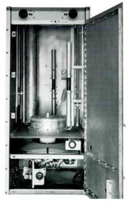
ONLY THREE TUBES BETWEEN EXCITER AND OUTPUT—View showing interior of PA and IPA cabinet with the 4CX15000A ceramic tetrode and two IPA tubes below shelf.
