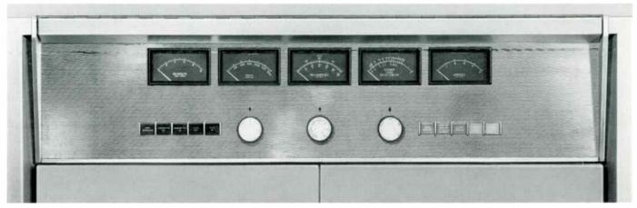
BTF-10E1 Control Panel. Tally lights and push-button controls simplify operation.
