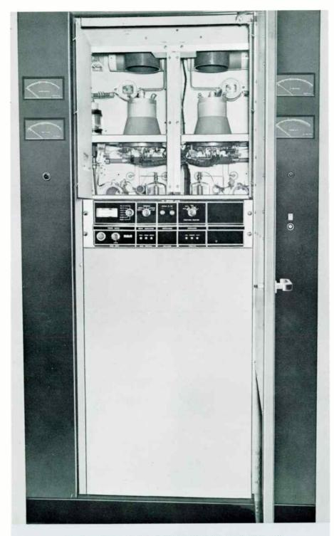
Front section of the exciter-modulator containing all components from oscillator through the driver stages.
