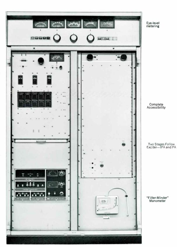
Optional Stereo Sub-Carrier Generator Fully Air Cooled
