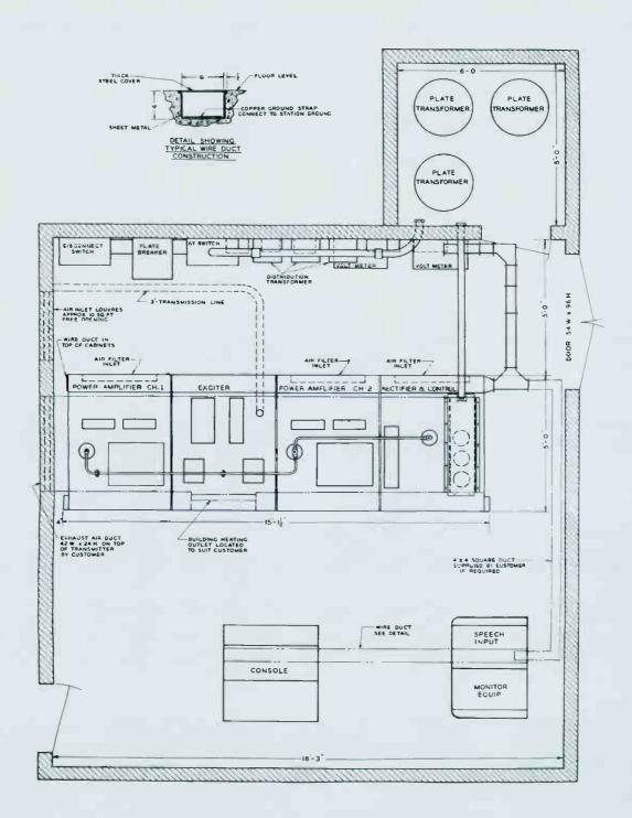
Typical floor plan for the BTA-50J Transmitter.
