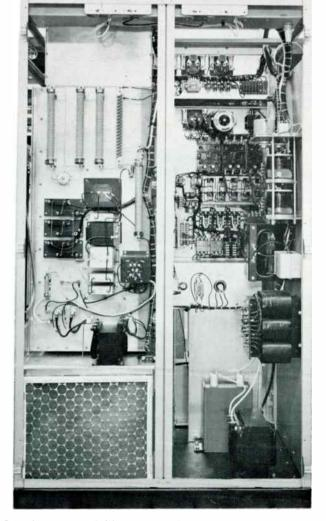
Complete accessibility. Rear view showing one of the amplifiers of the BTF-40E1 revealing the clean, vertical construction of PA cavity to left and control panel to right.
