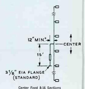
\* Can be made to dimension desired to bring input line to correct support position.
