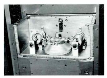
RF cavity with shielded cover removed.
