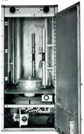
**COMPLETE ACCESSIBILITY**—Rear view of the BTF-10E1 revealing the clean, vertical construction of PA cavity to left and control panel to right.
