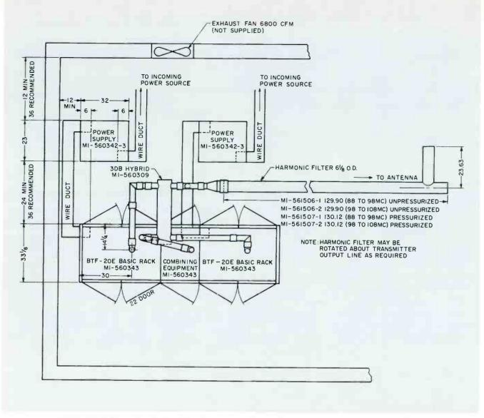
Space-saving floor plan of the BTF-40E. The separate, unitized power supply may be installed in a basement, attic, closet or other convenient place. (Wire duct and fan shown are not furnished.)
