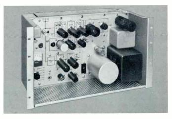
Nine-tube, direct-FM exciter provides unparalleled multiplex performance.
