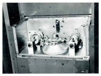
RF cavity with shielded cover removed.
