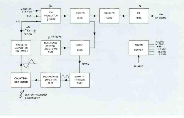
Block diagram of the BTE-10CT FM Transmitter.
