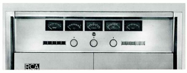
BTF-10E Control Panel. Tally lights and push-button controls simplify operation.
