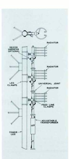
BFA Antenna shown side mounted on a typical uniform cross-section tower.
