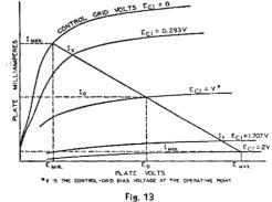
**Power output for pentodes** as Class A amplifiers can be calculated in much the same way as for triodes by means of the following formulas and a special plate characteristic family of curves, illustrated in Fig. 13.
