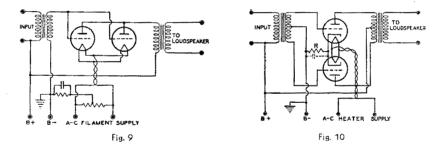
A Class A power amplifier is also used as a driver to supply power to a Class AB or a Class B output stage. Either triodes or pentodes as driver tubes may be used, but triodes are usually preferable since they produce less distortion.
