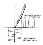
a-c cycle. The 80, 82, 83 and 5Z3 are examples of this type and are called fullwave rectifiers.
