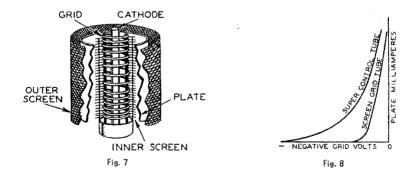
last intermediate-frequency stage. The characteristics of super-control types are such as to enable the tube to handle both large and small input signals with minimum distortion over a wide range. This feature is obtained by a special tube structure which makes possible variation in amplification factor with a change in grid bias. A cross-section of the structure of a typical super-control tube is shown in Fig. 7. This type differs from
