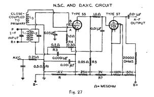
voltage for the 57 a-f amplifier. Under signal conditions, the 55 triode is biased to cut-off. No current flows through load resistor  $R_{\delta}$  so that the 57 operates at maximum plate current—limited, of course, by the minimum bias supplied by the bleeder  $R_{\tau}$ . Under this condition, the 57 amplifies the a-f voltage from diode B and passes it on to the audio-requency stages.
