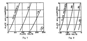
**Dynamic characteristics** include amplification factor, plate resistance, mutual conductance, and certain detector characteristics, and may be shown in curve form for variations in tube operating conditions.
