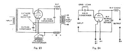
The grid-bias method of detection makes use of a tube which is operated with a grid bias such that the plate current with no signal is practically zero. The bias may be obtained from a cathode resistor (self-bias method), a C battery, or a bleeder circuit. When a signal is applied to the grid, rectification of the carrier occurs in the plate circuit,
