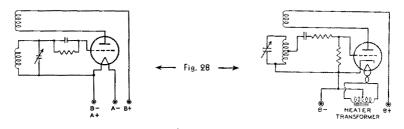
coupling between the input and output circuits. When sufficient feed-back occurs to more than equal the tube losses, the tube will oscillate. The action consists of regular surges of power between the plate and the grid circuit at a frequency dependent on the circuit constants of inductance and capacity. By proper choice of these values, the frequency may be adjusted over a very wide range.
