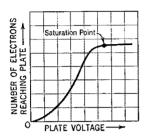
current, or, simply, emission. In most types of tubes, it is impossible to obtain this value by measurement, since the current flow is sufficiently large to change the emitting conditions, or to damage the tube. As a result, emission values in practice are determined at some lower voltage which will not harm the tube. Different results will be obtained if a different cathode voltage or temperature is chosen, since the cathode temperature determines the number of available electrons.
