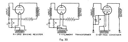
The size of the resistance for self-biasing a single triode can be determined from the following formula:
