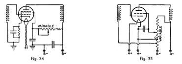
Screen voltage variation for the r-f amplifier stages is sometimes used for volume control of the receiver. Reduced screen voltage lowers the mutual conductance of the tube and results in decreased gain per stage. The voltage variation is obtained by means of a potentiometer shunted across the screen voltage supply. See Fig. 35.
