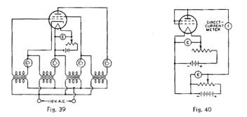
A **mutual conductance test** takes into account a fundamental operating principle of the tube. (This will be seen from the definition of Mutual Conductance on page 7.) It follows that mutual conductance tests, when properly made, permit better correlation between test results and actual performance than does a straight emission test.
