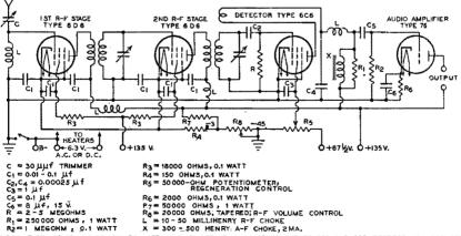
NOTE: TYPES 56, 57, AND 58 MAY BE USED IN THIS CIRCUIT IN PLACE OF THE 76, 806, AND 606 RESPECTIVELY, PROVIDED THEY ARE OPERATED AT THEIR RECOMMENDED HEATER, SCREEN, PLATE AND GRID BIAS VOLTAGES.
