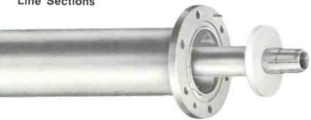
Shipped two sections per package. Each section includes one captive anchor insulator-connector, expansion joint, O-ring gasket, six bolts, nuts, lockwashers.
