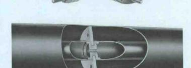
Efficient, precision-built line and line accessories. Featuring an electrically transparent Teflon insulator, this line uses the familiar bolt-flange connection. Insulator characteristics and precise inner-conductor centering allows cutting and re-flanging in the field without a change in operating impedance at the cut.
