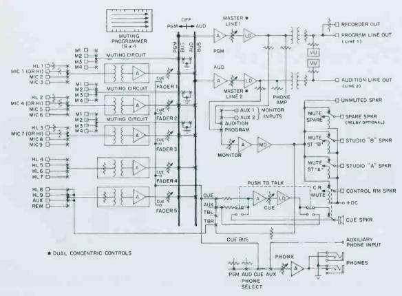
Functional Diagram, Type BC-15D Dual-Channel Mono Console
