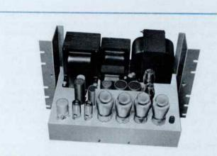
The 200-watt Power Amplifier is a bridging type amplifier using four Type 6550 beam tetrodes in a push-pull, Class AB<sub>1</sub>, circuit. Its exceptional frequency response and low distortion make it ideal for wide-range reproduction of music. When more than one amplifier is used in a system the inputs are paralleled. With 16 decibels of inverse feedback for frequency stabilization, it produces 200 watts of clean audio power.
