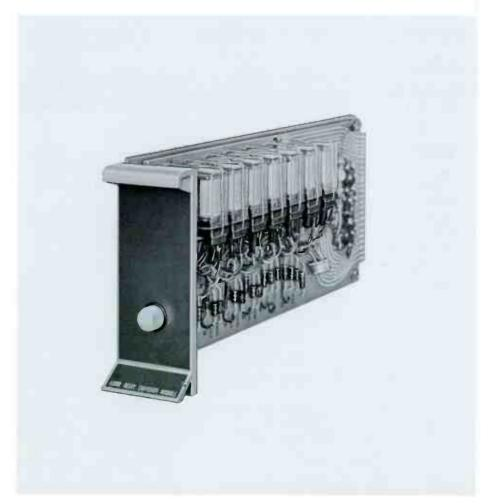
The Audio Relay Switcher Module is a primary component for use in custom relay switching systems. The basic module is a seven-input by one-output switcher and offers a true building block in the development of unlimited audio switcher configurations.
