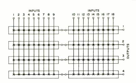
Typical 18x4 switcher using eight of the switcher modules described here. Matrices with 18 modules provide 162x1, 9x18, 81x2 or any arrangement with the same input/output product (see text). Module frames accommodate 18 modules each and frames interconnect easily.
