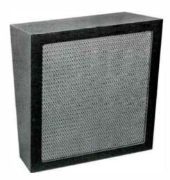
An open-back baffile for any standard 8- or 12-inch loudspeaker, the MI-11414-2 unit is built of one-half-inch plywood finished in textured lacquer. A fiber glass acoustic pad and adapter board are included. Two slotted brackets make mounting easy.
