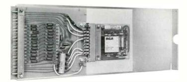
The Iso-Mix Submodule provides 90 dB isolation between inputs and imparts a voltage gain to the signals it passes. Normally this gain factor is either zero or 15 dB, preadjusted. However, an adjustment extends this to any value between zero and 25 dB.
