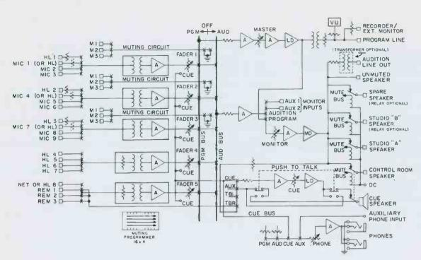
Functional Diagram, Type BC-15 Mono Console
