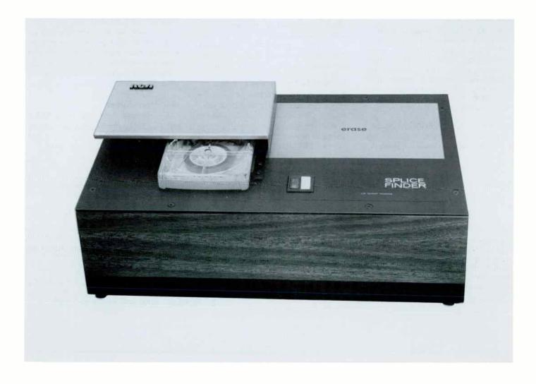
The Type SFE-1 and SFE-2 are devices most useful wherever NAB-type cartridges are recorded. It searches out and locates the tape splice at a point downstieam of the capstan. With the splice so located, it is essentially impossible to record on the splice. This, in turn, eliminates the familiar program discontinuity a recorded splice almost always causes.
