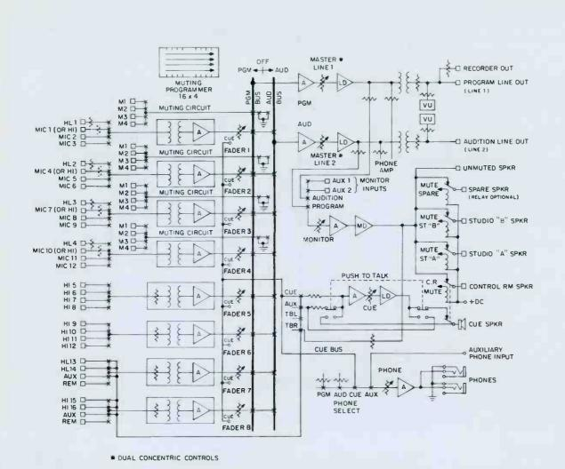
Functional Diagram, Type BC-18D Dual Channel Console
