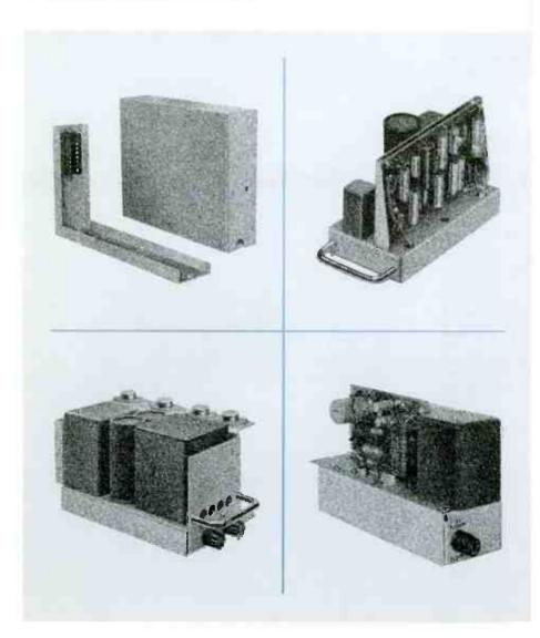
The BA-70 Series of Console Audio Amplifiers are used in the RCA deluxe line of Audio Control Consoles. The amplifiers are offered separately for use in custom-built installations.
