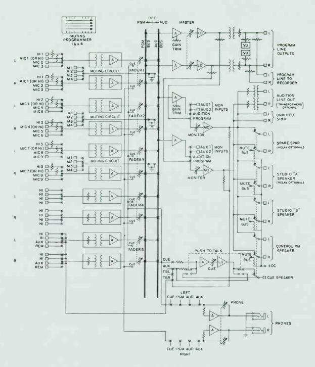
Functional Diagram, Type BC-15S Stereo Console
