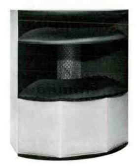
The LC-9 Loudspeaker System is designed for applications where high acoustical level, wide dispersion angle, and extended frequency response are required. The frequency range is covered by separate low and high frequency homs with a crossover point at 500 Hz. A feature of the LC-9 is the particular care with which the high and low frequency horns have been designed to provide matched acoustical wavefronts for smooth response over the entire frequency range.
