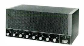
The Type SA-1004 is essentially an extension of the Type SA-1000 described above with four microphone preamps, two auxiliary inputs (for high-level phono or tuner) in addition to bridging input. Separate bass and treble tone controls are also included. The bass control cuts 20 and boosts 15 dB at 50 Hz; the treble control boosts 10 and cuts 20 dB at 20 kHz.
