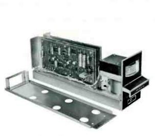
BA-45 Automatic Gain Control Amplifier with Guide Assembly.
