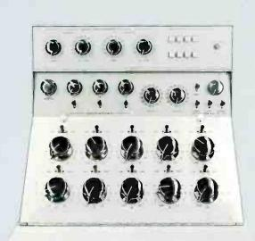
Custom-built ten-input mixer for Station WCAU designed for three-channel output. An accessory panel has been included to provide special utility and switching controls. This panel has been built into a special housing which is mounted on top of basic console form.
