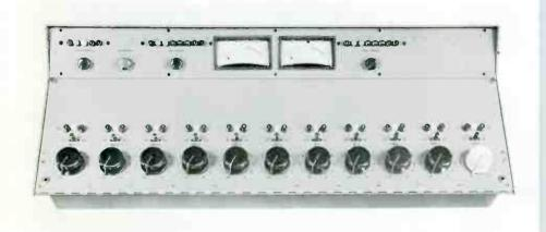
Custom three-channel audio control console shown is designed to match the three-channel master control shown on previous page. The eleven simultaneous mixers on this console and twenty-two on the sole and twenty-two on the master console offer ex-ceptional flexibility for an AM-FM station.
