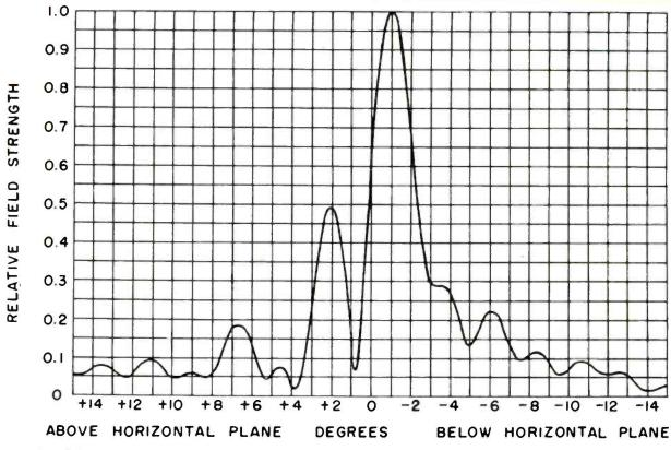
Typical Measured Vertical Field Pattern of an RCA Standard UHF Pylon, Type TFU-278HS, with 1° electrical Beam Tilt.
