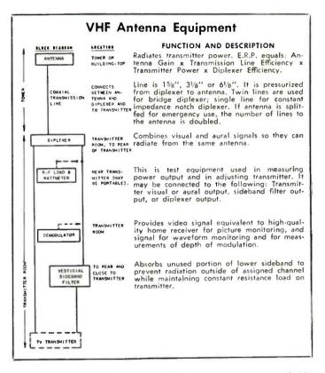
twin transmission lines is used. Other systems are available using either a bridge diplexer, or a Filterplexer.
