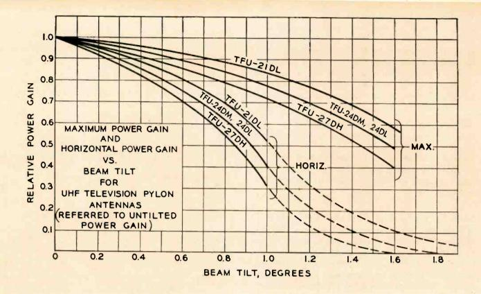
ELECTRICAL BEAM-TILTING is accomplished by moving the inner conductor (feed system) up or down, which shifts the phasing of the signals radiated from the upper and lower halves of the antenna. The effect of this is to raise or lower the beam uniformly around the antenna, thus expanding or contracting the cone of radiated power, umbrella fashion.
