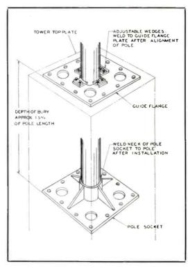
Sketch showing guide flange and pole socket installation.
