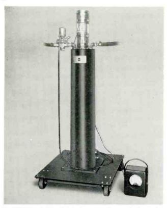
The MI-19199-L/H 6-kw VHF load is mounted on a wheeled truck to aid in changing connections.
