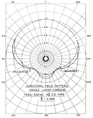
Calculated Pattern and a measured model pattern of a "Cardioid Directional" UHF Pylon.
