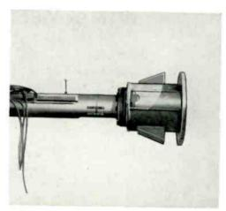
Side view of Flange Pedestal Adapter fastened to base of UHF Pylon. Note hole in adapter near antenna base through which transmission line passes.
