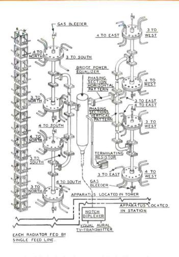
Detailed sketch showing layout of the feed system for an RCA Supergain-14 layers-non-directional.
