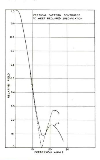
able latitude of control in the vertical pattern shape can be exercised by phasing between sections, by unequal feed line lengths. The power gain in the main load is less than that achieved with uniform phasing and power distribution due to a greater power radiated in other directions. Special vertical patterns are furnished on request.
