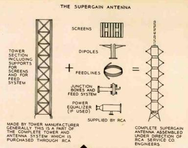
Sketch showing the various elements which go to make up the RCA Supergain Antenna.
