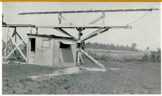
Every RCA UHF Pylon Antenna is subjected to actual vertical field pattern tests by use of a rotatable, built-up platform. Television stations are furnished (free of charge) with a measured curve of their antenna for permanent station engineering records. Antenna shown here under test is a channel #24 directional.
