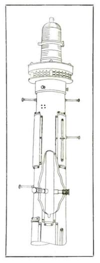
Top view of the RCA UHF Pylon Antenna with beacon removed to illustrate the "Spoke-Type" shorting plug and transmission line. Note that complete harness may be raised by use of lifting ring at top.
