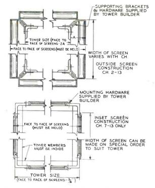
Sketch showing the detail of the RCA Supergain screen which varies from approximately 2½ feet face-to-face width for Channel 12 to 9 feet for Channel 2.
