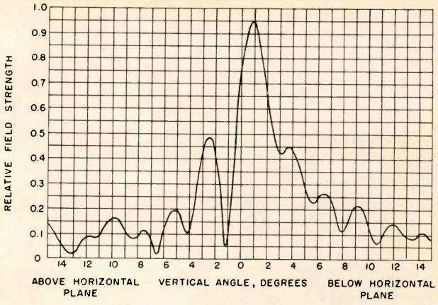
A near ideal vertical field radiation pattern which yields essentially constant field strength versus distance throughout a desired coverage area, custom engineered for an "on-the-air" commercial TV station.
