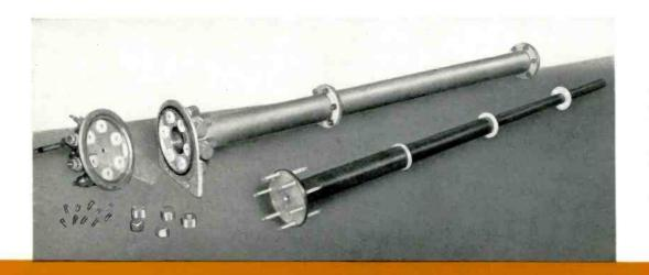
For Superturnstile Antennas, except for 3-section types, the "combined" feedline impedance is different from 51.5 ohms and therefore requires the coaxial transformer shown here which results in an exact impedance match.
