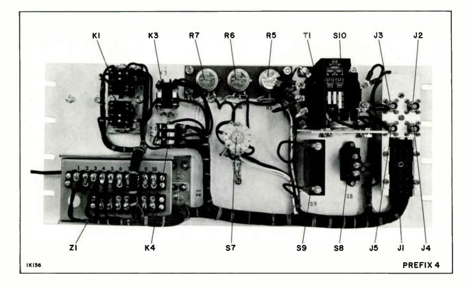
Figure 14. Meter Calibrate Panel, Rear View (Prefix 4)
