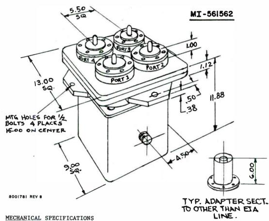
WEIGHT (approx.) MOUNTING **CLEARANCE** CONNECTIONS
