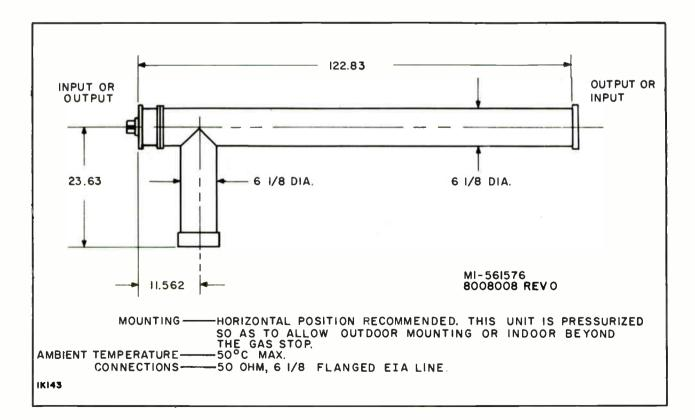
Figure 28. 40 kW Harmonic Filter, Pressurized (MI-561576), Outline Drawing
