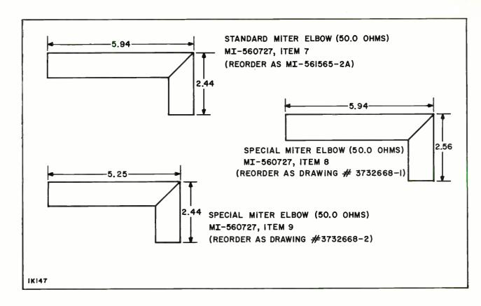
Figure 29. Coaxial Miter Elbows
