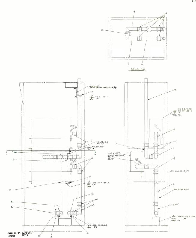
Figure 5. BTF-40E1 Combining Equipment, Installation Assembly
