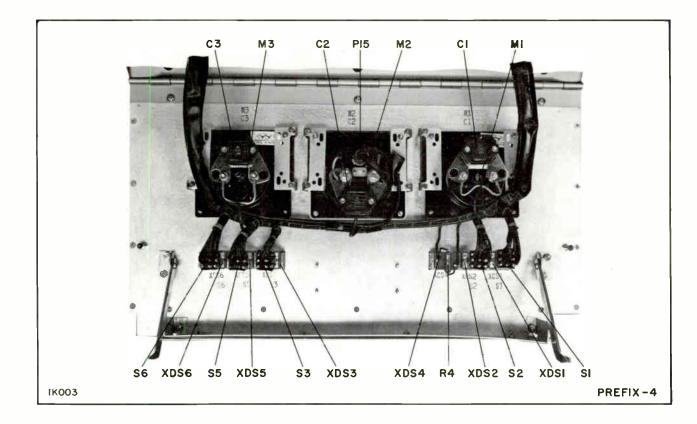
Figure 12. Meter Panel, Rear View (Prefix 4)
