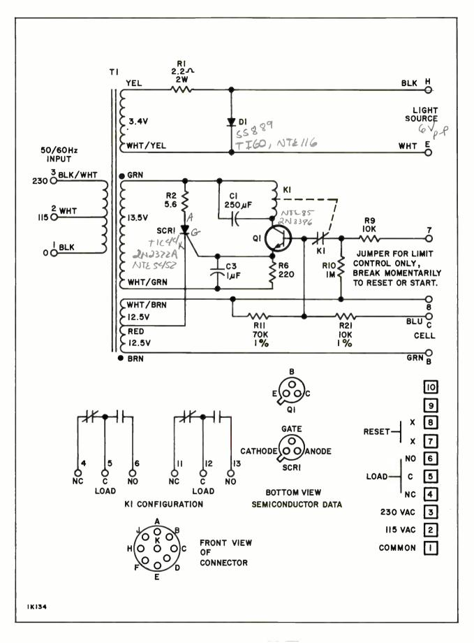
Figure 19. Control Module 4Z1, Schematic Diagram
