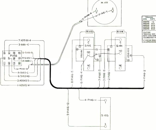
22-26 18-22 14-16 10-12 14-16 .082 .136 .170 .275 .275 Blue Yel, Yel, CAUTION: TERMINAL SIZE MUST BE SELECTED BY REFERENCE TO BOTH AWG WIRE SIZE AND INSULATION DIAMETER, IN ACCORDANCE WITH THIS TABLE.
