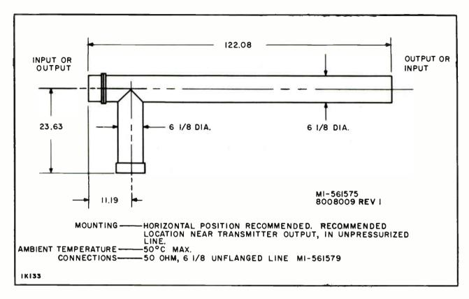
Figure 27. 40 kW Harmonic Filter, Unpressurized (MI-561575), Outline Drawing
