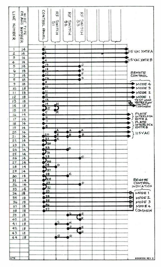
Figure 44. Control Panel MI-561767, Wire Chart
