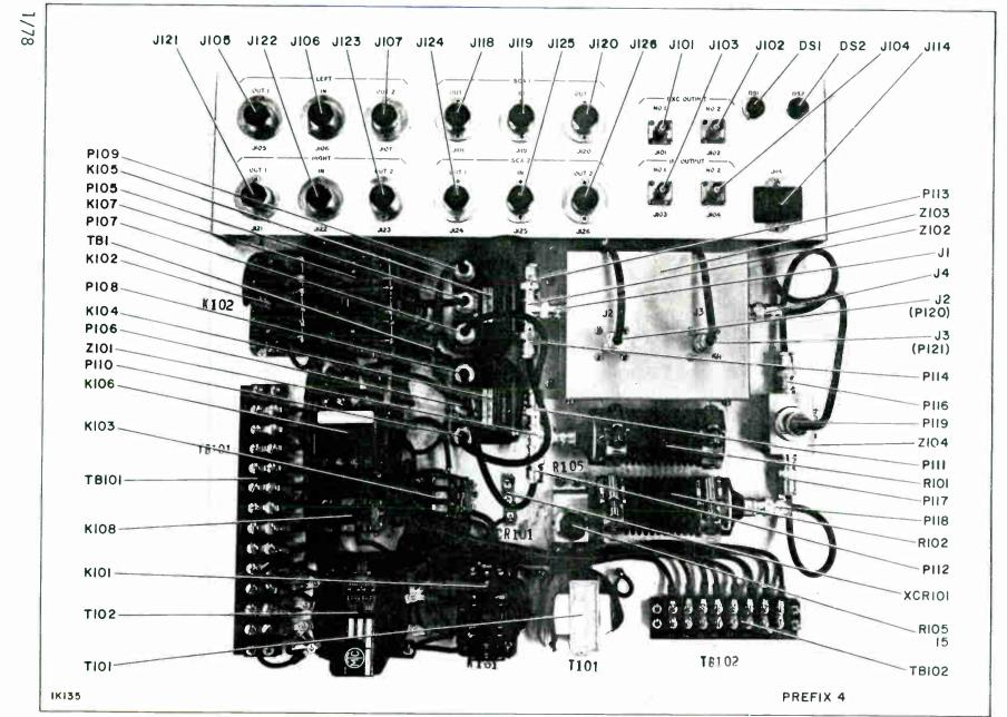
Figure 15. Exciter Switching Relay Panel MI-560700 Item 2, Rear View (Prefix 4)
