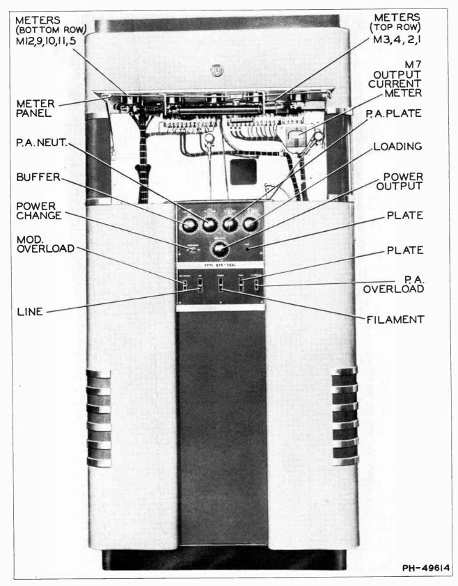
Figure 3—Transmitter (Front View, Meter Panel Open)
