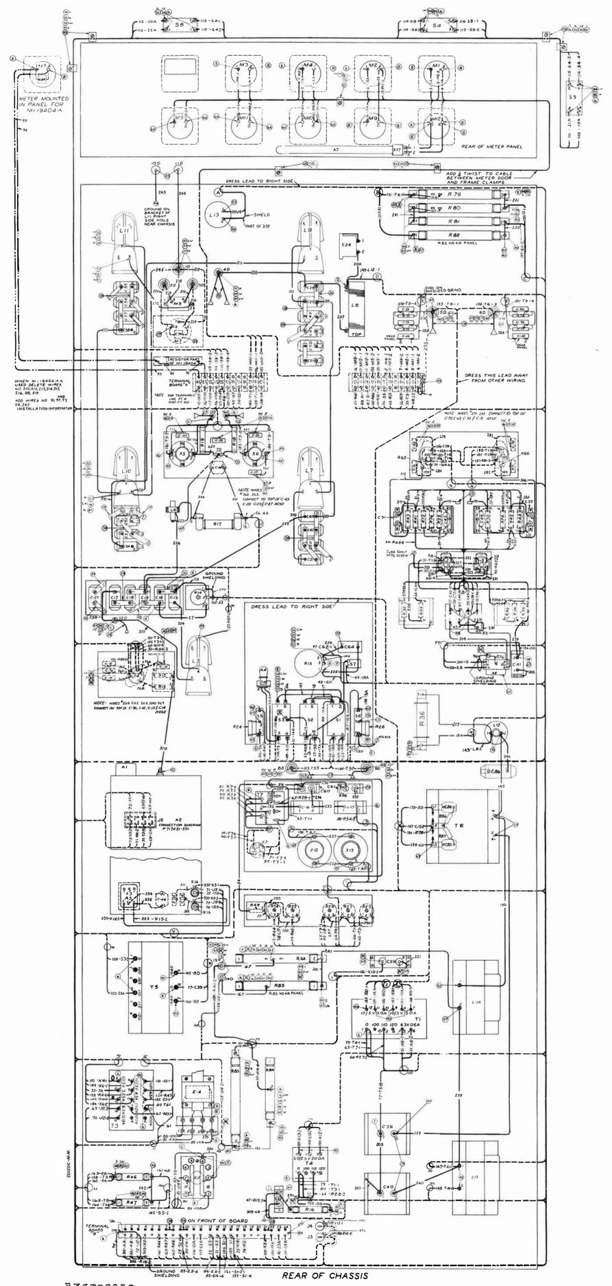
Coding at end of wires indicates wire number and destination of wire respectively. Where only one number is given, wire number is in-tended. A letter preceding a number, as (T2), indicates an electrical item. A number followed by a letter, as (25B), indicates a terminal number. Numbers in balloons are for manufacturing purposes only.
