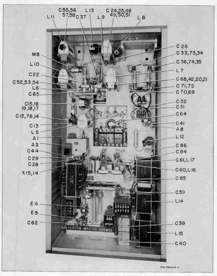
Figure 4—Transmitter Chassis (Rear View)
