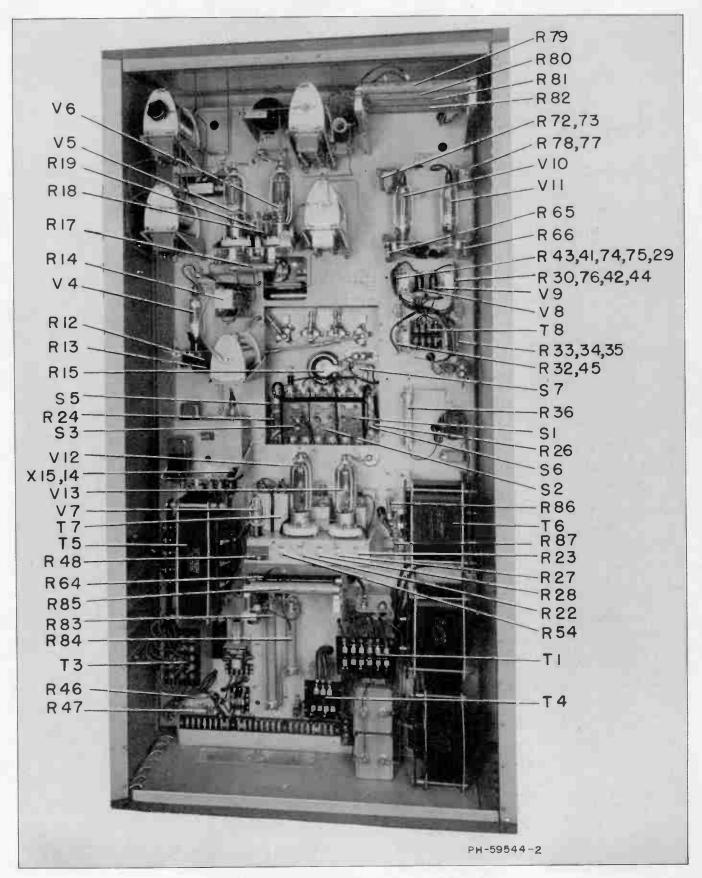
Figure 5—Transmitter Chassis (Rear View)
