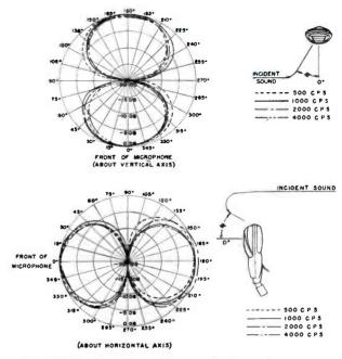
Directional Characteristics of the SK-46 Velocity Microphone.
