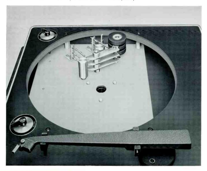
The turntable platter is a sturdy 14-pound aluminum casting. It and the spindle assembly are held in the main support casting in oilite bushings and the thrust is supported by a single ball at the bottom end of the spindle. The drive motor is mounted on a separate plate and supported by vibration mounts to eliminate rumble. All posts and shafts which provide bearings for cams and arms are assembled to a common plate to insure proper alignment.
