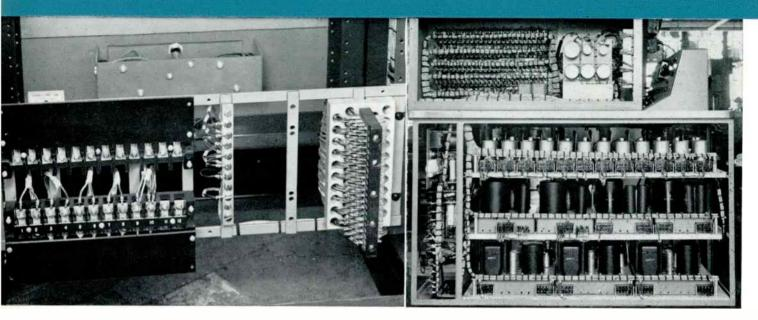
Fig. 1. Photo of terminals at bottom of rack. Power terminals are at left, ground buss in center and audio terminals at right.
