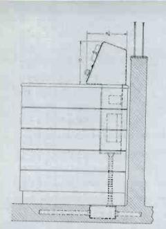
This cross-section view shows how the console at right was designed to permit some components to be mounted below the desk top. This results in small turret size and provides maximum visibility into the studio.
