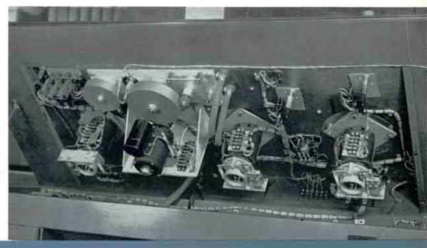
The entire motor board may be raised by means of a hinged panel to make control mechanism and wiring accessible.
