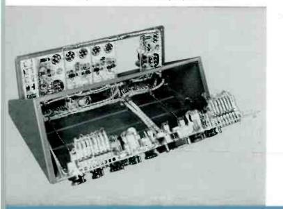
mounting frame is pivoted to provide easy access to the wiring for service.
