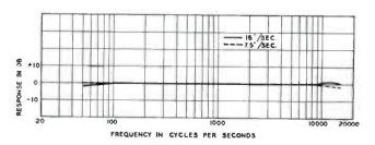
Typical response curve of RT-11B or RT-12C Tape Recorder.
