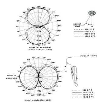
Directional Characteristics of the SK-35 Velocity Microphone.
