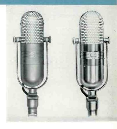
ment by positioning of a shutter to secure various areas of opening. The moving element is a thin corrugated metallic ribbon clamped at the ends and suspended in the air gap of a magnetic circuit consisting of an Alnico V permanent magnet and pole pieces. One side of the ribbon is open and the other is connected by means of a tube to a folded acoustically damped pipe contained in the center section of the microphone.
