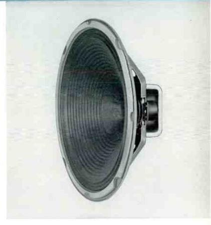
has the corrugated cone feature, which, by introducing just enough additional compliances, smooths and improves the frequency response characteristic. External metal parts of the MI-12418-B speaker are finished in umber gray metalustre. The speaker comes equipped with a matching transformer in place and wired to the speaker from the 6 ohm tap. Transformer impedances are 625, 1250, 2500, and 5000 ohms.
