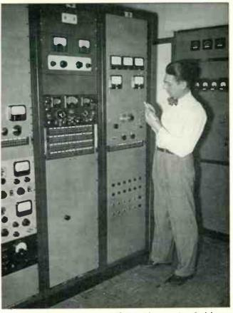
Engineer checks current ratios and phase at phase monitor. Push-button controls for remotely-controlled tuning motors and supervisory lights for the pattern-change relays are shown.
