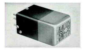
quartz plate and the top electrode is variable, and operable by rotation of a specially designed shaft provided with a screw-driver slot to facilitate adjustment under actual operating conditions. As the air-gap is varied to change the operating frequency, the crystal activity is also slightly affected. The recommended usable range of this variation in frequency is in terms of a crystal activity variation not exceeding 10% from the maximum.
