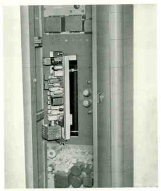
Hinged construction of the Exciter unit is a service and maintenance feature of new RCA STL equipment.
