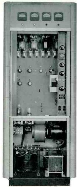
Front view of BTA-1M 1 KW AM Transmitter with horizontal sliding door fully opened and lower front panel removed. Overall simplicity of component arrangement is apparent.
