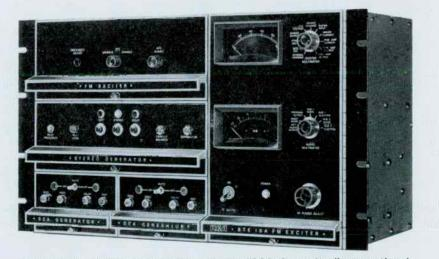
Exciter unit. "Stereo Generator" and two "SCA Generators" are optional. Note dual meters, one for dc parameters, one for audio measurements.
