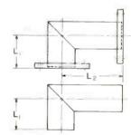
Flanged elbow uses swivel flanges and includes inner-conductor connector, O-ring gasket, six bolts, nuts, lockwashers. Unflanged elbow includes inner-conductor connector only.
