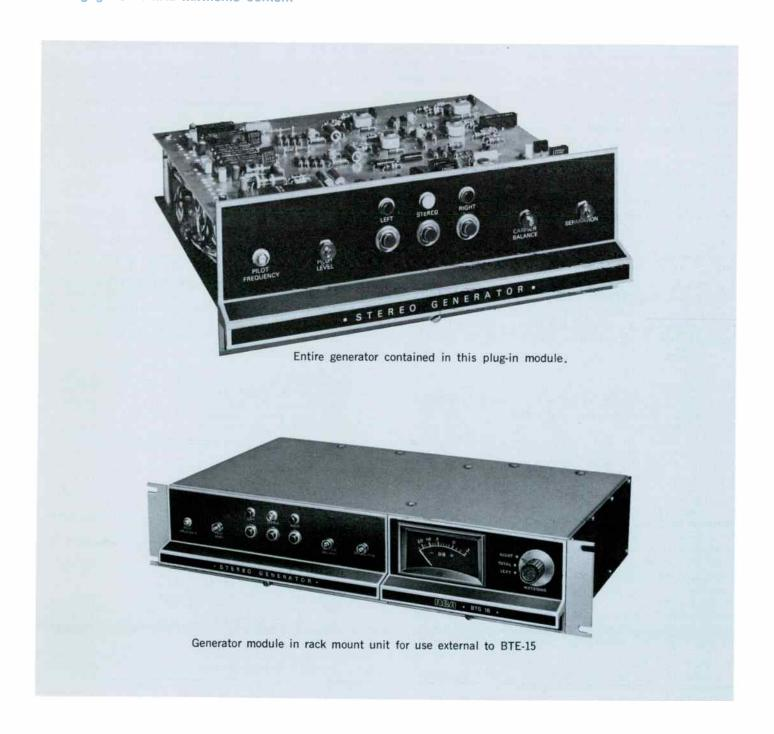
The BTS-1B Stereo Generator is a plugin module for the Type BTE-15A FM Exciter System. However, it is offered separately in a self-powered rack-mount assembly for use with RCA exciters and transmitters of earlier design. The selfpowered generator is also useful to form a composite stereo signal for an STL system. (See Ordering Information, below.)
