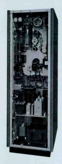
Unimpeded rear access to the transmitter is afforded by the full length door and the well laid out, vertical construction. Power supply components at bottom; r-f components at top.
