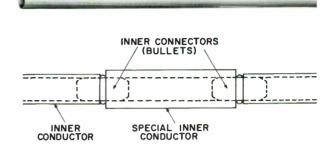
Oversize inner-conductor tube for splicing MI-19113C line when cut at point other than midway between insulators. Each splice requires two MI-19113C-11 inner-conductor connectors. (Not supplied, see below.)
