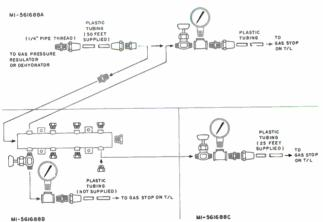
There are three gassing system kits: an "A" kit which is basic to Kit "B" which, in turn, is basic to Kit "C".
