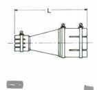
Reduces 31/8-inch (MI-19113C or MI-19313) unflanged line to mate with 1%-inch (MI-19112) unflanged line.
