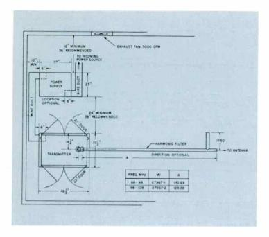
Space-saving floor plan of the BTF-5E1. The separate, unitized power supply may be installed in the basement, attic, closet, or other convenient place. (Wire duct and fan shown are not furnished.)
