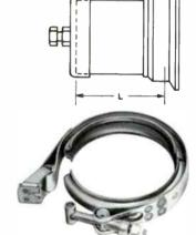
Caps male end of line temporarily to prevent moisture entry. Fitted for gassing and bleeding.
