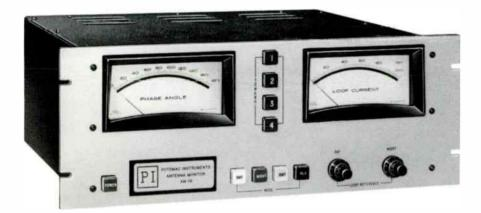
The PM-19 system uses the AM-19 (204) Antenna Monitor as a base and adds to it a PMA-19 Precision Monitor Adapter. The combination of the two units increases resolution and repeatability to one-tenth degree for phase angle and one-tenth percent for current deviation measurements. The system reads out loop current ratios directly. The system provides both analog and digital readout of all three parameters.
