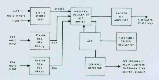
Simplified block diagram, Type BTE-15 Exciter equipped for stereo and two SCA subchannels.
