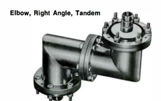
All flanges swivel. Includes one O-ring gasket, two captive connectors, twelve bolts, nuts, lockwashers.
