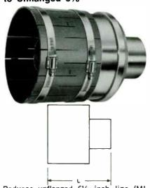
Reduces unflanged 6½ inch line (MI-561579) to unflanged 3½ inch line (MI-27791K). Requires coupling MI-27791K-4A (not supplied). Coupling for 6½ inch end included with two clamps.
