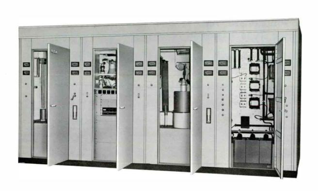
Compact in-line construction of BTA-50J showing left to right, left hand power amplifier, exciter, right hand power amplifier, and rectifier-control cubicle.
