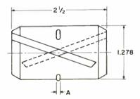
For joining inner conductors of MI-19313 transmission line sections.
