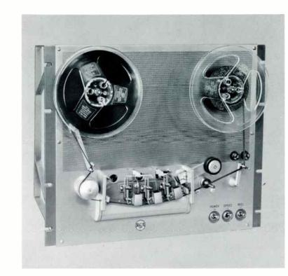
RT-21B Tape Transport with cover removed to reveal magnetic heads. Note cut-out provision on left for optional fourth head kit for playing pre-recorded stereo tapes.
