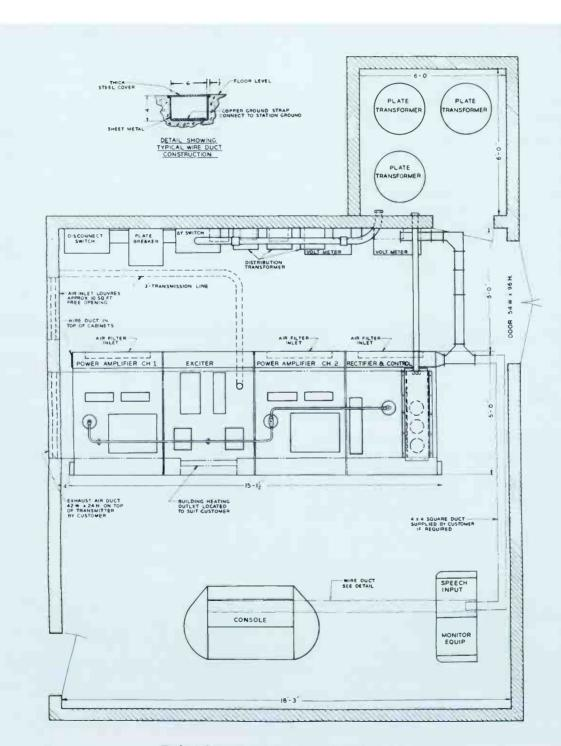
Typical floor plan for the BTA-50H1 Transmitter.
