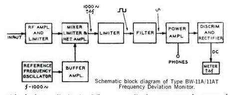
quick check on all circuits. When the monitor is working normally and this button is pressed, the meter deflection increases by approximately 5 Hz. A change appreciably different from 5 Hz indicates a defective circuit.
