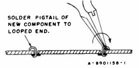
Figure 20—Replacement of Components in Printed Circuits
