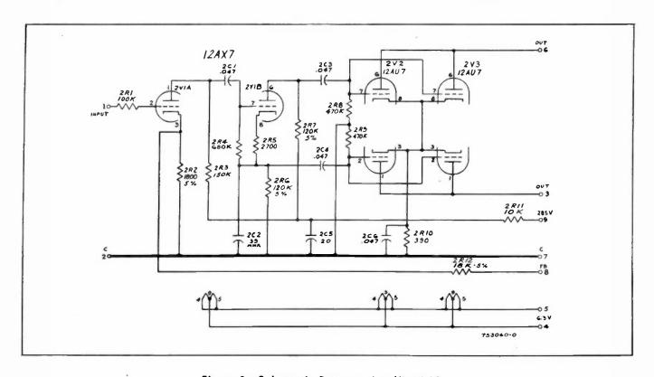
Figure 8—Schematic Program Amplfier 5AR8
