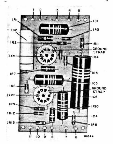
Figure 3—Preamplifier (5AR1—5AR3) Printed Circuit
