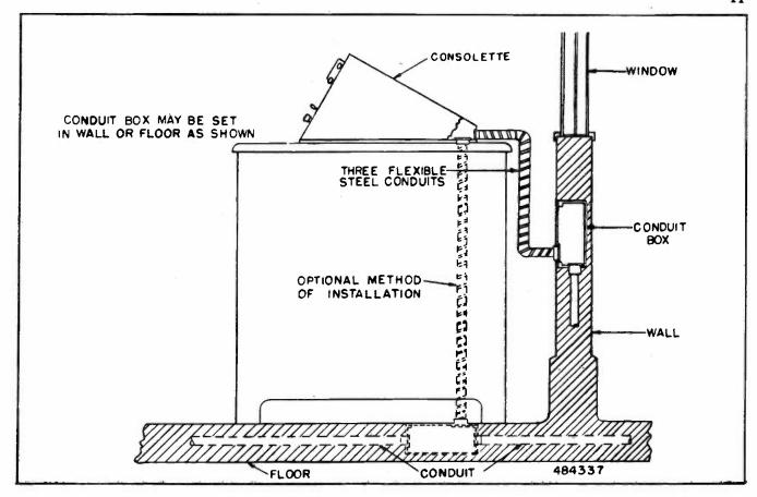
Figure 15—Typical Cable Installation
