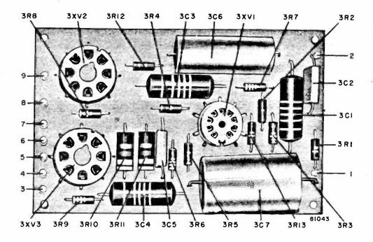
Figure 9-Monitor Amplifier 5AR9 Printed Circuit Board
