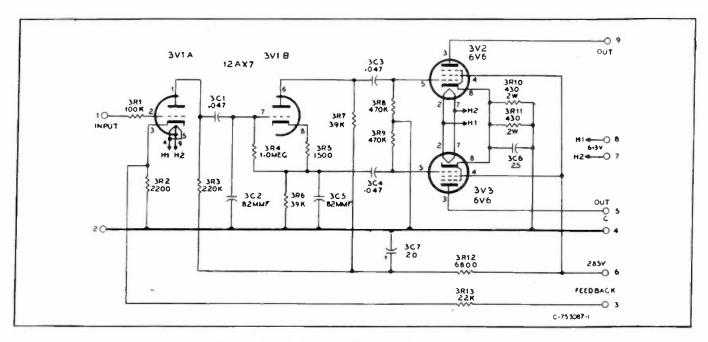
Figure 10—Schematic Monitor Amplifier 5AR9
