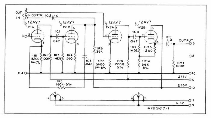
Figure 6—Schematic Diagram for Preamplifier (5AR4—5AR7)
