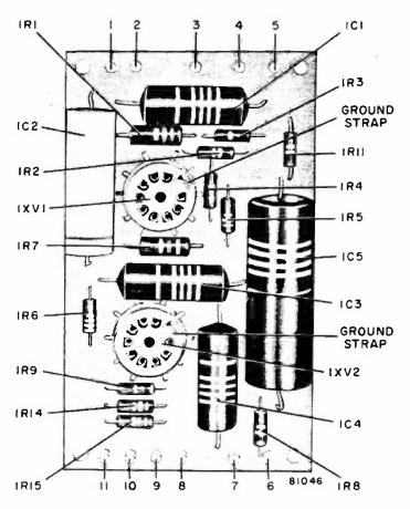
Figure 5—Preamplifier (5AR4—5AR7) Printed Circuit
