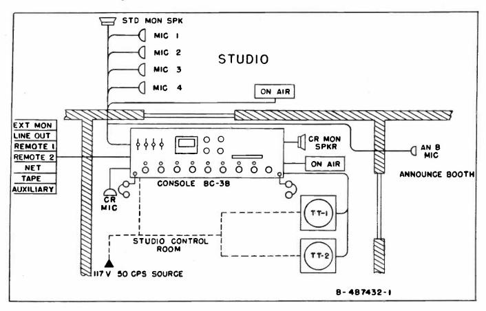
Figure 17—Typical Installation for One Studio
