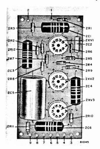
Figure 7—Program Amplifier 5AR8 Printed Circuit
