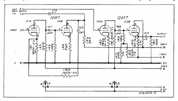
Figure 4—Schematic Diagram for Preamplifier (5AR1—5AR3)
