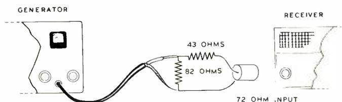
For a device with  $300\ \Omega$  input, a similar pad may be made up with values of  $56\ \Omega$  between center conductor and shield, and  $270\ \Omega$  between center conductor and the device under test.
