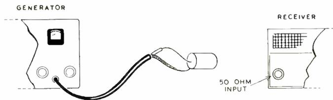
In the case of a device with  $72 \Omega$  input, a simple "pad" may be constructed out of two small composition (NOT wirewound) resistors:  $82 \Omega$  between center conductor and shield, and  $43 \Omega$  between center conductor and the device under test. This pad introduces a loss of 4 db and thus the voltage applied to the device is only 62% of the value indicated by the generator.
