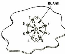
NUMBERING ON 7-PIN TUBE SOCKET
