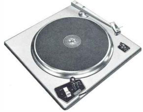
MODEL CB-88: Complete ready to operate 12" turntable assembly. Includes CB-77 12" chassis, M-6244 transistor preamplifier, dual viscous damped Gray arm, twin flip-over 1 mil. and 21/2 mil. reluctance cartridge with your choice of sapphire or diamond styli, 2-position equalizer to NAB-RIAA and high frequency roll off curves and self-contained power supply (part of preamplifier).
