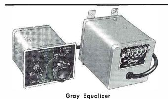
Four-position equalizer for use with any low impedance pick-up cartridge and provides these curves: (1) Flat, (2) Intermediate, (3) Standard, (4) Roll off. Output impedance 150/250 ohms. Supplied as illustrated with etched dial plate and knob. Used with low impedance cartridges only.
