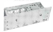
Operates with any approved FM frequency/modulation monitor where the signal is taken off the air and monitor is at studio. Amplifier supplied fixed tuned to your frequency. Power supply is not supplied. Requires 300 volts DC at 100 MA and 6.3 volts AC at 3 amperes.
