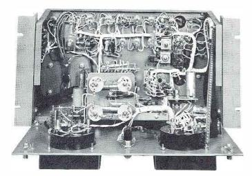
Front Panel Hinges Down for Complete Accessibility.
