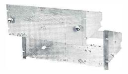
Used for rack or multiple mounting of plug-in units. Requires only 7" x 19" rack space. Front is ventilated by top half being perforated and is instantly removable to allow removing amplifiers from the front, or making gain adjustments. The BA-20 or BA-21 bases with receptacle, listed below, fasten to the bottom of the panel and shelf assembly. Depth is 133%". Finish medium gloss gray. Weight 10 lbs.
