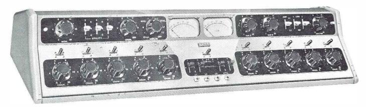
The Gates Model TV-10 audio console is one of the most outstanding consoles on the market for television and recording studios. This is a ten channel speech input system specifically designed for audio control in large television productions. For recording, it provides the input channels so necessary for the demands of professional recording studios.
