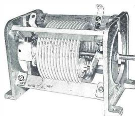
Used in both Gates and many other makes of transmitters and phasing equipment. Variable coils have cast aluminum end bells with double gripping bearing wheels. All types are micalex insulated and silver plated and have the highest possible "Q's".
