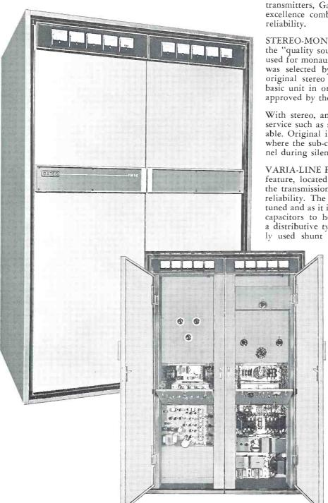
In the new FM-5C 5000 watt and FM-7.5B 7500 watt transmitters, Gates offers the very finest in technical excellence combined with styling, serviceability and reliability.
