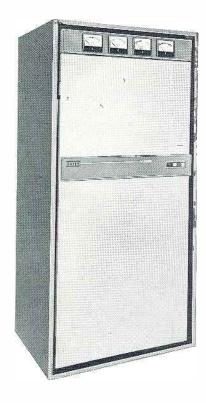
The BC-500G, 500 watt AM transmitter is essentially the same as the BC-1G, 1000 watt model. It consists of 4 RF stages with provision for two vacuum type crystal units of extreme stability. Following the 807 drivers, a simple type 833A final amplifier feeds a full "T" network for maximum harmonic attenuation. The final amplifier and "T" network are tuned by variable edgewise wound coils for exact tuning, loading and reliability.
