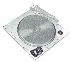
CB-510 complete operating transcription turntable includes CB-500 low noise chassis with synchronous motor, GRAY 208-S/G viscous damped pickup arm, twin flip-over 1 mil and 3 mil reluctance cartridge, 2-position variable equalizer to NAB/RIAA and high frequency roll off curves and M-6244 transistorized preamplifier with self-contained power supply. Output: 150 or 600 ohms adjustable from —22 dbm to —12 dbm, 12 MV input.
