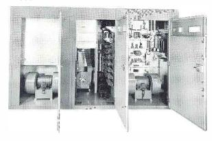
Rear view showing internal blowers and RF shielding. Where desired, one 10 HP belt driven blower is supplied for installation external to the transmitter and for any type of discharge arrangement.
