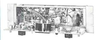
Front panel drops down for complete inner servicing. Big advantage of this type of construction is ability to keep important inner workings clean by means of bellows or small suction type cleaner.
