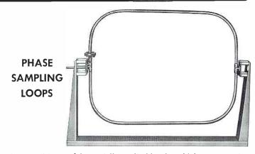
M-3283: This model especially applicable where high current ratios are to be sampled. May be rotated so that phase monitor amplitude values are nearly equal. Electrostatically shielded and insulated from tower. May be used with or without isolation coil at base of tower. Coil is single loop of  $\frac{7}{8}$  coaxial cable, heavily insulated from base frame. Matches either 50 or 70 ohm line. Size: 48" wide, 32" high.
