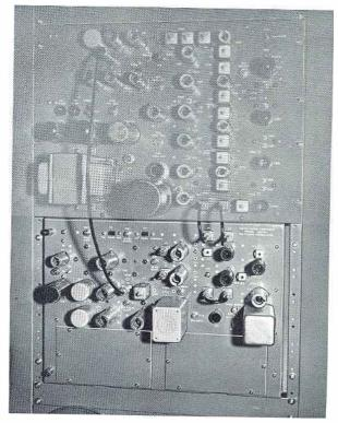
Top Unit — Gates "Cascade" FM Exciter. Lower Unit — M-6146 Stereo Generator.
