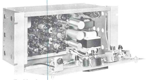
Hinged-down front panel permits complete front accessibility of components and inner servicing adjustments. Printed wiring by the Gates solid adhesion process assures uniformity and ease in both cleaning and circuit analysis. "Level Devil" finish is a medium gloss gray over a heavy prime coat. Design is for continuous duty.
