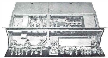
The regulated power supply protects the console amplifiers from variations due to line and load regulation. In addition, the power supply ripple is reduced to the point of nonexistence to assure uniformly low noise in all of the console circuits. The power supply is also short-circuit protected to prevent damage to any of the transistors in either the power supply or amplifiers from a momentary or sustained short in any of the circuits.
