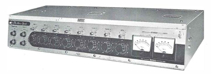
The Gates Stereo Yard is a completely new compact 8 channel console designed for full stereophonic operation. It provides the broadcaster with three full stereo microphone channels, utilizing six microphone preamplifiers and five high level stereo mixing channels.
