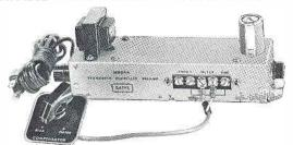
A single channel monophonic preamplifier designed for use in broadcasting, recording, and general sound requirements where low distortion and exacting frequency response characteristics are demanded. Features self-contained power supply and transformer output.
