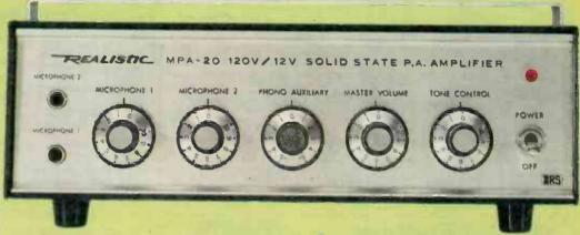
Realistic\* MPA-20. Level controls for Mike-1 and Mike-2, phono/aux. Tone and master volume controls for controlling all inputs simultaneously. Separate on/off switch. Pilot light. Outputs: 4, 8, 16 ohm speakers; 25 and 70-volt line. Power: 20 watts RMS at 8 ohms. Response: 200-10,000 Hz at full power. 41/2x101/2x71/2" metal case. Carry handle/mobile bracket, power cords for 12 VDC and 120 VAC. U.L. listed. 32-2020
