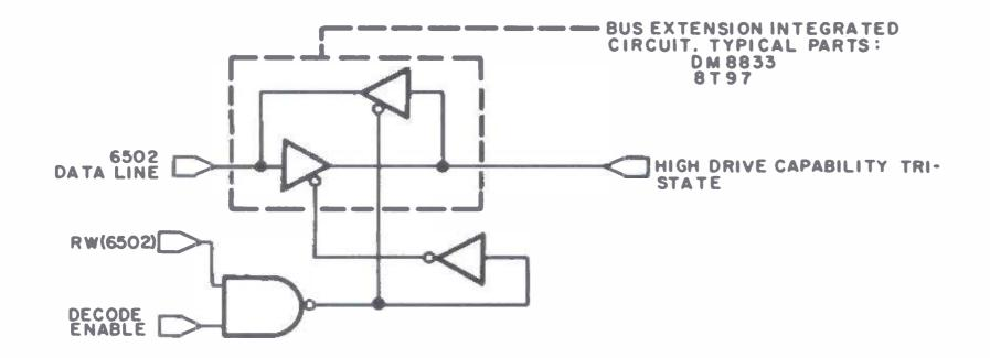
Figure 8: Adding a gate to the bus extension control resolves a potential conflict through the use of a decode enable signal which is high if external memory is referenced, low if memory on the KIM-1 board is referenced.
