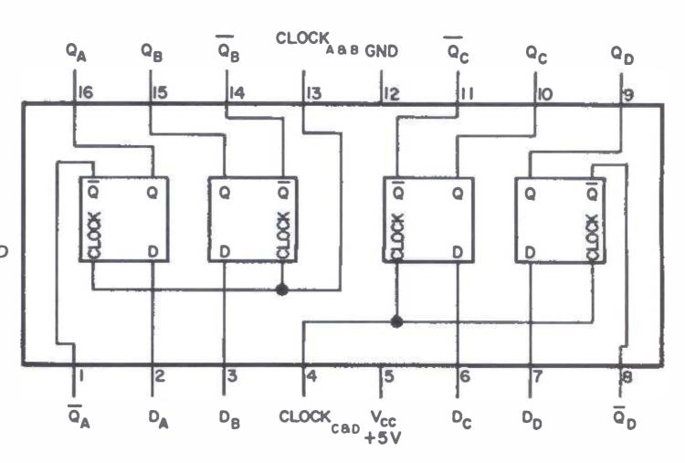
Fig. 16. Pinout of the 7475 latch (or register) circuits. (Top view)
