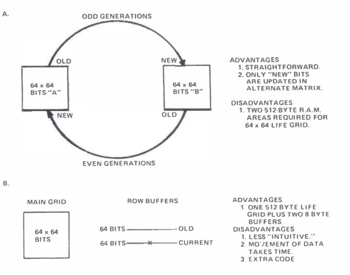
main grid copy. Two 64 bit rows must be maintained the last previous row and the current row - as 8 byte copies. These copies contain information prior to updating in the row by row scan down the matrix. The main advantage is a saving of data areas (partially offset by more complicated software). The main disadvantages are its less "intuitive" nature, the extra time required to make data copies, and a slightly larger program.
