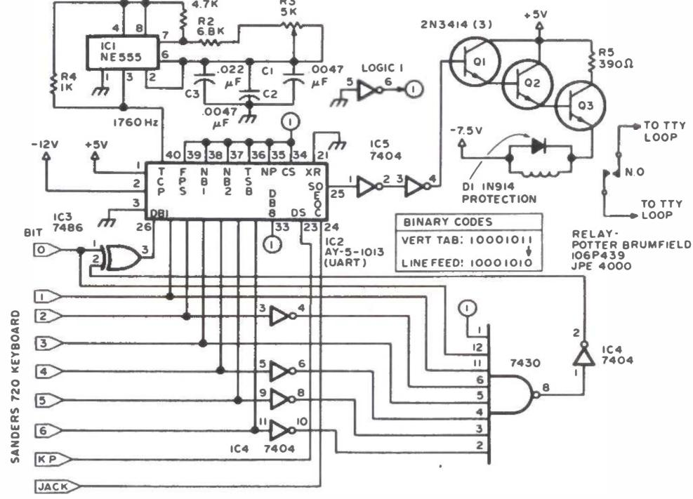
Figure 1: Using a UART and special case logic to convert and serialize the output of a keyboard for a 60 mA current loop.
