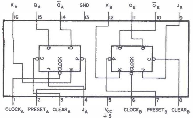
Fig. 10. Pinout of the 7476 IC, a dual flip flop similar to the 7473 but having both PRESET and CLEAR. (Top view )
