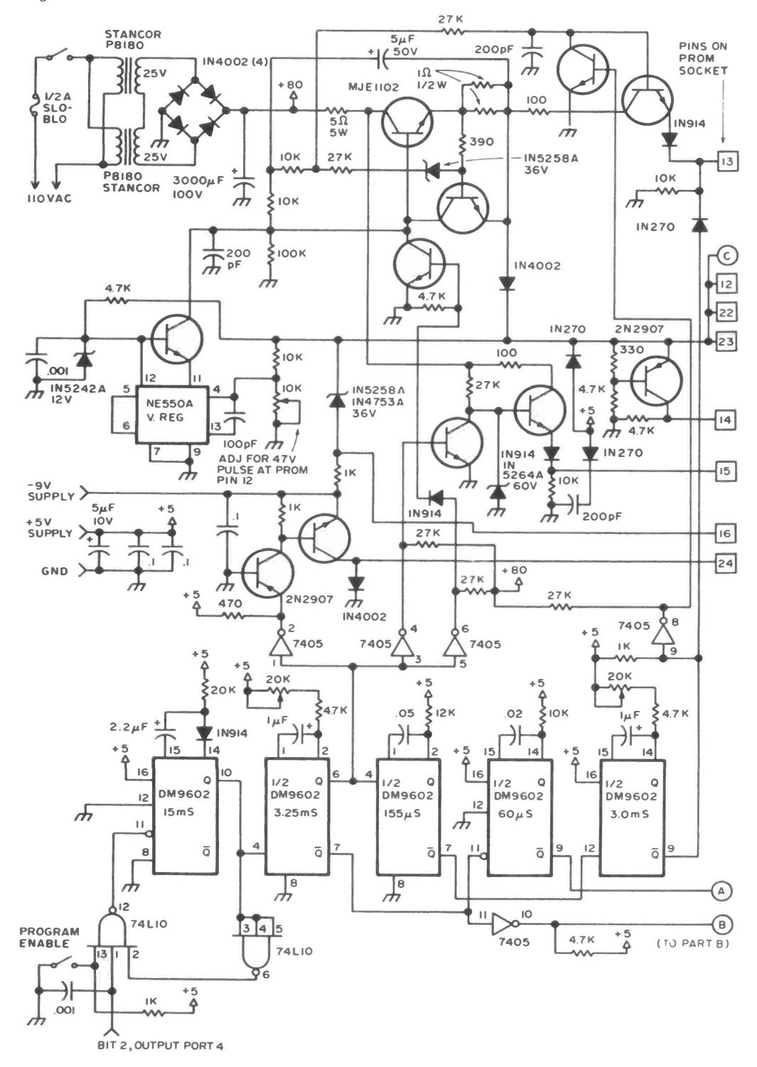
Figures 3A and 3B: Computer controlled PROM programmer for stored charge PROMs. Unless otherwise noted, transistors are MPS-A06 or 2N3722 or equivalent. Pin 14 of ICs to 5 V, pin 7 to ground.
