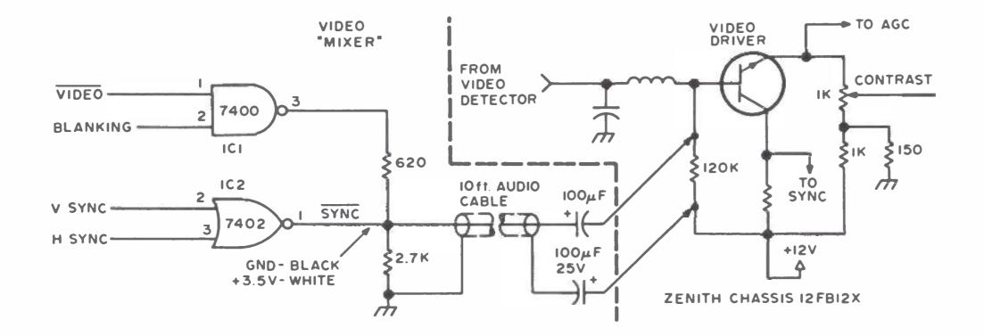
Figure 1: The "Ignorance Is Bliss" Television Drive Circuit. The components to the left of the dashed line were added as part of the interface. The components to the right of the dashed line are part of the Zenith 12FB12X chassis which was used for the television display.
