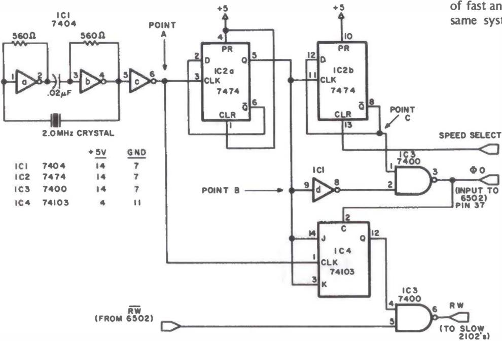
Figure 1: A circuit which creates an alternative slow clock cycle for the 6502 processor on the KIM-1 board under control of a "SPEED SELECT" line generated by slow memories. SPEED SELECT = 0 for fast cycles, SPEED SELECT = 1 for slow cycles. This circuit requires a 2.0 MHz crystal.
