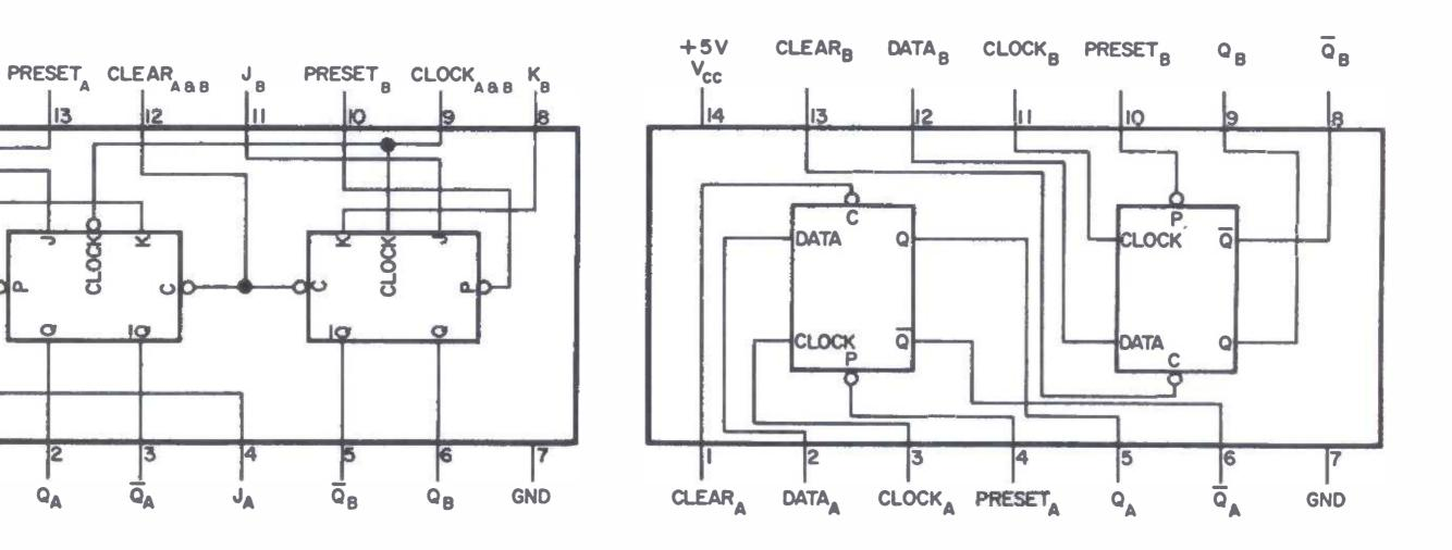
Fig. 11. And still another combination - the pinout of the 74H78 has 14 pins with common CLEAR and CLOCK, and separate PRESET pins.
