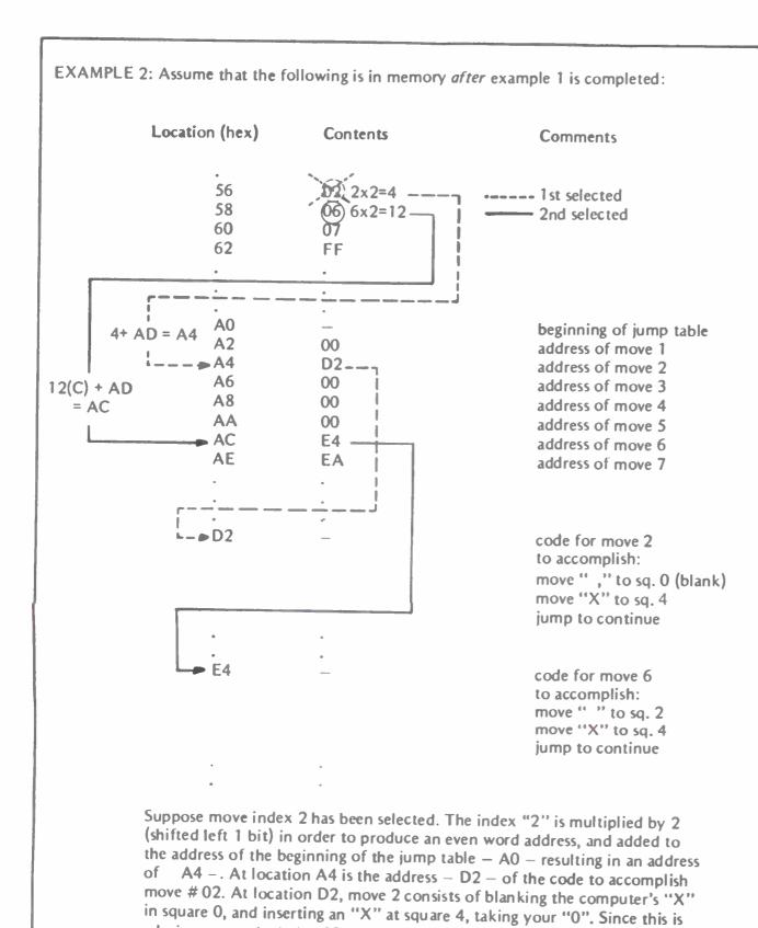
a losing move, the index 02 will be made null (replacement by 00 is good for error checking), and move 06 will be accomplished in the same manner
