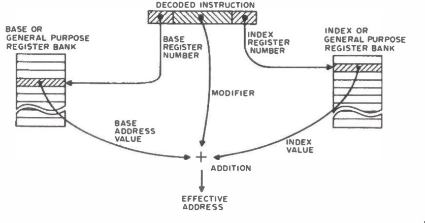
Figure 5: Combining Two Index Registers. A more general address calculation uses one register as a base register, a second register as an index register, and a modifier. The effective address is then the sum of the values found in the two registers and the value of the modifier. The order of calculation and detailed significance of the registers depends upon the processor design which uses this type of address calculation.
