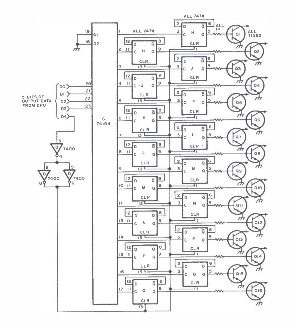
Figure 1: This is all you'll need to build if you already have a parallel output port you can use to control the interface card. If not, lines D0 through D4 should be joined with the corresponding points in figure 2. Transistors Q1 through Q16 can be any economical NPN with reasonable Beta. Due to varying configurations (you may not want to build up all 16 channels or use different transistors), I suggest the card be wirewrapped.
