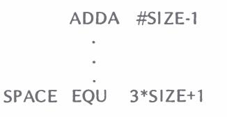
which would specify (for SIZE=25) that 24 should be added to the A accumulator, and that SPACE should have the constant value 76 wherever it appears in the program.
