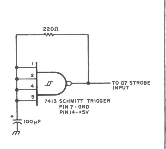
A test setup for manual verification of the display. The Schmitt trigger integrated circuit, a 7413 NAND function, has an RC feedback network to cause oscillations. This logic oscillator is used to drive the strobe input continuously, so that memory will be filled with a constant character pattern if that pattern's ASCII code is presented on
