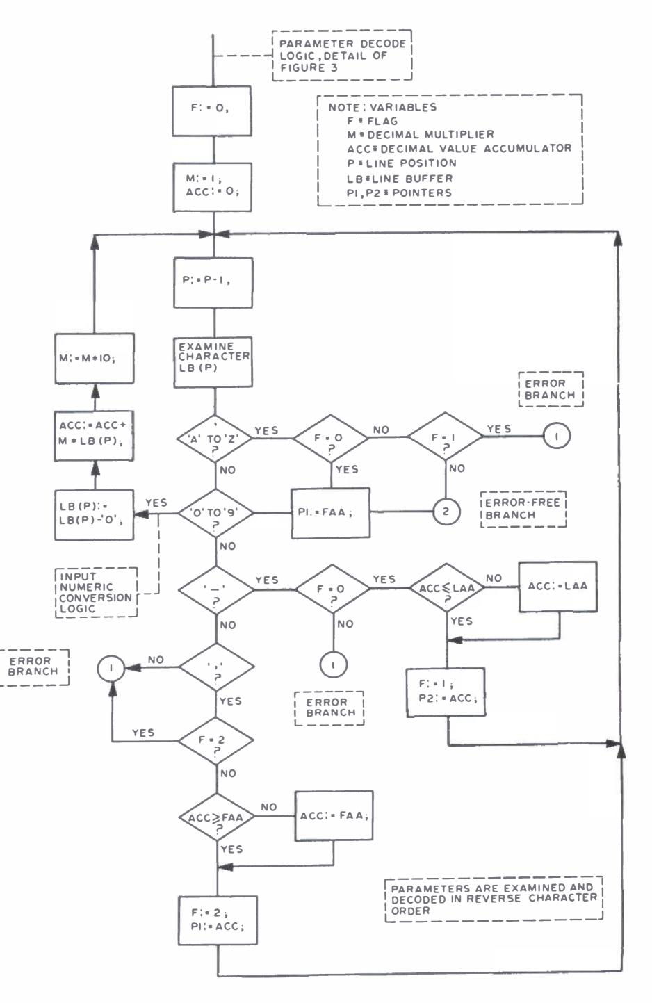
Figure 5: Parameter Decoding Logic Details. Figure 3 contains a box labelled Decode Command Line and a conditional test labelled Errors, with a note referencing figure 5. This figure contains the details of the logic needed to decode a command line into two parameters and a command. There are two possible exits from this logic. An error exit to terminal (1) occurs if an error is detected; an error free exit to terminal (2) occurs if no errors are detected.
