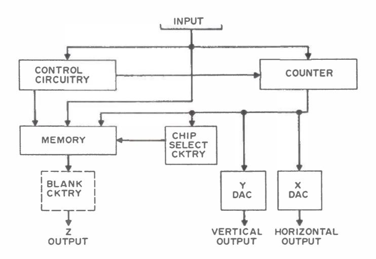
organized according to the computer's instructions. During the scan cycle, the digital dot pattern is converted to analog waveforms which reproduce the image on an oscilloscope screen. The graphic interface stores the dot pattern within its own internal refresh memory. Therefore, once the pattern has been generated and loaded into the graphic interface memory, the computer is left free to execute other programs.
