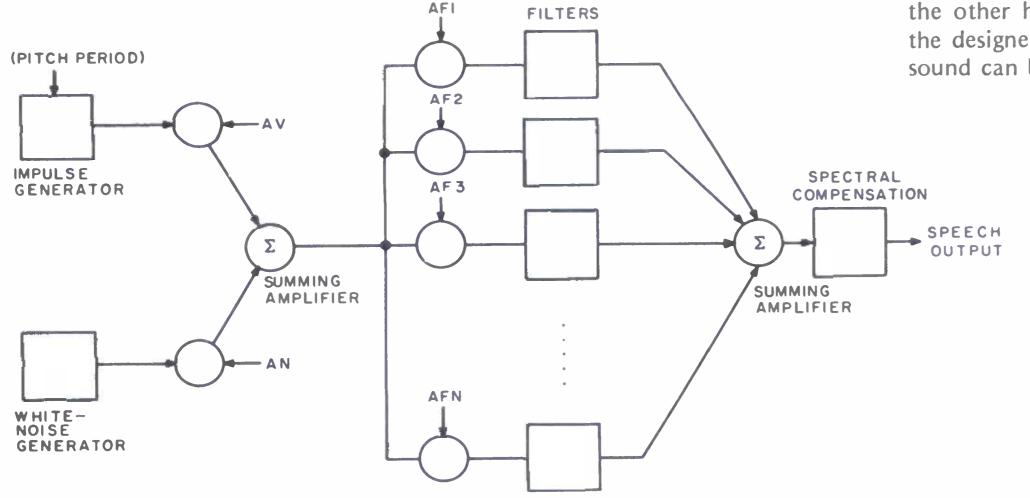
Figure 2: The parallel analog speech synthesizer in block diagram form.
