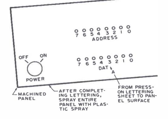
A word of caution; let the spray dry thoroughly before mounting the components. Secondly, on each spraying put down only a light coat. Otherwise the letters will tend to move (float?) a little out of place. Also be careful when mounting components onto the panel so that the lettering and/or the panel's surface is not scratched. The end result of lettering and care will be a very good looking piece of equipment.
