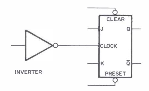
Fig. 4. Inverting the clock input converts rising edge-triggered operation into negative edgetriggered operation and vice versa.
