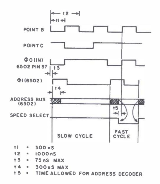
Figure 2: Method 1 SPEED SELECT Discipline. In this method, fast cycles are the rule, slow cycles are the exception. Refer to figure 1 for points B and C. Invalid data on the address bus is indicated by the crosshatched areas.
