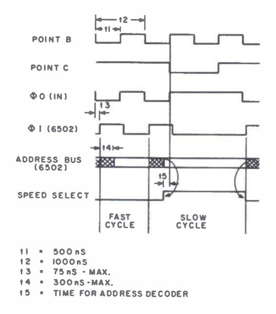
tained at 1.0  $\mu$ s for the fast memory access, while for the slower 2102s, the cycle is automatically stretched to 2.0  $\mu$ s.
