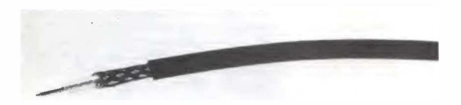
Photo 1: Coaxial cable consists of a central conductor, an outer conductive braid, and a protective coating. It is bulky and expensive, but it has good characteristics as a transmission line for data.
