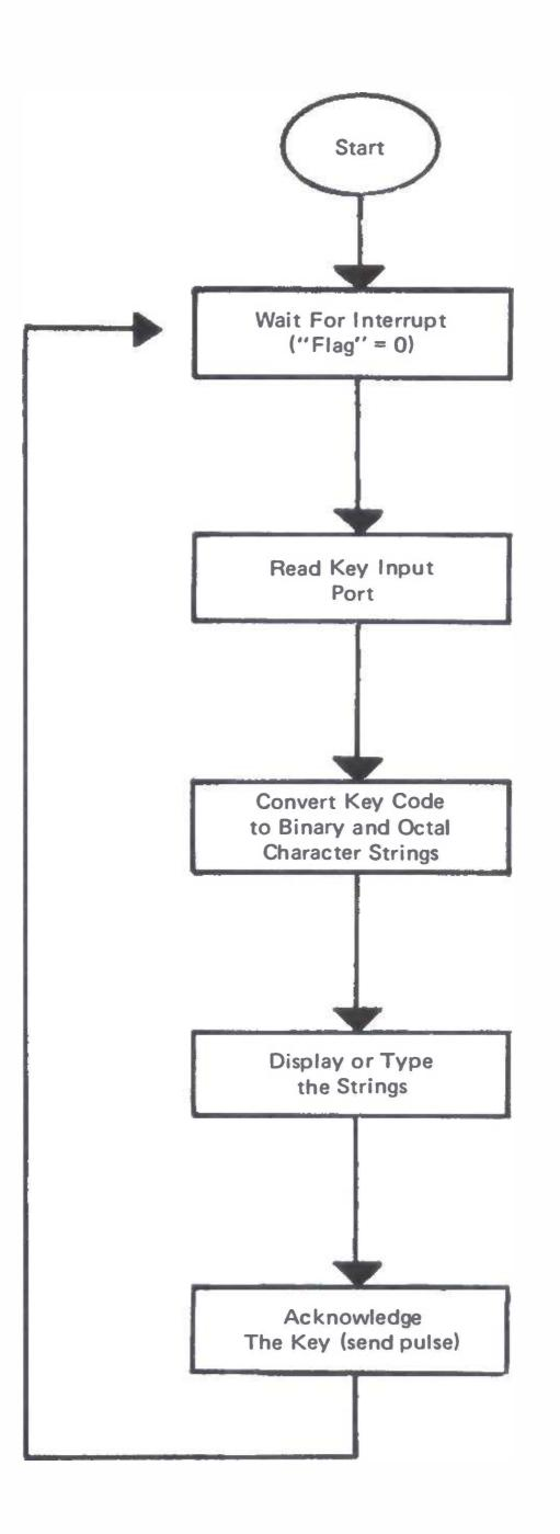
Fig. 6. Keyboard Test Program Flow Chart.
