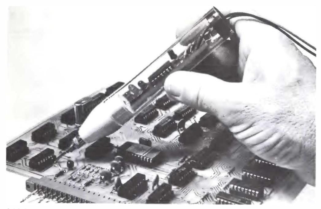
A logic clip is like 16 binary voltmeters in a neat little package.
