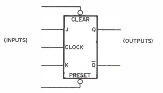
Fig. 1. The JK flip flop block diagram.
