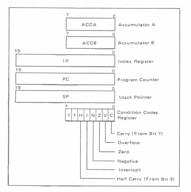
Fig. 2. The programmer's view of the 6800 CPU. This diagram, excerpted from the Motorola 6800 documentation, shows the various registers of the CPU including the processor's condition code register. Note the similarity to the MCS6501 in Fig. 3.
