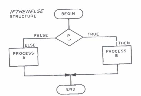
Figure 2: The IFTHEN-ELSE structure is a conditional test and two alternative SEQUENCE structures. The THEN alternative is executed if the condition, P, is found to be true. In this illustration, the THEN alternative is shown as a one step SE-QUENCE structure called B. The ELSE alternative is executed if the condition is found to be false. In this illustration, the ELSE alternative is shown as a one step SEQUENCE structure called A.
