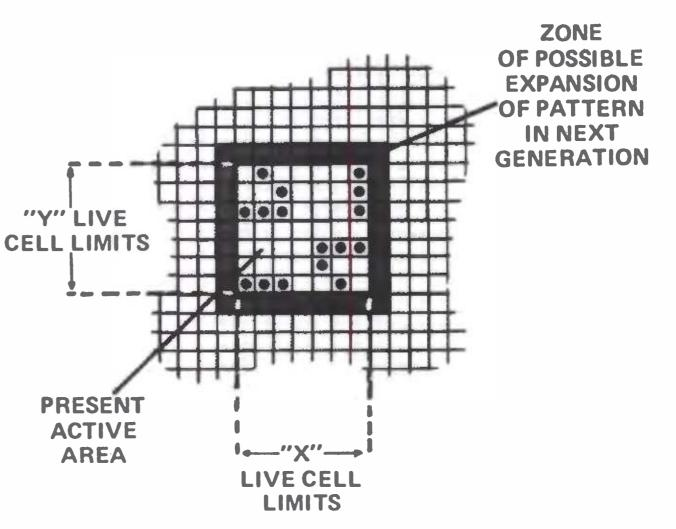
possible expansion. Thus in the case of the 64 by 64 matrix of LIFE points, this optimization for the pattern of Fig. 5 will limit the program to calculation of 81 new points versus the 4096 points which would be calculated if at least one cell was found at each of the minimum (0) and maximum (63) values of the X and Y The "facts of life" must be applied to each location in the grid to compute the next value - cell or no cell - of that location.
