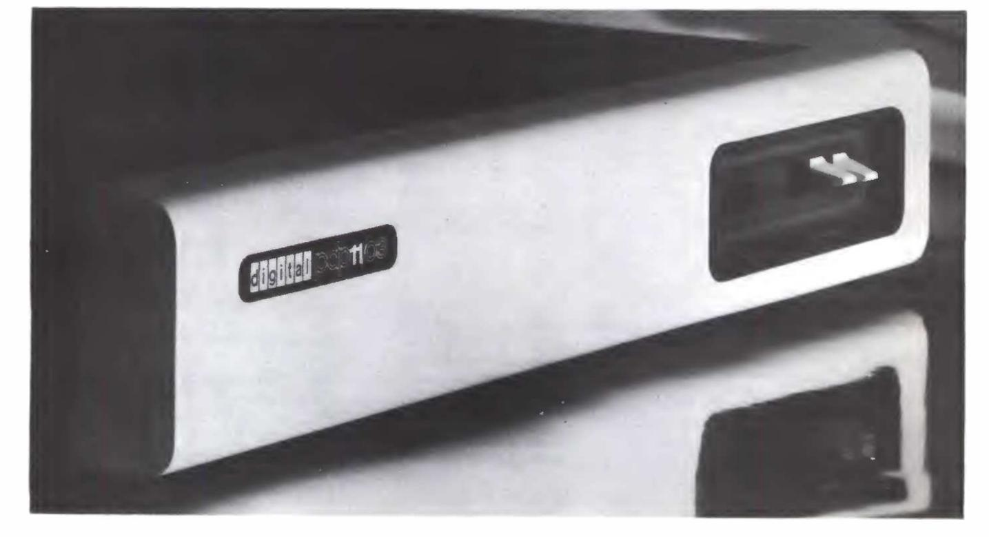
To accomplish this goal, the LSI-11 was designed to optimize system costs rather than component costs. A four-chip microprogrammed central processor was selected to emulate the PDP-11 instruction set, allowing the inclusion of automatic dynamic memory refresh without additional cost. The microprogrammed processor also makes feasible user microcode and an ASCII console which will be discussed later.
