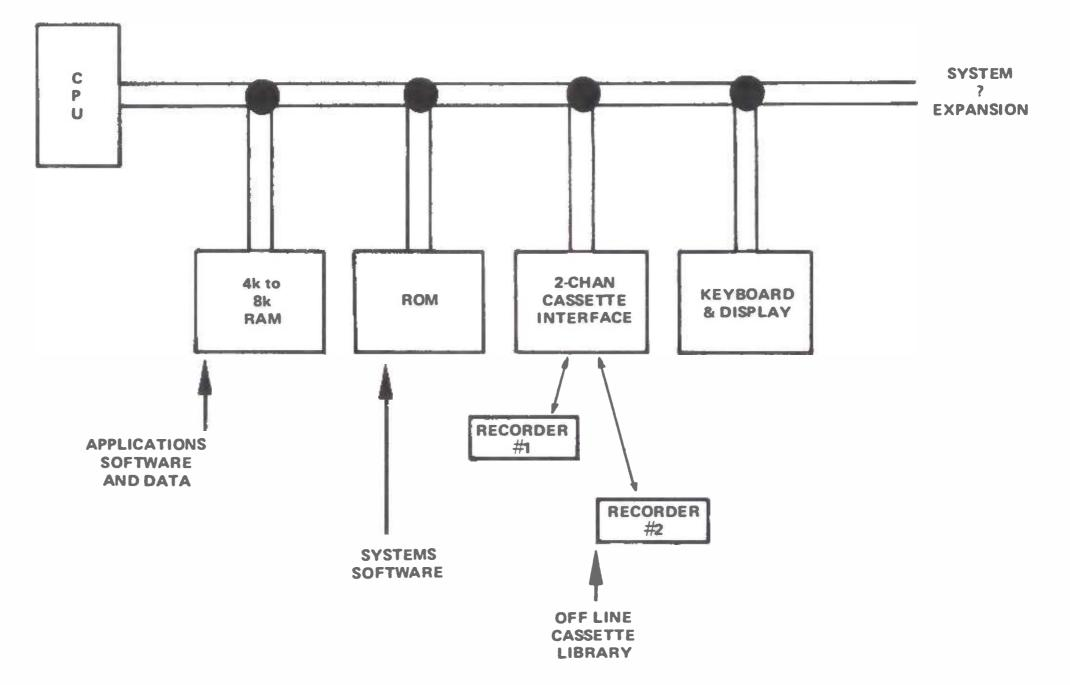
Fig. 1. The Complete Low Cost Computer System (circa September 1975). This diagram shows the major components of a typical low cost computer system — which should total up under \$1000 depending upon manufacturer and details of design. At the time this editorial is written, several kit manufacturers meet this functional benchmark at prices well under \$1000. As time goes on the improvements of mass production should drop the average price of such systems.
