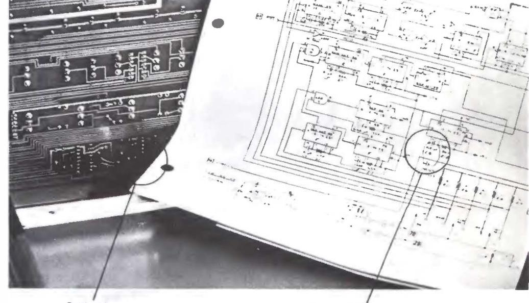
Solder the additional capacitor to the rear of the control panel board.
