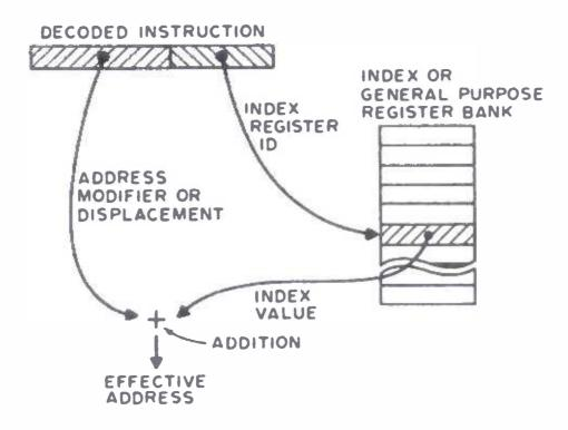
microprocessor designs, the index register is not large enough to contain a full base address. For instance, this occurs if the microprocessor uses a 16 bit address space and contains only an 8 bit index register. This case would require using the index register to contain a displacement with the base address becoming the instruction's modifier field.
