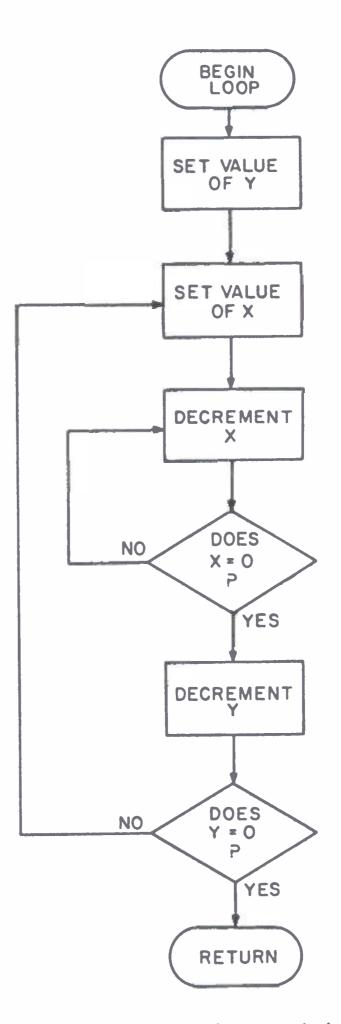
Fig. 2. Getting fancy. By nesting one timing loop within an outer loop, much longer delays can be obtained. Two parameters "x" and "y" are re-
