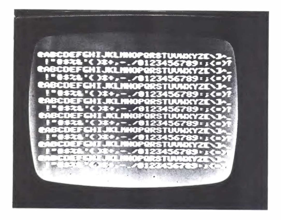
Photo 1: This is a test display pattern generated by connecting the low order outputs of the character and line counters to the character generator ROM's 6 input bits. The result presents every combination of the character set, so every character pattern is visible on the screen.
