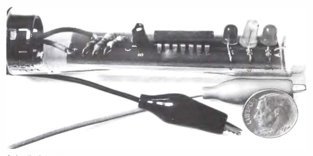
A detail of the Chesapeake Digital Devices logic probe board. The three LEDs are at the right in this picture, with the 74S00 IC in the center.
