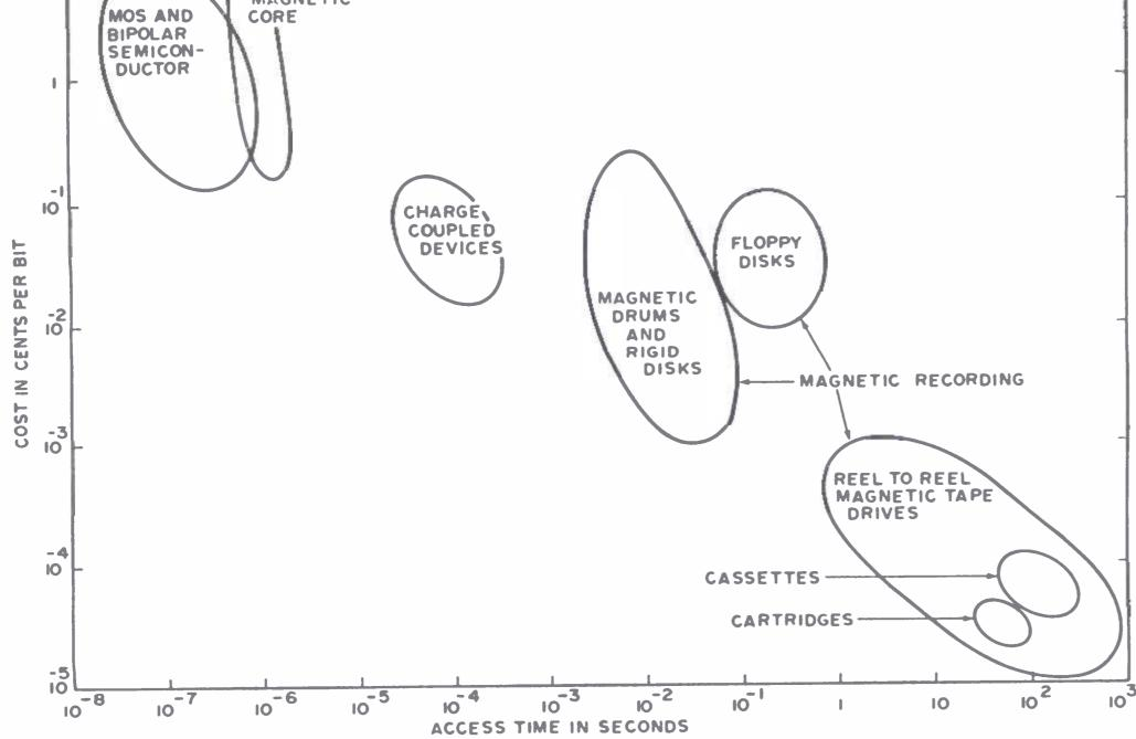
Figure 1: Digital computer memory hierarchy: cost as a function of access time.
