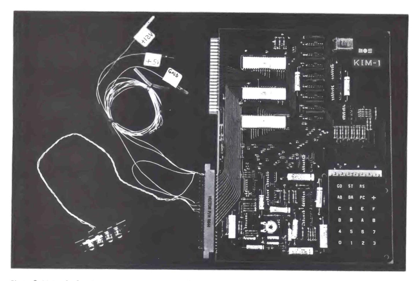
Photo 3: Wiring for Stand Alone Use. With due respect to the instructions in the KIM-1 user's manual, and addition of some mis-
