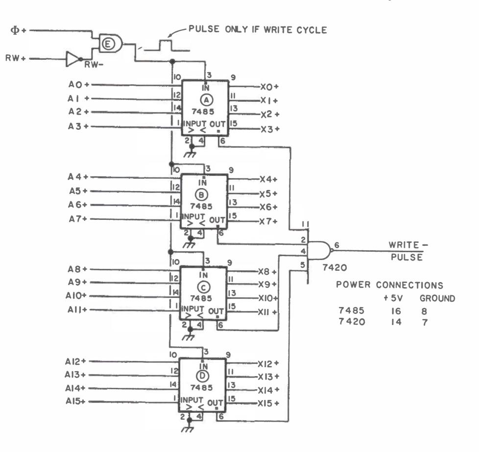
cascading input for equality is used to enable the comparison: the AND gate "E" detects a CPU write operation as the simultaneous occurrence of the clock  $\emptyset$ + and a low state of RW+.
