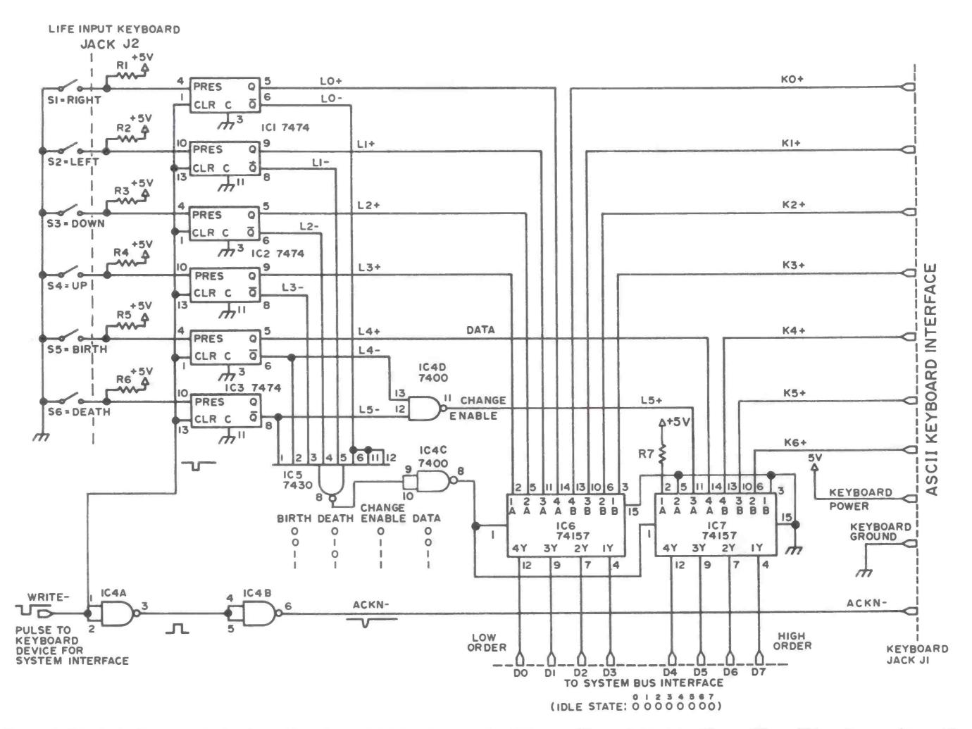
Figure 2: The logic diagram of a keyboard interface which implements the formats of figure 1. Resistors R1 to R7 are TTL pull up resistors. The value are not critical, and may range from 1 K0 to 10 K0, ¼ W.
