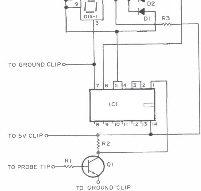
Fig. 2. Circuit diagram for the James logic probe kit.
