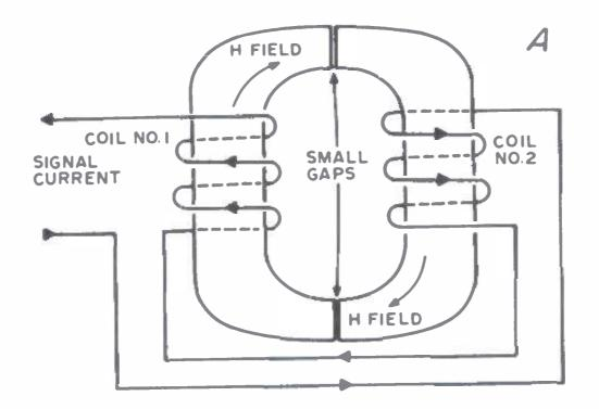
Figure 5: (a) Magnetic ring head, with balanced coils and gaps. (b) Magnetic head with single coil and gap.
