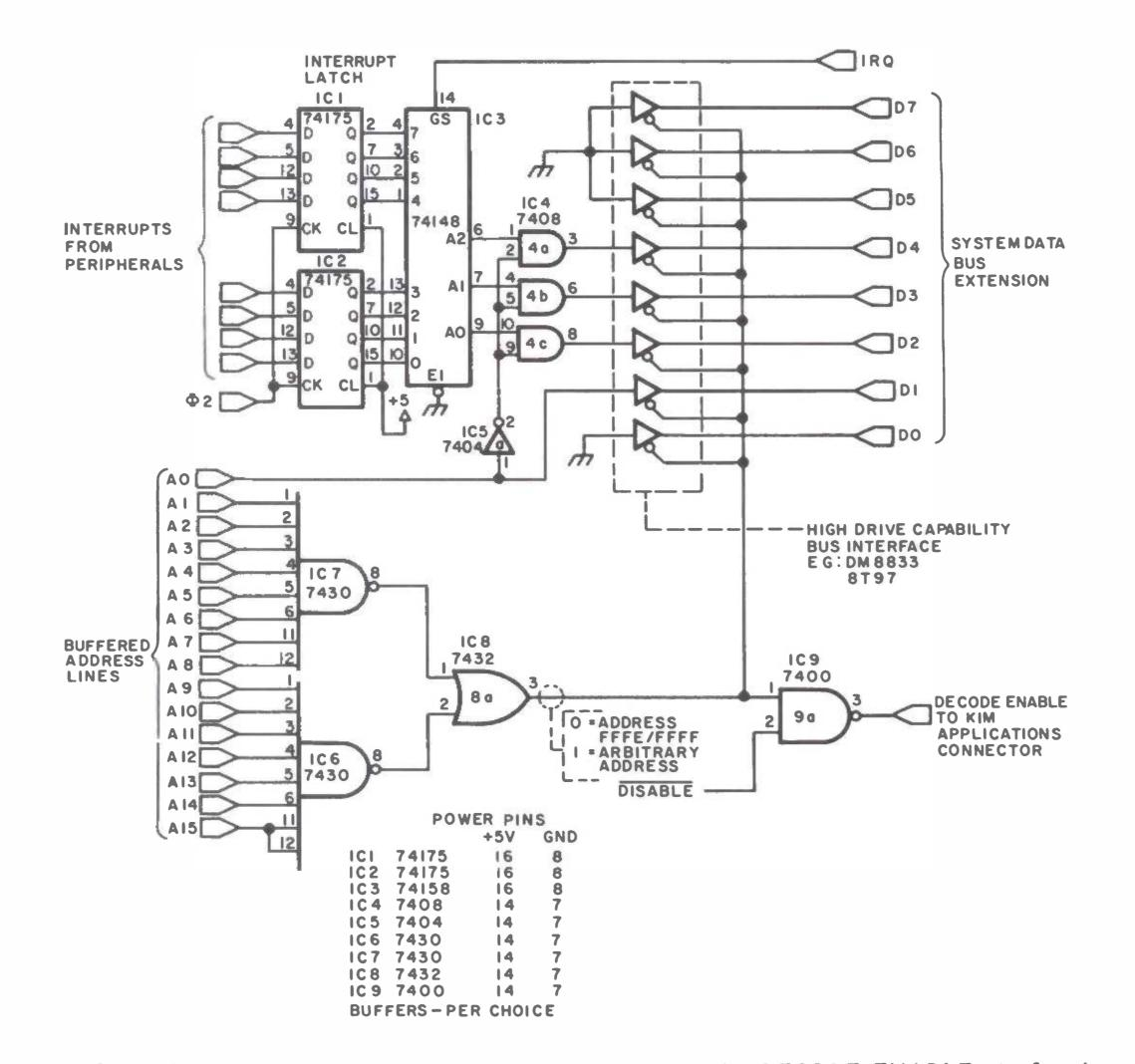
Figure 9: By disabling normal address decode through the DECODE ENABLE pin for the KIM-1 applications connector, an alternate source of the interrupt vector at locations FFFF
