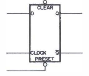
Fig. 12. Making a "D" flip flop out of a "JK" with an inverter. (Top view) Fig. 13. The block diagram of a D flip flop.
