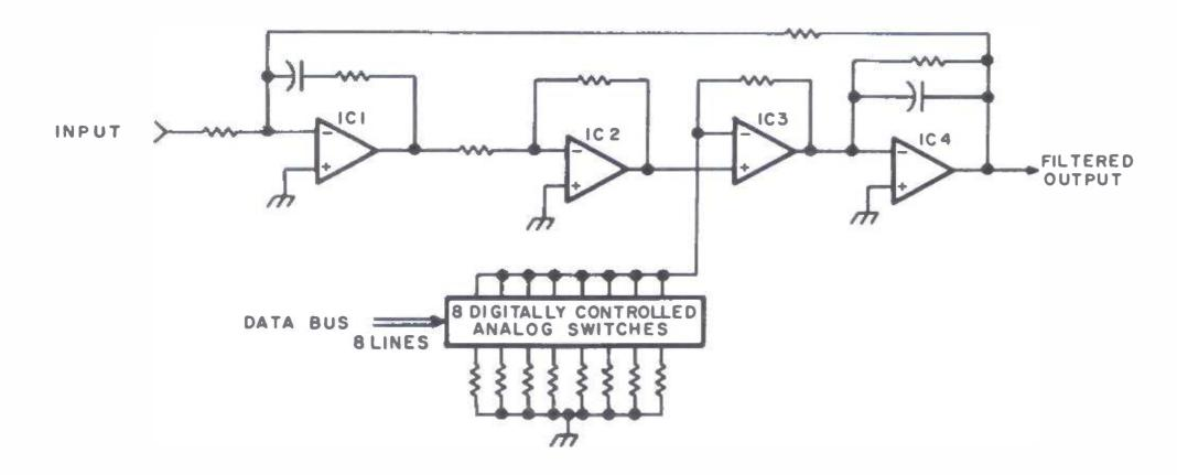
Figure 9: Typical Formant Resonator Circuit. A digitally controlled band pass filter can be built four operational from amplifiers and 8 digitally controlled analog switches. The filter characteristics are set by the choice of the resistance and capacitance elements as well as the digital control word. The operational amplifier IC3 serves as a gain controlled amplifier in the feedback loop, which alters the filter resonance.
