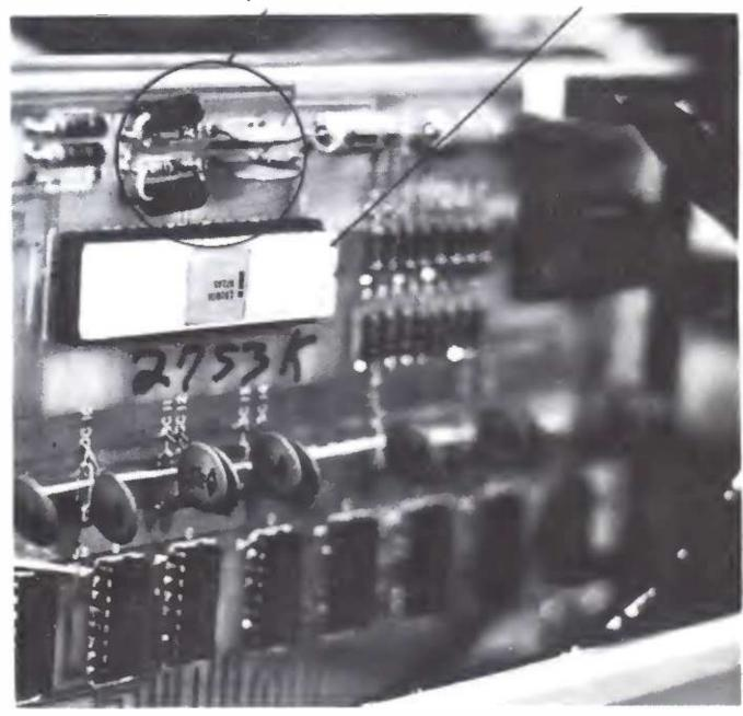
Fig. 3. Adding a parallel capacitance of .0047 uF to C8 of the Altair CPU board schematic lengthens the data out enable line time so that memory write does not extend longer than the data out time.
