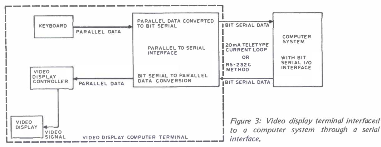
computer system via the telephone. The serial interface converts the parallel data from the keyboard to a bit serial form. In this form, the bits of the character are sent one bit at a time until the entire character has been sent. Of course the computer system must also have a serial IO interface.
