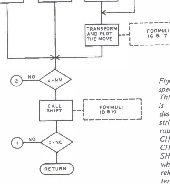
Figure 6: CHARPLOT specified as a flow chart. This is a subroutine which is called whenever it is desired to draw a character string of output. Subroutines referenced by CHARPLOT are: SUB-CHAIN (see figure 7) and SHIFT. SHIFT is a routine which is used to move the relative origin of characters from the present character position to the next character position.
