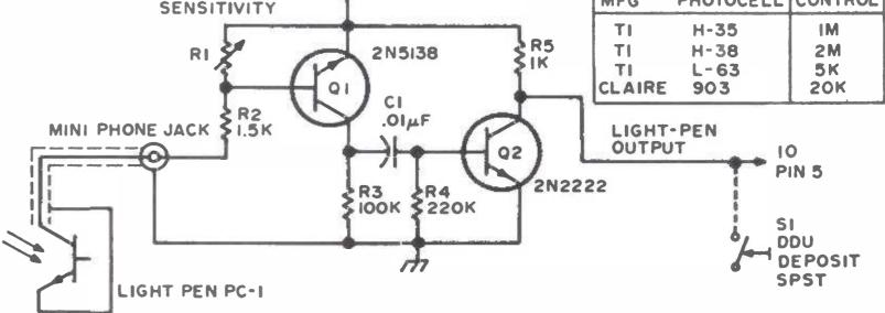
Figure 1: The simple version of the light pen can be constructed according to this schematic. All resistors ¼ W.
