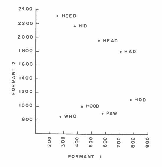
Figure 11: The Steady State English Vowels. The distinctions between various vowel sounds can be illustrated by plotting them on a two dimensional graph. The horizontal axis is the formant 1 frequency, the vertical axis is the formant 2 frequency. A location for each vowel utterance can be determined experimentally by locating the resonance peaks with an audio spectrum analyzer.
