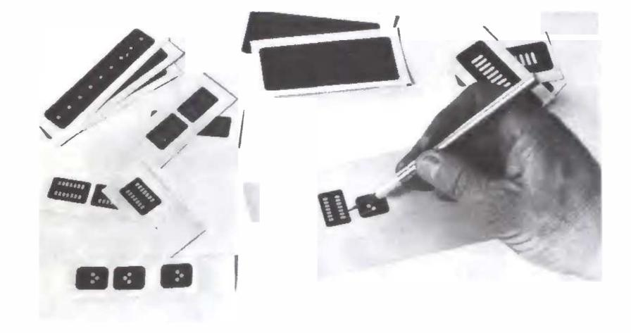
Photo 5: The Bishop Graphics "'B' Neg" Method. In this method, a negative is made directly, using self adhesive black patterns on a mylar backing. The connections between patterns are made by cutting away the black layer with a sharp knife as in the "Cut-N-Peel" method. using a yellow light for illumination.
