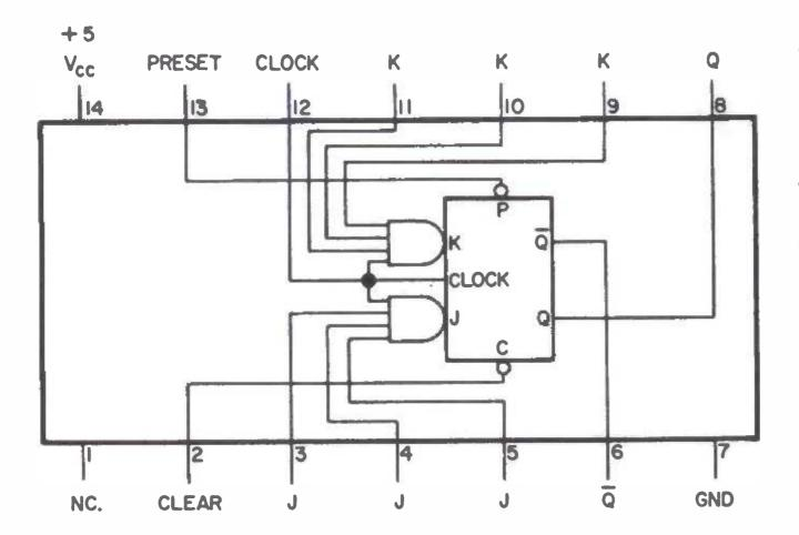
Fig. 7. Pinout of the 7472 IC, a positive clock pulse master/slave flip flop. (Top view )
