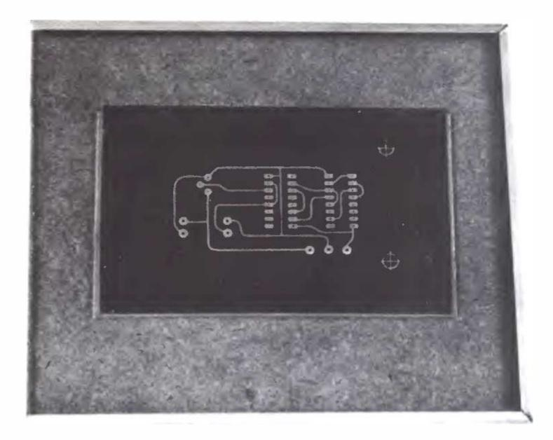
Photo 2: Printing the Circuit. Once a negative of the artwork has been created, the next step is to print the circuit. The negative is placed over a sensitized PC board and held firmly in place by a glass cover plate in the printing frame. The glass guarantees smooth and even contact for accurate transfer of the image. The board is then exposed to a photoflood lamp for one to three minutes.
