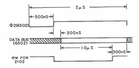
Figure 6: Write Cycle for Slow 2102 Memories using the circuit of figure 5. The output pulse width of RW is adjusted to 1.2  $\mu$ s nominally. (Check the results on your scope even if you use other than precision parts of the values shown for R1 and C1 in figure 5.)
