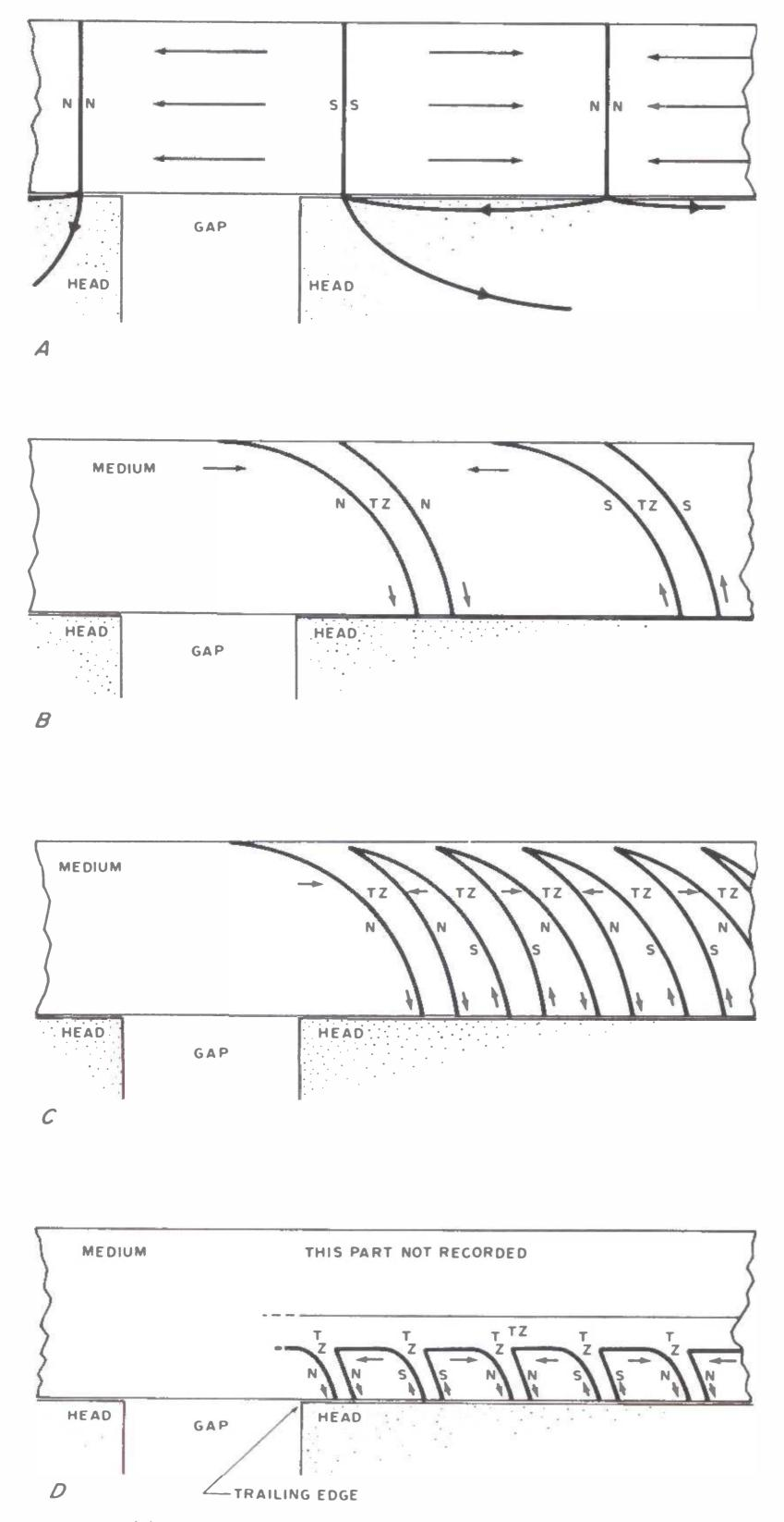
upon it, while the part farthest away from the head has not seen a field high enough to leave a signal. We can record through the whole coating by increasing the drive through the head coils. With a higher drive current, the transition region is labeled "Recording Zone – Maximum Drive" (figure 6). Note how the width of the transition region has increased; this is a fundamental limitation of the medium and the head.
