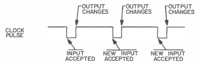
Fig. 5. Timing of a negative clock pulse master/slave flip flop.
