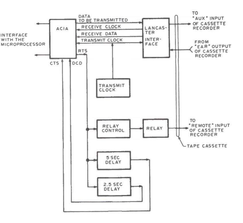
Figure 1: Block diagram of the COMPLEAT Tape Cassette Interface. This illustrates the major elements of the interface; see Don Lancaster's BIT BOFFER article in this issue for details of the hardware of the cassette modem.
