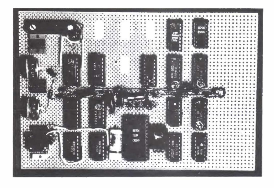
Photo 2: Prototype Circuit. The large socket is for the character generator. Test points are the 6 small rectangular objects along the left hand side of the board. A 7812 regulator in a plastic package is to the right of the character generator, and is used to provide the -12 V bias for the ROM. A zener diode with a dropping resistor is used to create the -5 V bias required for the ROM.
