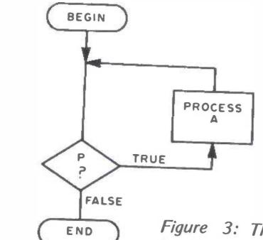
Figure 3: The DOWHILE structure is a looping form which repeats a specified SE-QUENCE structure over and over again as long as a condition, P, is true. DOWHILE tests the condition prior to executing the SEQUENCE structure for the first time. Thus in this example, the SEQUENCE structure A could be executed 0, 1, 2...N times, depending upon how soon the condition P becomes false as a result of A's work.
