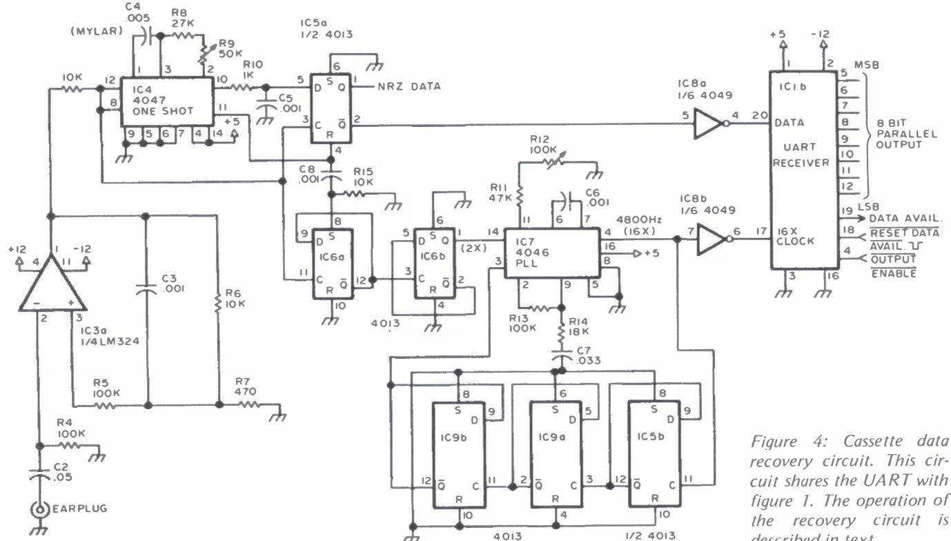
Instead of clocking the data into a shift register, it may be more desirable to use the receiver portion of a UART, since the UART receiver has built in circuitry to identify the beginning and end of each byte or character automatically. Furthermore, the UART parallel data outputs are 3-state, which permits convenient direct connection to most 10 ports or data buses. (For a more
