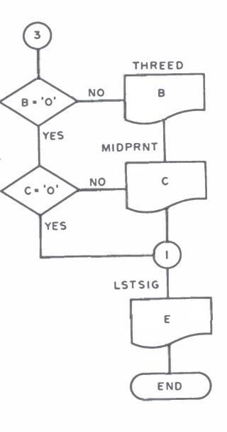
Figure 7: A binary to decimal conversion is performed to output 3 decimal digits encoded as ASCII numeric characters. This is a flow chart of the conversion routine, with labels referring to table 3.
