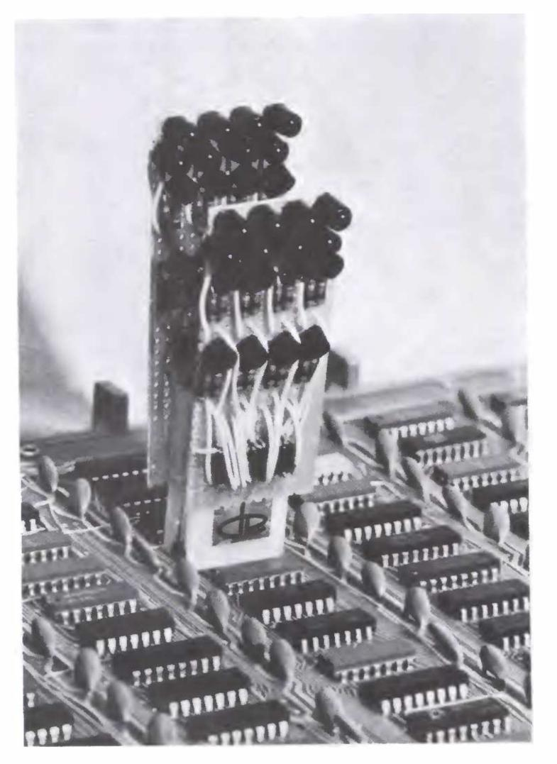
This test clip operates like the expensive, commercially available clips selling for \$85 or more without requiring batteries or external power. All types of ICs may be tested (TTL, DTL, MOS, etc.) and LEDs are used to indicate the logic state of each pin being tested.
