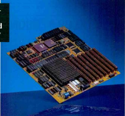
Solid. The 80486-33 EISA features 8 expansion slots with 6 EISA bus master slots, all of which allow for seamless integration of 16-bit and 8-bit AT/ISA I/O cards. Additionally, you'll have no more worries when your memory needs intensify. The 80486-33 EISA provides over ten various memory capacity choices from 1 to 64MB on-board! These memory configurations utilize 256K, IMB or 4MB SIMM memory concurrently.
