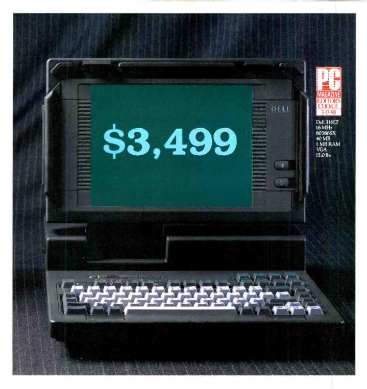
The laptop above is ours. The Dell 316LT. It comes with an Intel® 386" SX CPU running at 16 MHz. 1 MB of RAM, expandable to 8 MB, and a backlit VGA display. With a 40 MB hard drive it weighs 15 lbs. It won the InfoWorld Exceptional Value Award, and was one of only two 386SX laptops to win the PC Magazine Editor's Choice Award.
