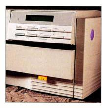
glance when the input tray is low on paper. The bright-orange flag, which is easily seen whether the printer is at your desk or connected remotely to a network, drops automatically. The printer need not be on for this feature to work.
