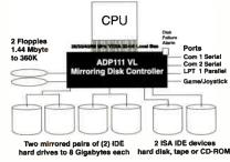
Sustained Transfer Rate (Core Test 2.7) 3624 Kb or 3.6 Mbytes per second in SVC 486 Meets IEEE VESA Standards
