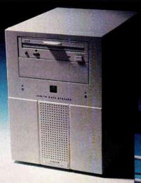
The 8- by 11- by 12inch 7-Stor Personal Server provides dedicated file and printer sharing for peer-to-pee Ethernet LANs. The optional internal CD-ROM adds \$499 to the \$999 base unit price of the Model 400. Hooking to coaxial cable requires an optional FriendlyNet connector (inset).
