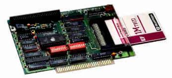
Quatech's I/O cards are available in RS-232. RS-422 and RS-485. Each are PCMCIA PC Card 2.1 compliant and support "hot-swapping" (insertion and removal of card while system is on). Quatech also offers a single port IBM PC compatible Enhanced Parallel Port PCMCIA card and a 24 digital input/output Type II PCMCIA card.
