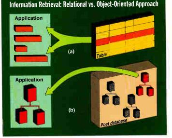
Retrieving information from a typical relational database (a) usually means pulling a row from a table structure, disassembling the fields, and translating them into variables your program can use. Poet (b) lets you pull objects from the database and place them directly into C++ class structures—all pointers and references intact.
