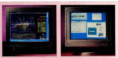
Nanao's FlexScan F780iW (left) and Nokia's Multigraph 445X define the leading edge in monitor technology, with 1600- by 1200-pixel resolution at an 80-Hz refresh rate. The FlexScan sacrifices low-end graphics support for excellent performance at high resolution, while the Multigraph 445X relies on digital fine-tuning to enhance display quality. Both monitors provide a wide variety of configuration options—the FlexScan through the front panel, and the Multigraph through a configuration menu.
