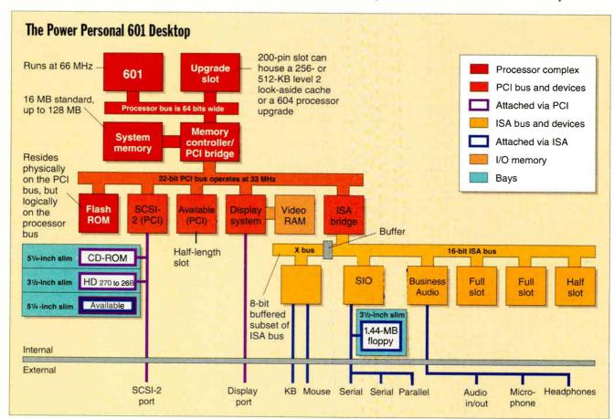
The basic system in the Power Personal desktop line runs a 601 processor at 66 MHz. The system employs the basic PReP topology of a hierarchy of buses connected by bridges. Most of the components used in the system are commodity components available on the open market.
