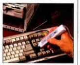
After you build this digital logic probe, you explore the operation of your computer's 101-key, detached "Intelligent" keyboard and its dedicated microprocessor.
