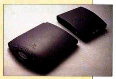
standard SCSI-2 connection. You can use the drive as either a stand-alone audio CD player or a multisession Photo CD player. The unit has data transfer rates of up to 306 KBps and an access speed of less than 180 ms.
