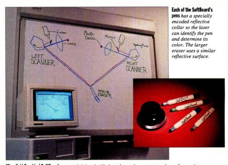
Microfield Graphics' SoftBoard, a porcelain/steel whateboard, uses lasers to scan the surface and report any pen activity to an attached computer. Included Windows or Macintosh software converts your drawings into viewable images.
