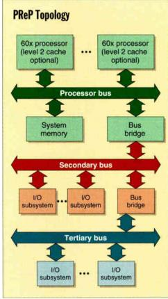
PReP systems can incorporate many different bus types into a hierarchical structure. At the top is the processor bus, which connects one or more processors and their caches to both system memory and system I/O. Connection to system I/O comes via a bus bridge to a secondary bus; in most PReF systems, this secondary bus will be PCI. The secondary bus can then bridge to a tertiary bus, such as ISA, and so on.
