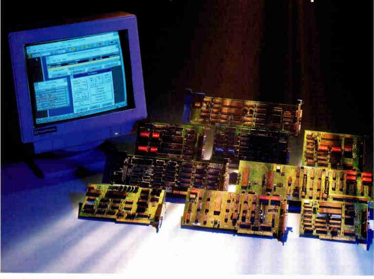
uatech manufactures a complete line of communication adapters for PC/XT/AT®, Micro Channel® and compatible buses to meet asynchronous and synchronous, serial and parallel communication requirements with protocols such as RS-232, RS-422, RS-485, Current Loop and IEEE488.
