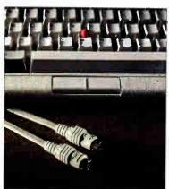
design: The integrated Trackpoint pointing device allows you to navigate graphical applications without taking your hands off the keyboard to use a mouse.
