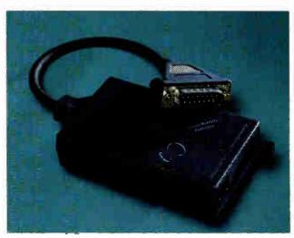
20 feet of silver-satin cable with RJ-11 constructions at a silver streak allows full 10-Mbps Ethernet speed over the UTP phone cord.
