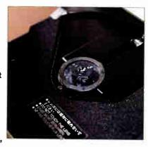
as do the Pentiums and 486s we received from DEC. This unique drive design uses three spring-backed ball bearings to hold a CD in place.
