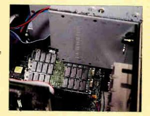
manufacturer doesn't follow the convention of designating the 3½-inch drive as the A drive. We couldn't reverse drive designations from within the BIOS setup since both drives are on the same ribbon cable connector, and the documentation did not provide any information on changing jumpers.
