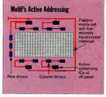
With active addressing, proprietary ASICs (applicationspecific ICs) that sit off the panel can address many rows simultaneously. The ASICs take the image from the graphics card and quickly calculate in real time where voltages need to be applied to the crystals. According to Motif, this technique provides near-TFT performance at a slightly higher cost than passive
