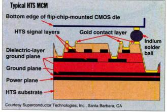
In HTS MCMs, line widths in transmission lines can be very narrow (i.e., 2 microns), allowing a higher packing density and improved signal transmission over conventional MCMs. Shown here is the module that wires multiple chips together while providing their ground plane and power source.
