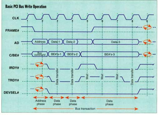
A PCI write transaction is similar to a read transaction. The data phase of read and write transactions ends when The PCI bus can transfer both IRDY# and TRDY# are asserted. The wait states shown here are inserted only when a slow device is accessed.
