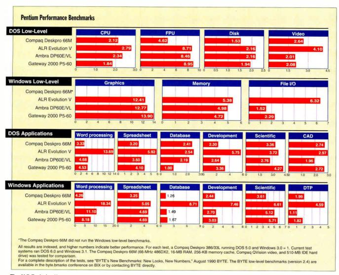
**The ALR Evolution V** provides the best overall applications performance, mainly because of its caching IDE drive card—something you could add to the other systems. However, its good low-level performance gives it an edge in processor-intensive tasks regardless of peripheral configuration. Note the strong floating-point performance of the Pentium systems relative to the 66-MHz 486 Compaq, included for comparison.
