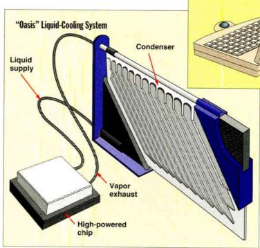
Aavid's liquid-cooling scheme uses Fluorinert, a material that has a boiling point of about 60'C. Once the Fluorinert reaches its boiling point, it forces open a valve that leads to the condenser. There, the vapor is cooled and returned to the evaporator unit.
