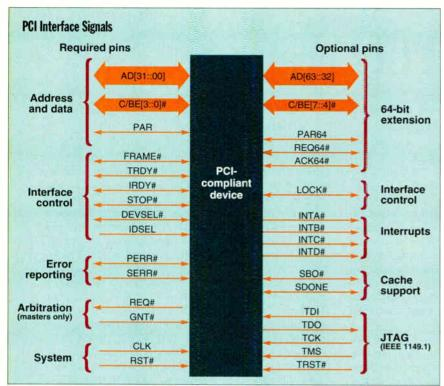
PCI pins and signals. The required pins are signals that are needed to implement a PCI bus. The optional pins help implement a 64-bit bus, exclusive memory access (the LOCK signal), and cache support.
