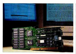
The Colorgraphic Twin Turbo gives not one, but two accelerated displays. Two VGA connections support two monitors: The Windows driver stretches the desktop across both monitors so that windows can be dragged seamlessly from one monitor to the next as if you had one big monitor.
