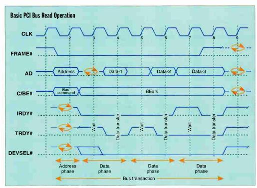
A read transaction starts with the address phase, with FRAME# asserted, AD[31::0] driving the address onto the bus, and C/BE# containing a valid PCI bus command. The data phase follows, which can have any number of data transfer and wait cycles. During the data phase, C/BE# indicates what byte lanes are used.
