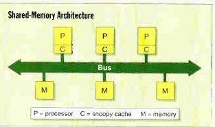
Caching is required for performance, but intelligent caches are needed to work correctly. Consider the following example: Processor A reads a memory location and caches the data; processor B writes a new value to that same location. "Snoopy" caches, which monitor the bus, keep A from using the outdated value.
