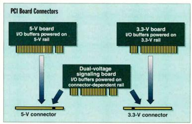
PCI won't replace the standard expansion buses that A keyed notch on the PCI board determines what signal levels it supports. This
