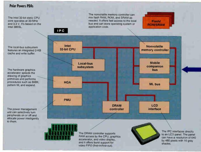
The Polar chip set is a highly integrated solution that offers just about all the functionality you need in a PDA system.
