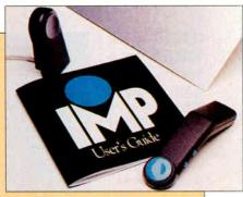
15 feet away from your computer. Windows- and Microsoft Mouse-compatible, Imp consists of a hand-held wireless transmitter and a compact receiver that connects to your PC's serial port. The transmitter has a control disc for cursor control and four auxiliary buttons that act as keyboard keys. Powered by your PC, the receiver has indicator lamps that reflect communication activity and the status of the batteries in the transmitter.
