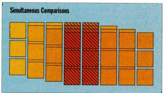
**The motion estimator hardware** lets the same 16- by 24-pixel range be used for phases 1, 2, 3, and 4 of four different 8- by 8-pixel blocks concurrently. This limits the number of times that a piece of an image must be loaded into the motion estimator.
