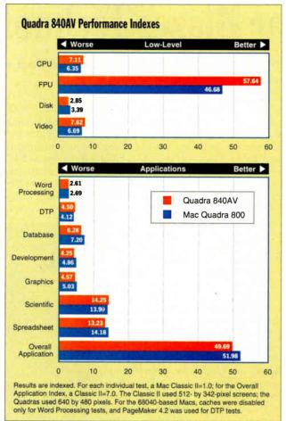
Running at 40 MHz, the Quadra 840AV is the fastest Mac yet. A new SCSI driver, however, puts hard drive performance slightly behind that of a Quadra 800 that BYTE tested previously. Slower drive performance spills over into some of the application test results.
