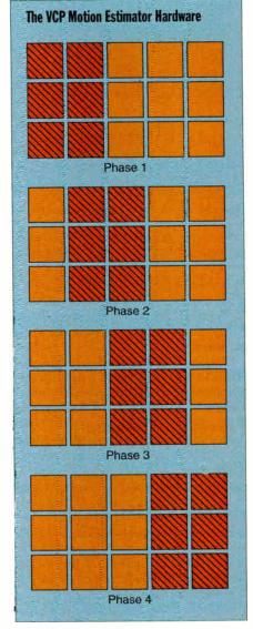
The VCP doesn't store the entire 40- by 24pixel block internally because such a large block would slow processing throughput: thus, the hardware compares the blocks in four phases.
