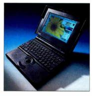
provides rich color, good contrast, and a wide viewing angle. The PowerBook 165c's power charger cranks out 24 W (up from 15 W) and can recharge the battery faster. In addition, the PowerBook 165c is less expensive than PC notebooks with active-matrix screens.
