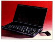
Other features, such as the mechanical-arm-like mouse that pops out from the side of the machine, Windows 3.1 in ROM, and the complete lack of traditional (and power-consuming) rotating hard drives, put this machine a notch above the competition.
