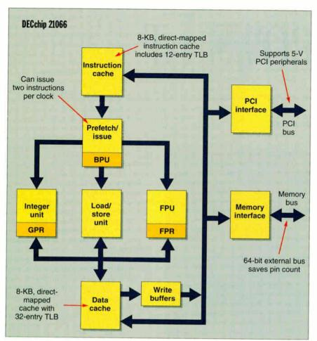
**Integrating an Alpha core** with both memory and PCI controllers yields a powerful chip that is easy and inexpensive to integrate into a system. Despite its added functionality, the DECchip 21066 requires 144 fewer pins than the 21064.
