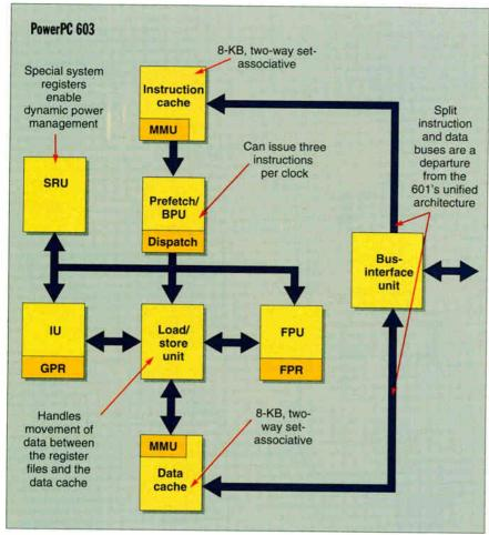
**The PowerPC 603** introduces a Harvard architecture and dynamic power management to the PowerPC line. Expected to dissipate 2 to 3 W at 80 MHz, it is ideal for notebooks and energy-efficient desktop systems.
