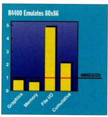
Running the BYTE low-level Windows benchmarks, an SGI Magnum 75SC (Mips R4400 processor) turns in a credible performance in emulation mode against an IBM PS/2 Model 90 XP 486 (486DX/33 processor). The cumulative index is skewed by the fantastic performance of the Windows NT file system.
