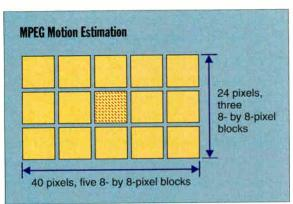
**The MPEG algorithm** searches a 40- by 24-pixel block surrounding a single 8- by 8-pixel block to find the best alignment between the reference frame and the current one.
