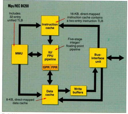
The R4200 integrates a complete RISC pipeline and 24-KB cache on a die 82 mm². Its low power consumption and high performance make it ideal for notebook systems.
